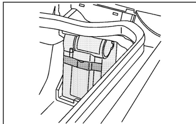
3. Locate the tire inflator kit on the driver's side of the vehicle, near the back corner of the trunk.
