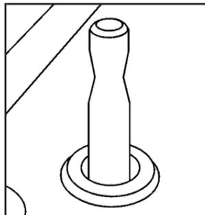
From inside the vehicle, use the manual door lock knob. Pull up on the knob to unlock the door. Push down on the knob to lock the door.
