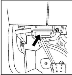
1. Locate the interior hood release lever. It is located below the instrument panel on the driver's side of the vehicle.
