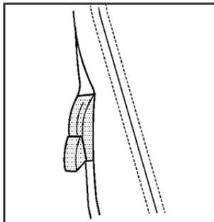
Your vehicle may have a latch located on the outboard side of the seats near the top of the seatback that enables the front seatback(s) to fold forward.
