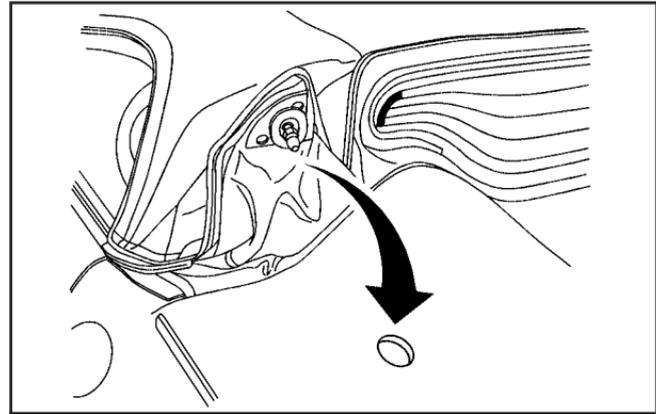
7. At the rear edge of the convertible top, press down on the two buttresses (C) to latch them into the top of the trunk.
