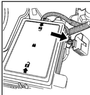
The remote positive (+) terminal is located under a red plastic cover on the engine compartment fuse block. Open the cover to access the terminal.
