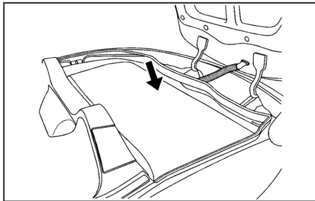
8. After the top is stored, apply one even push, as shown, on the convertible top to ensure that the top is fully retracted and securely stored.
