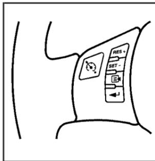
The cruise control buttons are located on the steering wheel.
