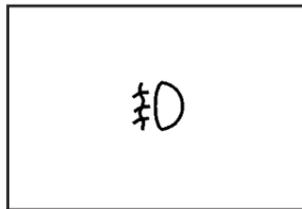
If your vehicle is equipped with a fog lamp button, it is located on the instrument panel, to the right of the steering wheel.
