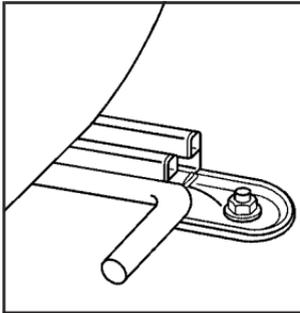
Lift the lever located under the front of the seat to unlock it.
