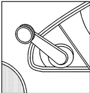
If your vehicle has manual windows, use the window crank to open and close each window.
