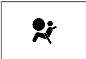
There is an airbag readiness light on the instrument panel cluster, which shows the airbag symbol.
