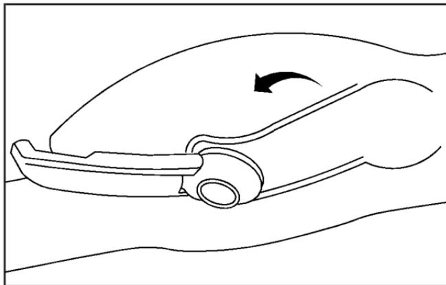
5. The convertible top front latch, located above the inside rearview mirror, must be unlatched. Pull the latch down and turn it counterclockwise to unlatch it. Leave the latch open and rotated to prevent damage.
