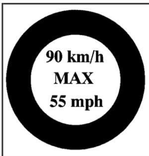
16. If the flat tire was able to inflate to the recommended inflation pressure, remove the maximum speed label from the sealant canister and place in a highly visible location such as the inside of the upper left corner of the windshield or to the face of the radio/clock.
