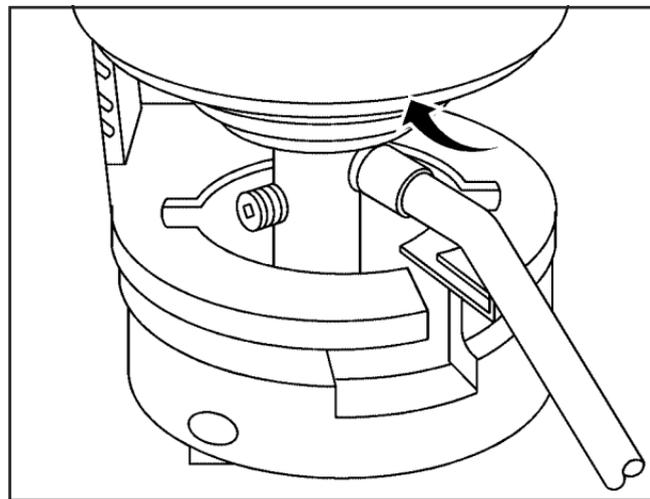
1. Unlock the air compressor inflator hose from the sealant canister by pulling the lever up.
