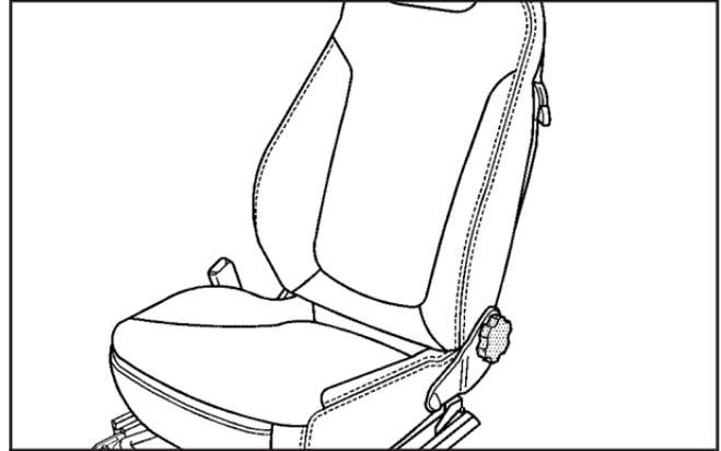
To adjust the seatback, turn the knob on the outboard side of the seatback until the seatback is in the desired position.
