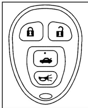
The vehicle's doors can be locked and unlocked, and the trunk can be unlatched from about 3 feet (1 m) up to 60 feet (18 m) away with the remote keyless entry transmitter.
