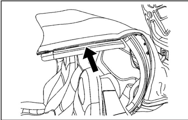
5. Pull the convertible top forward by firmly gripping the side edge (B) and applying a brisk upward and forward motion to get the top in the pull-up position.
