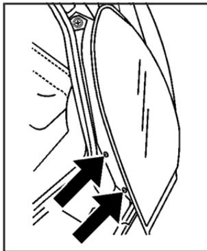
2. Remove the two screws, which hold the taillamp assembly, from inside the vehicle.
