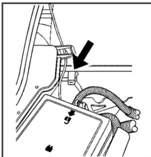
The remote negative (-) ground bracket is located in the rear of the engine compartment, on the passenger's side of the vehicle, and is marked GND (-).
