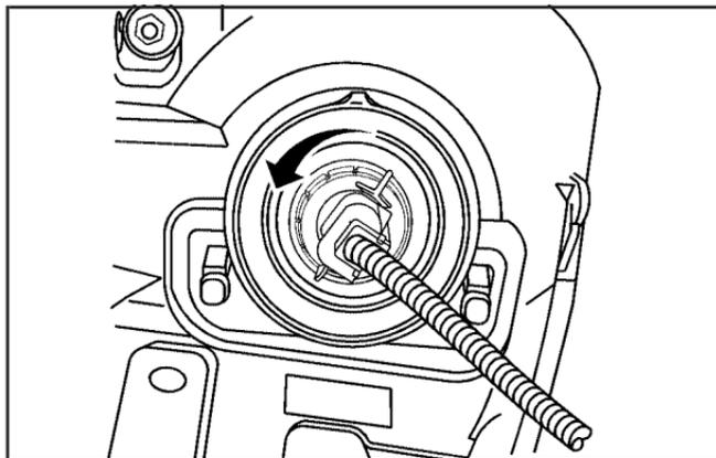
3. Turn the bulb socket counterclockwise and pull it from the headlamp assembly.
