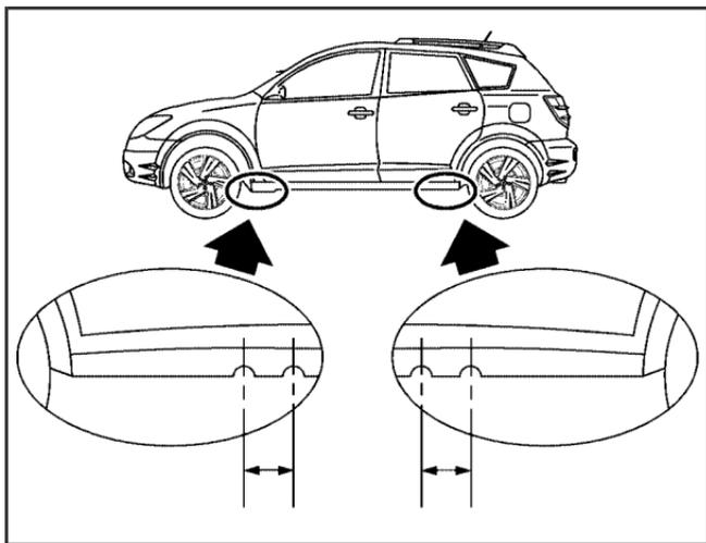
4. Position the jack and raise the jack lift head to fit over the car flange between the two notches.
