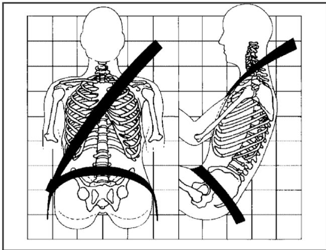
The lap part of the belt should be worn low and snug on the hips, just touching the thighs. In a crash, this applies force to the pelvic bones. And you would be less likely to slide under the lap belt. If you slid under it, the belt would apply force at your abdomen. This could cause serious or even fatal injuries. The shoulder belt should go over the shoulder and across the chest. These parts of the body are best able to take belt restraining forces.
