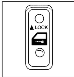
If your vehicle has this feature, the power door lock switch is located on the armrest of the driver's and front passenger's door.
