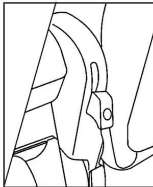
2. Pull up on one of the levers located on either side of the back of the passenger's seatback.
