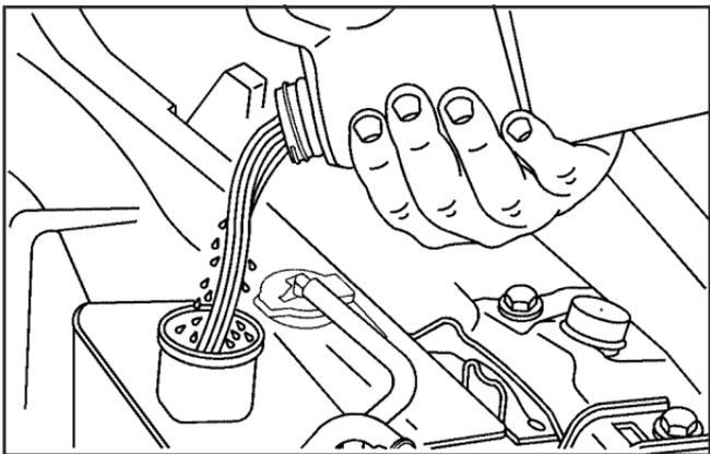
4. Then fill the coolant recovery tank to the FULL mark.
