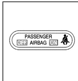
The passenger sensing system will turn off the right front passenger's frontal airbag and seat-mounted side impact airbag (if equipped) under certain conditions.
