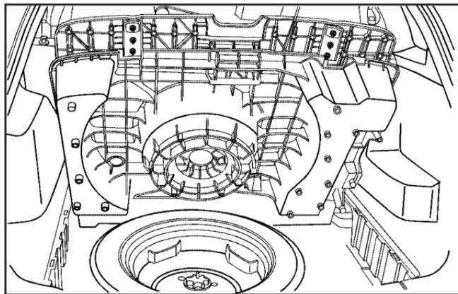
4. Unscrew the center retaining nut and lift up the plastic tray to expose the compact spare tire.
