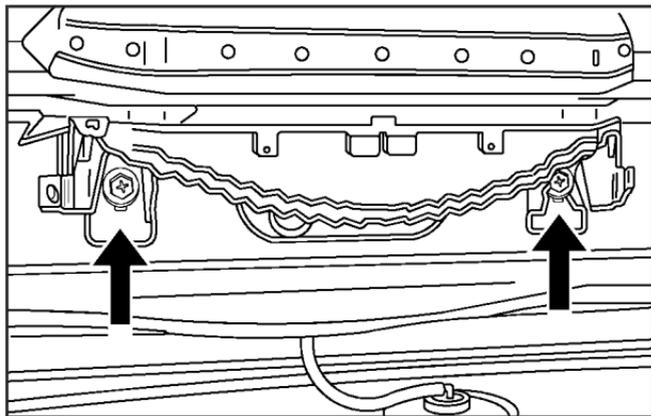
3. Remove the two screws from the CHMSL housing. Then remove the housing to expose the bulb.
