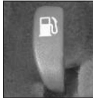
The fuel door release lever is located near the floor under the driver's seat on the outboard side.
