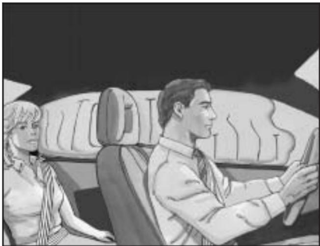
If your vehicle has a roof-mounted side impact airbag for the driver and the passenger seated directly behind the driver, it is in the ceiling above the side windows.
