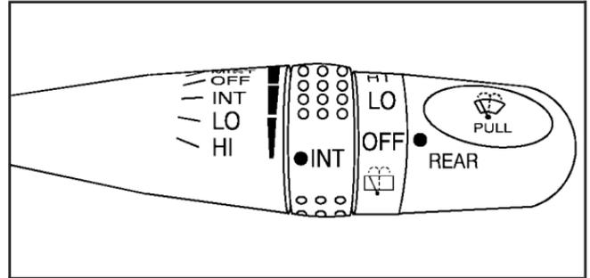
The lever on the right side of the steering column controls the windshield wipers and washer.
