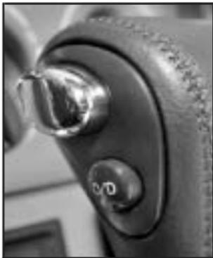
Your automatic transaxle has an O/D (overdrive off) button located on the left side of the shift lever.
