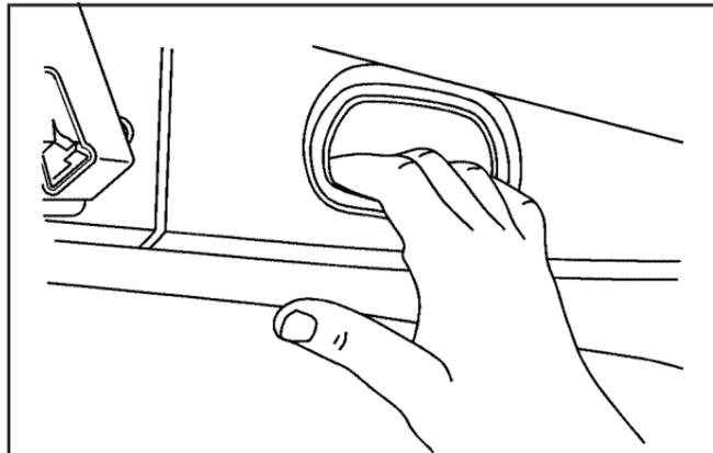
When closing the liftgate, use the handle to pull it down.
