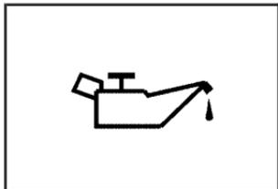
If the engine oil pressure light appears on the instrument cluster, it means you need to check your engine oil level right away.
