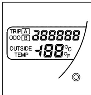
The button located on the right side of the instrument panel cluster allows you to switch between the odometer and the two trip odometers.
