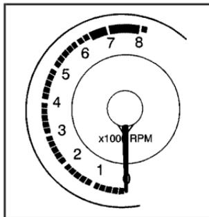
The tachometer shows engine speed in thousands of revolutions per minute (rpm).
