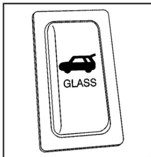
Your vehicle may have a liftglass release button which is located on the instrument panel to the left of the steering wheel. Press this button to release the liftglass.
