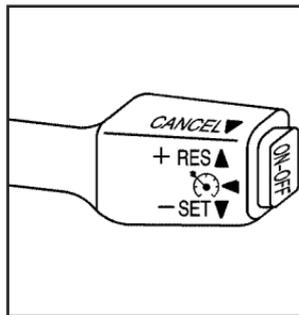
If your vehicle has cruise control, the lever is located on the right side of the steering wheel.
