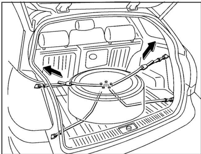
7. Position the tire edge against the rear center end of the floor panel. Pull the end of the straps to make sure the tire is secure.
