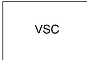
This light warns that there is a problem somewhere in the traction control system or the vehicle stability control (VSC) system.
