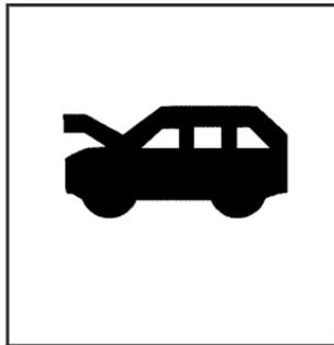
1. Pull the release handle with this symbol on it. It is located below the instrument panel to the left of the steering wheel.
