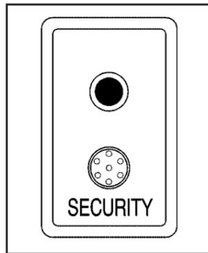
The indicator light located on the instrument panel to the left of the steering wheel will come on when all doors and liftgate are closed and locked.
