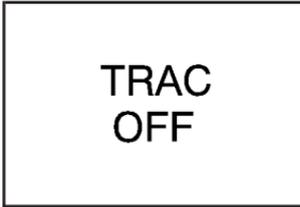
The TRAC OFF button is located to the left of the steering wheel below the instrument panel cluster.
