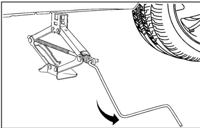
11. Lower the vehicle by turning the jack handle counterclockwise. Lower the jack completely.
