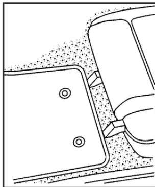
To remove the floor mat, pull up on the rear of the mat to disconnect it from the locator hooks.
