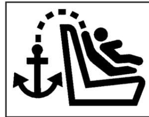
To assist you in locating the top tether anchors, the top tether anchor symbol is located on the trim cover.
