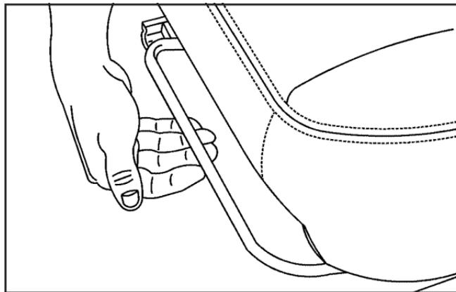
Lift the bar located under the front of the seat to unlock it. Slide the seat to where you want it and release the bar. Try to move the seat with your body to be sure the seat is locked in place.
