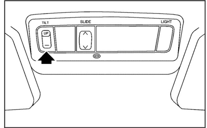
If the vehicle has a sunroof, it can be opened or put in a tilt position. To tilt the sunroof, slide the sunshade rearward, then press the switch marked UP. Press the other end of the switch to lower the sunroof. The ignition must be in the ON position for the switch to work.
