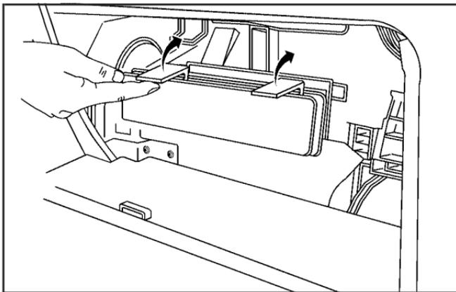
3. Lift the snaps on the filter cover to remove the cover.
