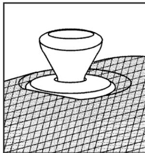
1. Pull up on the lock release knob, located on the top outboard side of the seatbacks.
