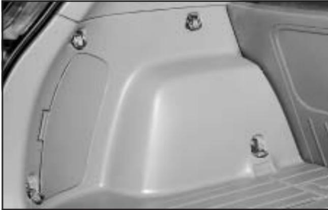
The tire tie-down straps are designed to secure a flat tire. You can also use the straps and hooks to secure your luggage.
