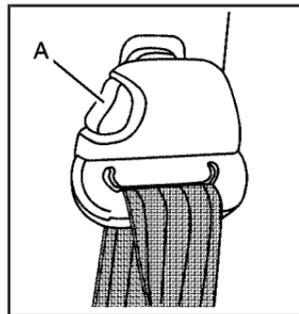
To move it down, squeeze the button (A) and move the height adjuster to the desired position. You can move the height adjuster up just by pushing up on the shoulder belt guide.
