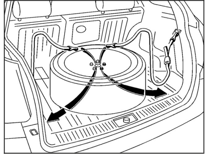
5. Pass the straps through the center hole of the wheel.
