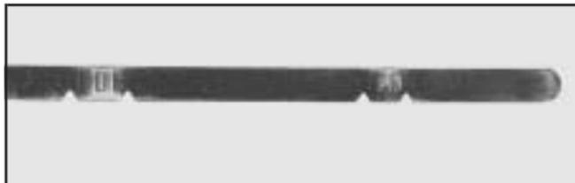
3. Check both sides of the dipstick, and read the lower level. The fluid level must be between the two dimples in the hot range.
