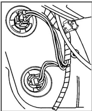
2. Turn the bulb socket counterclockwise and pull it out of the lamp housing.
