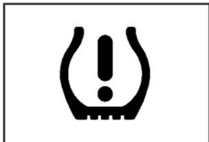
This light, on the instrument panel cluster, comes on when the tire pressure monitoring system detects a low-tire condition.
