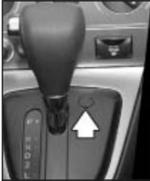
2. Carefully pry the cover from the shift lock override, located to the right of the shift lever.
