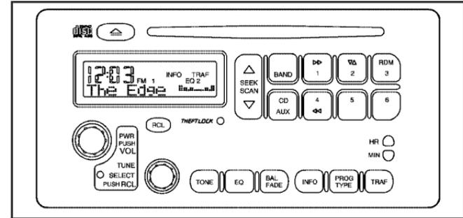
The radio has a blinking red light that is used as a theft-deterrent feature. The light will blink whenever the ignition is off.
