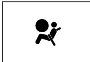
This light will come on for about seven seconds when you start your vehicle. Then the light should go out. This means the system is ready.
