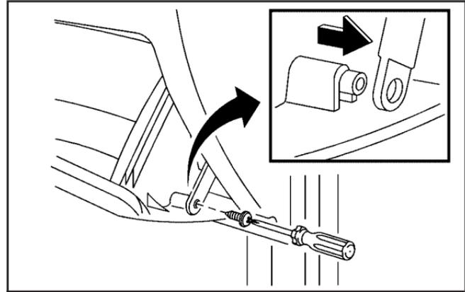
1. Lower the glove box door and remove the screw on the right side of the glovebox with a tool. Slide the arm of the glovebox off.
