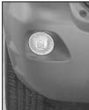
The back-up lamp bulb is located in the bumper.
