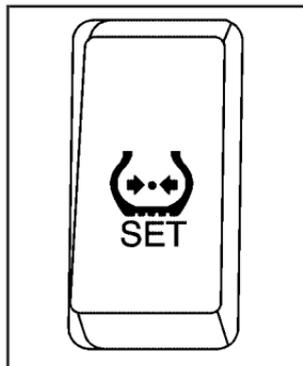
3. If the low-tire pressure warning light is on, push the SET (reset) button for a few seconds. The low-tire warning light should go off. The reset button is on the instrument panel to the left of the steering wheel.
