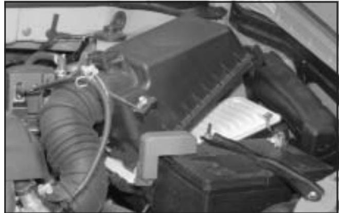
1. Release the two clips that hold the cover down.
