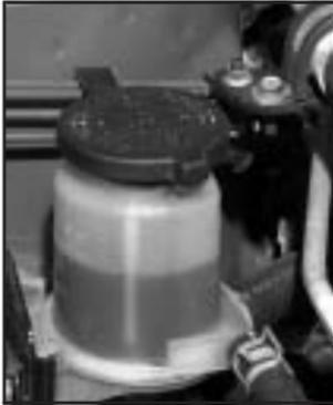
The power steering fluid reservoir is located in the engine compartment on the passenger's side of the vehicle. See *Engine Compartment Overview* on page 5-12 for reservoir location.
