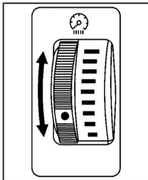
The instrument panel brightness control is located to the left of the steering wheel on the instrument panel. Turn the wheel on the left of the control up or down to increase or decrease brightness.
