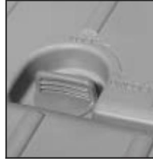
1. Turn the two lock knobs on the floor of the cargo area to UNLOCK.
