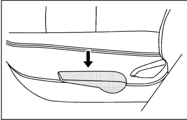
The driver seat height adjuster is located on the outboard side of the seat. To raise the seat, pull up on the lever repeatedly until the seat is at the desired height. To lower the seat, push down on the lever repeatedly until the seat is at the desired height.
