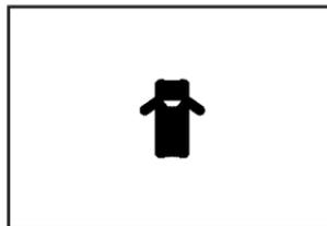
This light will come on if any door, the rear liftgate or the rear liftglass are not completely closed.
