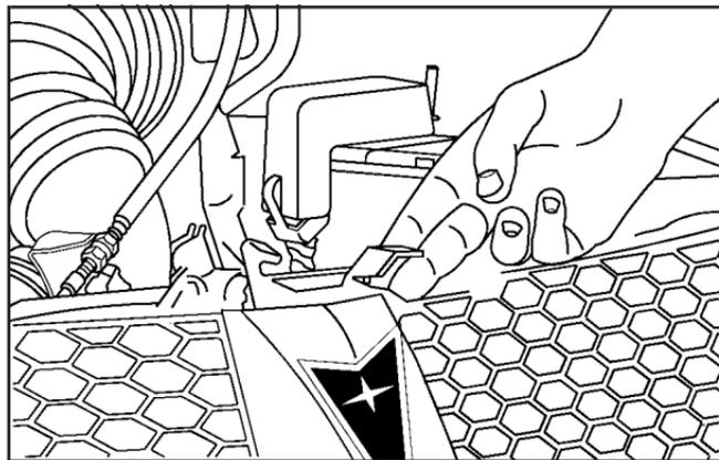
2. Then go to the front of the vehicle and pull up on the secondary hood release. The lever is located near the middle of the hood.
