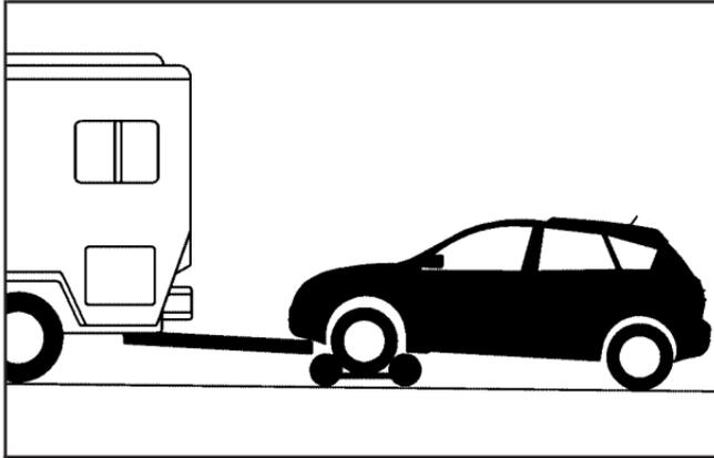
If your vehicle is a front-wheel drive vehicle it can be towed using a dolly. To tow your vehicle using a dolly, follow these steps:
