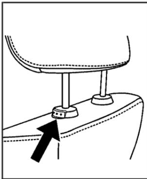
Press the release button at the base of the head restraint and push the restraint down to lower it.
