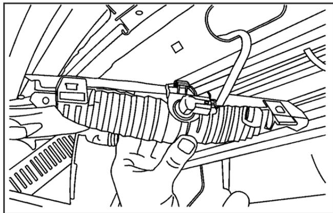
4. Turn the bulb socket counterclockwise and pull it out of the lamp housing.
