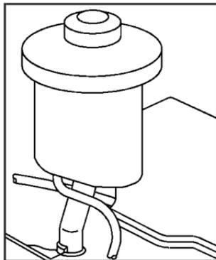
The hydraulic clutch and brake master cylinder use the same reservoir. It is filled with DOT-3 brake fluid. See *Engine Compartment Overview* on page 5-12 for the location of the reservoir.
