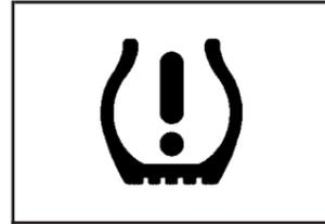
This light should come on briefly as you start the engine. It will then come on only when a low tire pressure condition exists.
