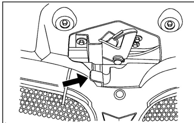
2. Then go to the front of the vehicle and move the secondary hood release lever to the right.
