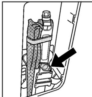
3. Install the jack in the left side panel of cargo area and secure it with the wing bolt.
