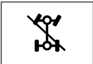
This light will come on along with the ALL WHEEL DRIVE OFF message when the rear drive system is overheating.
