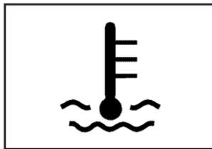
The engine coolant temperature warning light will come on when the engine has overheated.
