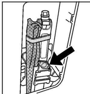
5. Remove the wing-bolt holding the jack and then remove it.
