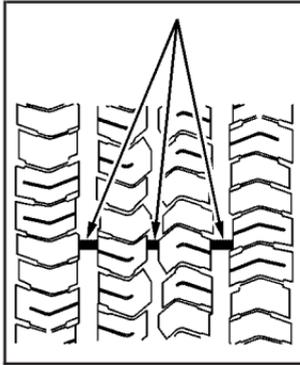
One way to tell when it is time for new tires is to check the treadwear indicators, which will appear when your tires have only 1/16 inch (1.6 mm) or less of tread remaining. Some commercial truck tires may not have treadwear indicators.
