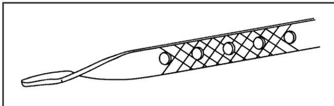
If the oil is below the cross-hatched area at the tip of the dipstick, you will need to add at least one quart/liter of oil. But you must use the right kind. This section explains what kind of oil to use. For engine oil crankcase capacity, see *Capacities and Specifications on page 436*.
