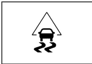
Your vehicle has a Traction Control System (TCS) and StabiliTrak<sup>®</sup> warning light.
