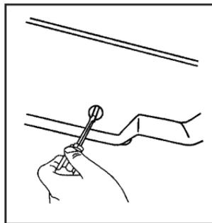
Use a tool to push the service release lever located on the latch until you hear or feel the gate release.
