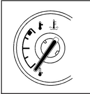
This gage measures the temperature of the vehicle's engine.
