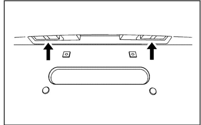
2. Turn and pull the license plate lamp down through the liftgate opening.
