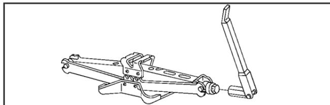
4. Attach the wheel wrench to the jack bolt head and turn the wheel wrench clockwise. That will raise the lift head a little.
