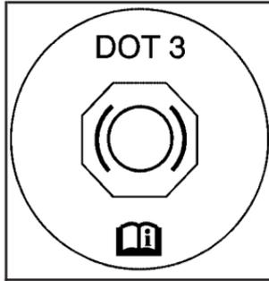
Your brake master cylinder reservoir is filled with DOT-3 brake fluid. See *Engine Compartment Overview on page 348* for the location of the reservoir.
