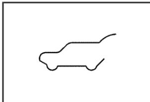
If this light comes on, your liftgate is not completely closed. Driving with the liftgate open can cause carbon monoxide (CO) to enter the vehicle.
