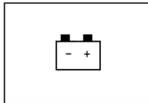
The battery warning light will come on briefly as a check, when you turn on the ignition. Then it should go out when the engine is started.
