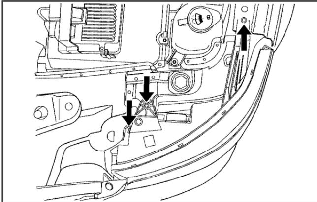
2. Remove the three headlamp assembly attachment screws.
