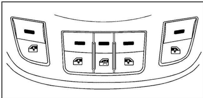
The window switches for all doors are located on the center console. A window switch for each rear window is located on each rear door.
