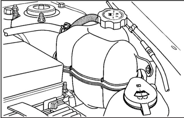
The surge tank is located on the driver's side of the engine compartment. See *Engine Compartment Overview on page 348* for more information on location.
