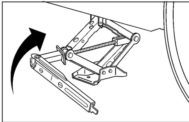
8. Raise the vehicle by turning the jack handle clockwise. Raise the vehicle far enough off the ground so there is enough room for the road tire to clear the ground.
