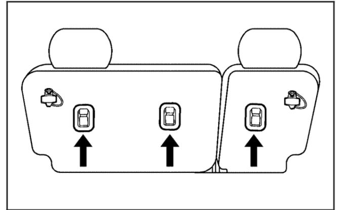
The top tether anchors for each rear seating position are located on the back of the rear seatback. You may need to adjust the rear compartment storage panel/cover in the rear cargo area to access the anchors. Be sure to use an anchor located on the same side of the vehicle as the seating position where the child restraint will be placed.
