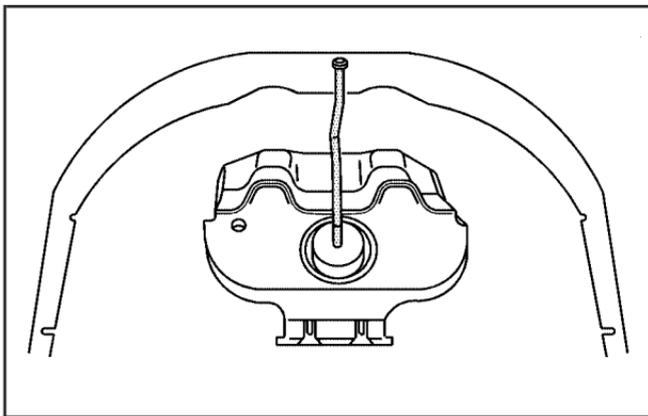
5. Screw the threaded wheel stow rod onto the spare tire bracket. The final position of the wheel stow rod must be turned to the farthest forward position.
