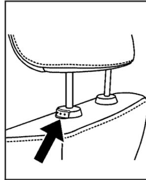
Pull the head restraint up to raise it. To lower the head restraint, press the button, located on the top of the seatback, and push the restraint down.
