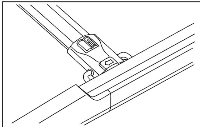
Press the levers down until the locking mechanisms fully engage to the side rail. Make sure each lever is in the down position. The crossrail will not slide when properly engaged.
