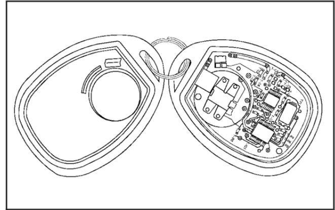
2. Once the transmitter is separated, use a pencil or similar object to remove the old battery. Do not use a metal object.
