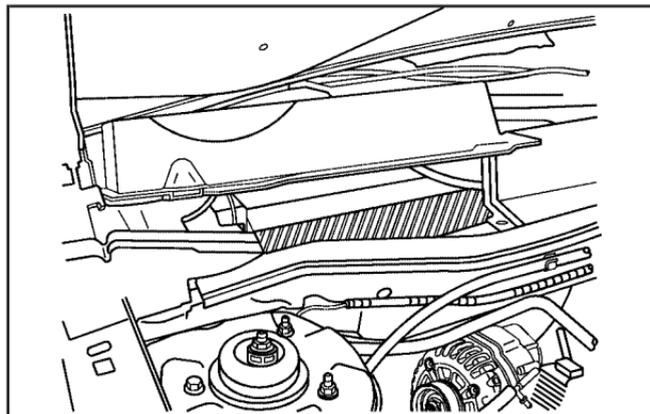
6. Remove the filter from the vehicle.
