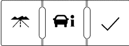
The buttons are the trip/fuel, vehicle information, and set/reset buttons. The button functions are detailed in the following pages.
