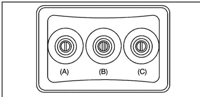
The A/V jacks are located on the rear of the floor console. The A/V jacks allow audio or video signals to be connected from an auxiliary device such as a camcorder or a video game unit to the RSE system. Adapter connectors or cables may be required to connect the auxiliary device to the A/V jacks. Refer to the manufacturer's instructions for proper usage.
