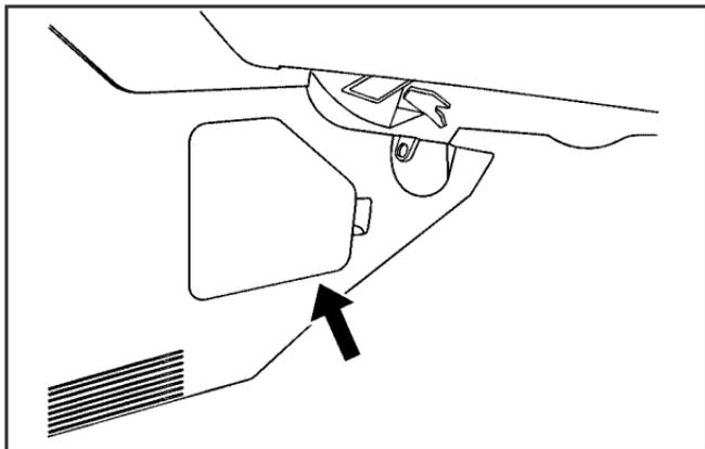
Remove the console cover to access the fuse block.
