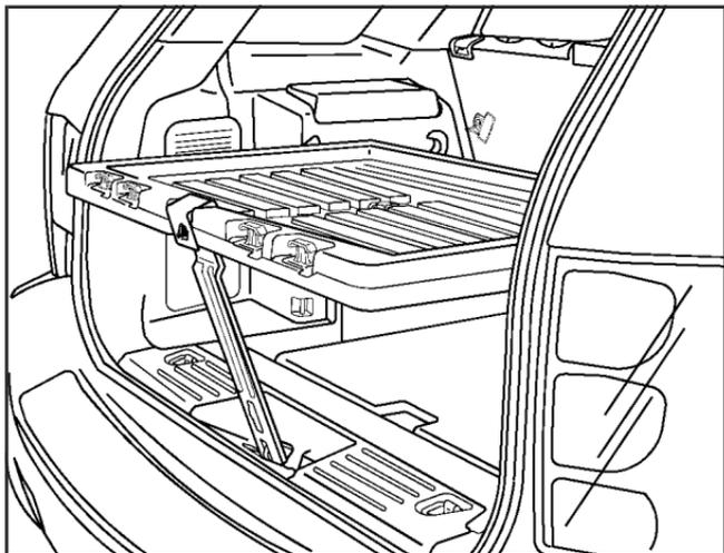
Your vehicle may have an adjustable panel that also functions as a table. The maximum load for the table is 100 lbs. distributed (45 kg).
