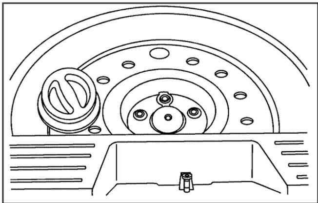
2. Remove the nut retaining the spare tire.
