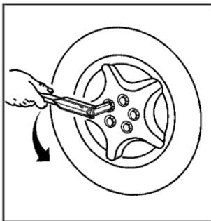
1. Loosen all five plastic caps by turning the wheel wrench counterclockwise. Do not try to remove plastic caps from the cover or center cap.
