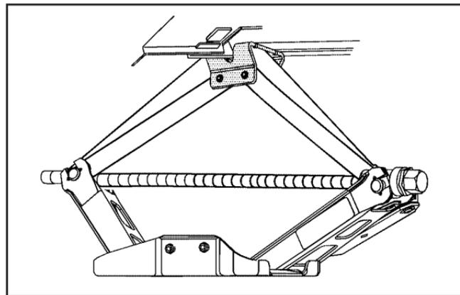
With the jack head positioned correctly on the metal jacking flange, it should look like this from underneath.
