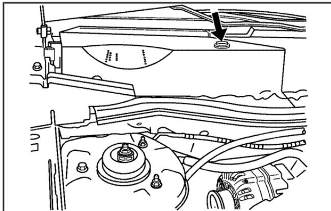
1. Remove the push pins from the rear of the passenger's side air inlet panel. It is located in the rear of the engine compartment on the passenger side of the vehicle.
