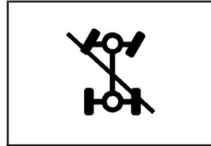
This light will come on when the rear drive system is overheating.
