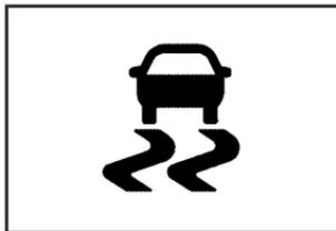
The traction control system can be turned off by pressing the traction control button, located next to the gear shift lever.
