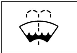
Open the cap with the washer symbol on it. Add washer fluid until the tank is full. See *Engine Compartment Overview* on page 348 for reservoir location.
