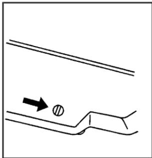
To open the liftgate if this happens, remove the interior trim plug located at the base of the liftgate from inside the vehicle.
