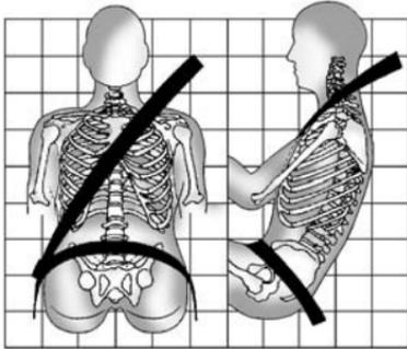
Sit up straight and always keep your feet on the floor in front of you. The lap part of the belt should be worn low and snug on the hips, just touching the thighs. In a crash, this applies force to the strong pelvic
