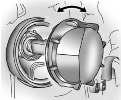
5. Turn the dust cap counterclockwise to remove.
