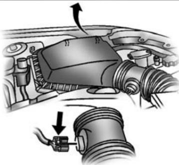
3. On the V8 engine, remove the airflow sensor connector by pushing in the tab and pulling straight back.
