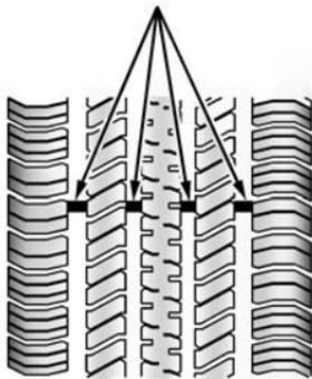
One way to tell when it is time for new tires is to check the treadwear indicators, which will appear when the tires have only 1/16 inch (1.6 mm) or less of tread remaining.
