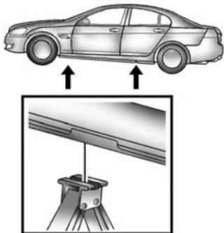
3. Position the jack lift head at the jack location nearest the flat tire. The location is indicated by a mark on the bottom edge of the vehicle. The jack must not be used in any other positions. Raise the jack until it engages with the jacking point.
