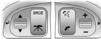
Some audio controls can be adjusted at the steering wheel.
