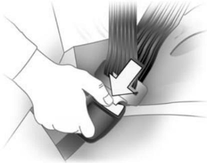
To unlatch the belt, push the button on the buckle. The belt should go back out of the way. When the safety belt is not in use, slide the latch plate up the safety belt webbing. The latch plate should rest on the stitching on the safety belt, near the guide loop on the side wall.
