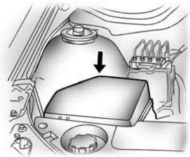
To open the fuse block cover, remove the clip on cover.
