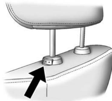
Pull the head restraint up to raise it. To lower the head restraint, press the button, located on the top of the seatback, and push the restraint down.
