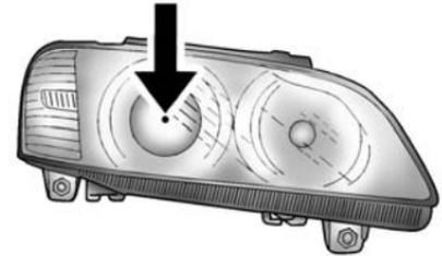
2. Locate the aim dot on the lens of the low-beam headlamp.
