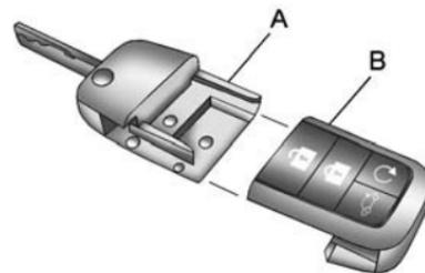
The key is purchased as two sections: the key blade and immobilizer section (A) and the remote keyless entry and remote start system section (B).
