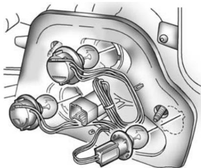
9. Push the new bulb into the socket and turn it clockwise to lock it into place.
