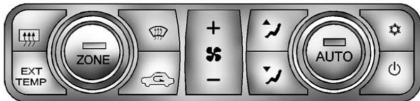
**⏻ (OFF):** Press to turn the climate control system off. Press any button to turn the system on again. While the climate control system is off the recirculation and rear window defogger can still be turned on.
