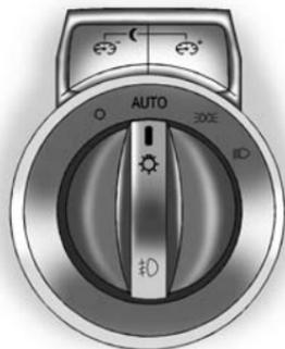
The exterior lamps control is located on the instrument panel to the left of the steering wheel.
