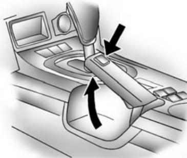
To set the parking brake, pull up on the parking brake handle. If the ignition is in the ON/RUN position, the brake system warning light will come on. See *Brake System Warning Light* on page 4-16.
