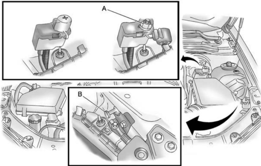
The positive jump start connection is covered by a red cap. Remove to expose the terminal.
