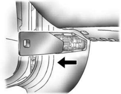
The instrument panel fuse block is located on the end of the instrument panel, on the driver's side of the vehicle. To access the fuses, open the fuse panel door by pulling out.
