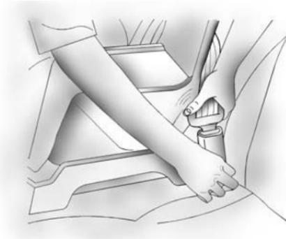
4. Push the latch plate into the buckle until it clicks. Make sure the release button is positioned so you would be able to unbuckle the safety belt quickly if necessary.
