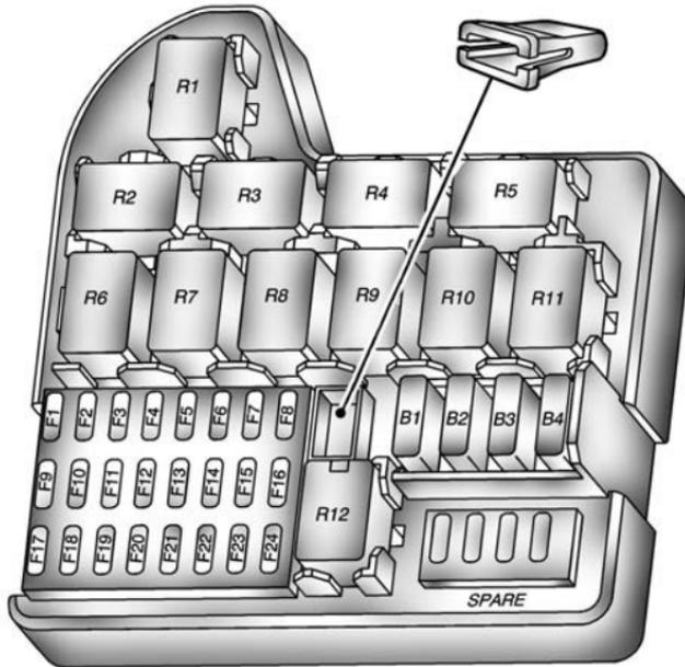
**Instrument Panel Fuse Block - Fuse Puller Shown**
