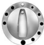
The sunroof control is located between the sun visors. It works when the ignition is in ON/RUN. The sunroof will not operate after the engine is turned off.
