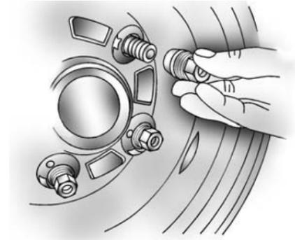
9. Remove all of the wheel nuts and place them in a dry, clean place to avoid getting dirt in the threads.
