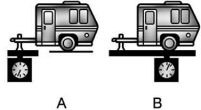
If you are using a weight-carrying hitch, the trailer tongue (A) should weigh 10 to 15 percent of the total loaded trailer weight (B).
