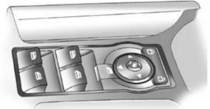
With the ignition on, move the selector switch located on the center console to the left or right to choose either the driver or passenger side mirror.
