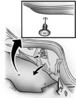
5. Turn the trunk lining securing pins counterclockwise and pull down at the same time to remove.
