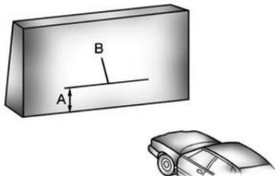
4. At the wall, measure from the ground upward (A) to the recorded distance from Step 3 and mark it.
