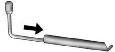
2. Use the fully extended wheel wrench to loosen all the wheel nuts one-half turn counterclockwise. Do not remove them yet.
