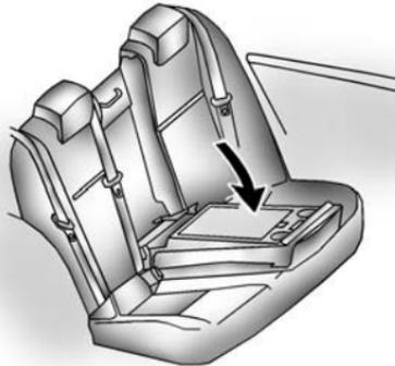
Press the button at the top of the seatback to release it, then fold it forward.
