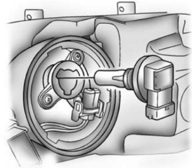
7. Turn the bulb socket counterclockwise and pull it out to remove from the lamp assembly.
