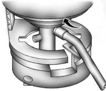
4. Turn the sealant canister so the inflator filling hose is aligned with the slot in the compressor.
