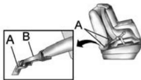
Lower anchors (A) are metal bars built into the vehicle. There are two lower anchors for each LATCH
