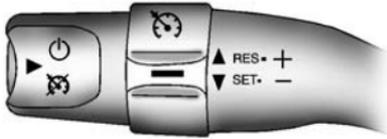
For vehicles with cruise control, the lever is located on the left side of the steering wheel.
