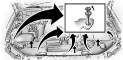
2. Remove the radiator support by turning the head screws counterclockwise and then pulling them straight out.
