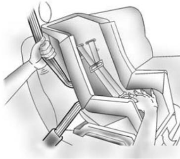
5. To tighten the belt, push down on the child restraint, pull the shoulder portion of the belt to tighten the lap portion of the belt, and feed the shoulder belt back into the retractor. If you are using a forward-facing child restraint, you may find it helpful to use your knee to push down on the child restraint as you tighten the belt.
