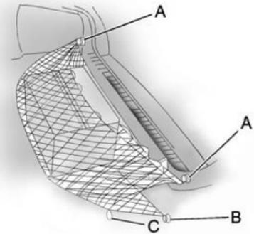
To install the net, attach each of the corner loops (A, B) to the four hooks inside the trunk, leaving the center loop (C) unhooked.
