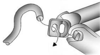
5. Fit the jack handle onto the jack by sliding the hook through the end of the jack.
