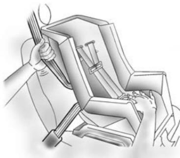
6. To tighten the belt, push down on the child restraint, pull the shoulder portion of the belt to tighten the lap portion of the belt and feed the shoulder belt back into the retractor. If you are using a forward-facing child restraint, you may find it helpful to use your knee to push down on the child restraint as you tighten the belt.
