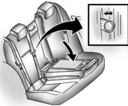
There is an emergency trunk release handle located inside the trunk on the trunk latch. Access the release handle by folding the rear seat center seatback. See *Rear Seat Operation* on page 1-5. Pull the release handle to open the trunk from the inside.
