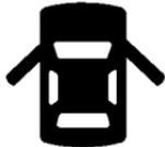
When the ignition is on, this light stays on until all doors are closed and completely latched.
