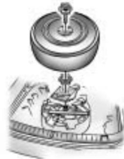
3. Turn the retainer nut counterclockwise and remove the spare tire.
