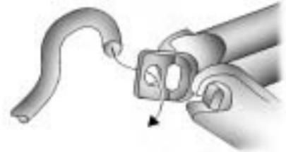
5. Fit the jack handle onto the jack by sliding the hook through the end of the jack.
