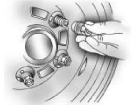
9. Remove all of the wheel nuts and place them in a dry, clean place to avoid getting dirt in the threads.
