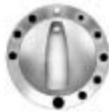
The sunroof control is located between the sun visors. It works when the ignition is in ON/RUN. The sunroof will not operate after the engine is turned off.
