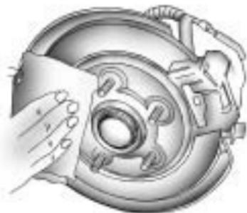
10. Remove any rust or dirt from the wheel bolts, mounting surfaces and spare wheel.
