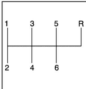
This is the shift pattern for the six-speed manual transmission.
