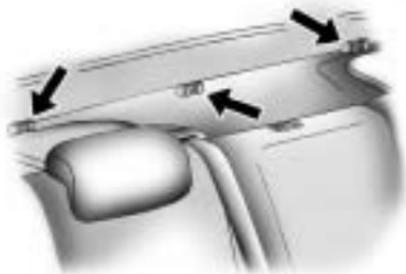
The top tether anchors are located on the rear seatback filler panel. Be sure to use an anchor located on the same side of the vehicle as the seating position where the child restraint will be placed.
