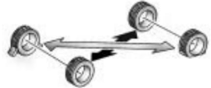
When you have a flat tire, place the wheel block at the tire diagonally across from the flat tire.
