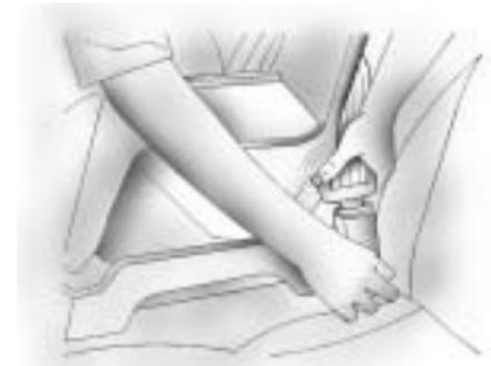
4. Push the latch plate into the buckle until it clicks. Position the release button, on the buckle so that the safety belt, could be quickly unbuckled if necessary.
