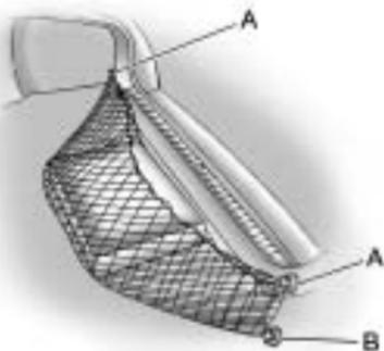
To create a pouch, attach the four corner loops (A) to each of the two top hooks. Attach the nets center loops (B) to the bottom hooks.
