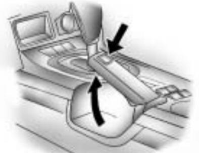
To set the parking brake, pull up on the parking brake handle. If the ignition is in the ON/RUN position, the brake system warning light will come on. See *Brake System Warning Light* on page 4-15.
