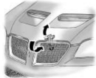
2. Pull up on the secondary hood release. The lever is located near the middle of the hood.
