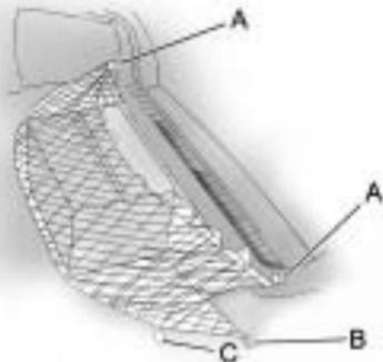
To install the net, attach each of the corner loops (A, B) to the four hooks inside the trunk, leaving the center loop (C) unhooked.
