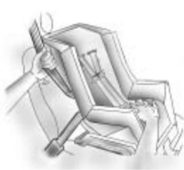
6. To tighten the belt, push down on the child restraint, pull the shoulder portion of the belt to tighten the lap portion of the belt and feed the shoulder belt back into the retractor. When installing a forward-facing child restraint, it may be helpful to use your knee to push down on the child restraint as you tighten the belt.
