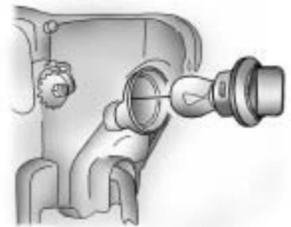
3. Turn the bulb socket counterclockwise and pull straight out.
