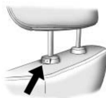
Pull the head restraint up to raise it. To lower the head restraint, press the button, located on the top of the seatback, and push the restraint down.
