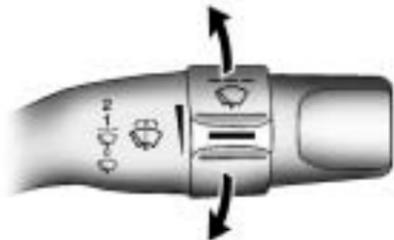
The windshield wiper/washer lever is located on the right side of the steering column.
