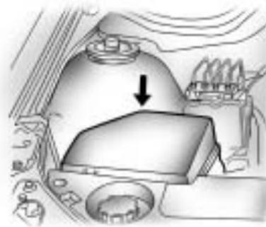
To open the fuse block cover, remove the clip on cover.
