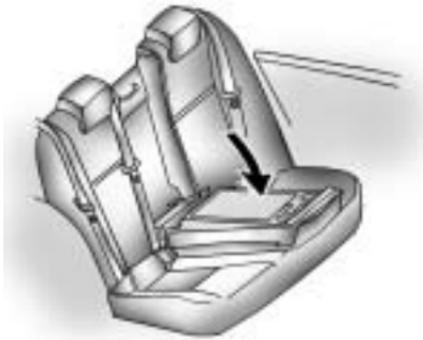
Press the button at the top of the seatback to release it, then fold it forward.
