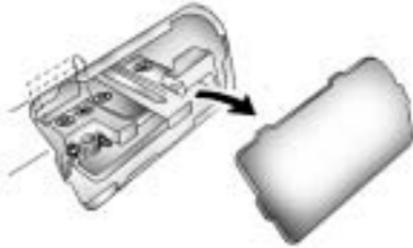
The rear compartment fuse block is located on the left side of the trunk behind a cover.
