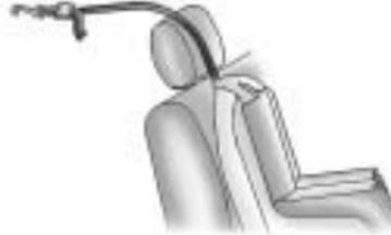
If the position you are using has a fixed headrest or head restraint and you are using a single tether, route the tether over the head restraint.
