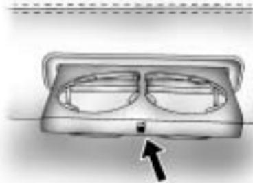
For vehicles with a rear seat cupholder, there is a cupholder on the front edge of the rear seat cushion. To open or close, press on the cupholder.
