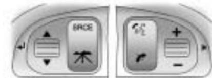
Some audio controls can be adjusted at the steering wheel.
