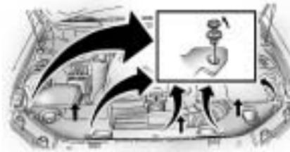
2. Remove the radiator support by unscrewing and prying out the head screws.
