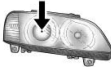
2. Locate the aim dot on the lens of the low-beam headlamp.
