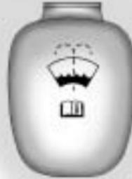
Open the cap with the washer symbol on it. Add washer fluid until the tank is full. See *Engine Compartment Overview* on page 9-6 for reservoir location.
