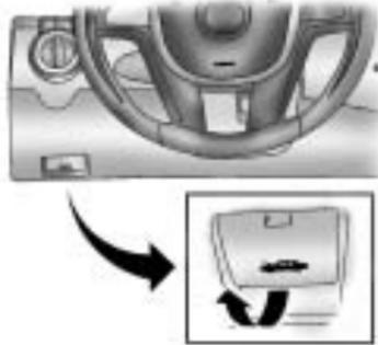
1. Pull the release handle with the above symbol on it. It is located below the instrument panel to the left of the steering wheel.
