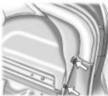
3. Turn the four convenience net hooks securing the plastic trunk trim counterclockwise.
