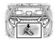
Attach the hooks to the indented slots on the sides of the rear cargo area.
