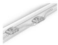
If the level of the shoulder is only slightly below the pavement, recovery should be fairly easy. Ease off the accelerator and then, if there is nothing in the way, steer so that the vehicle straddles the edge of the pavement. Turn the steering wheel 8 to 13 cm, 3 to 5 inches, (about one-eighth turn) until the right
