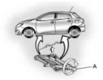
Position the jack and raise the jack lift head to fit over the car flange between the two notches.
