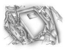
This engine compartment fuse block is located in the engine compartment on the driver side of the vehicle near the air cleaner. See Engine Compartment Overview on page 9-6.
