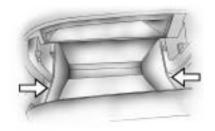
Open the glove box door. Push each side of the glovebox in and pull out to remove.
