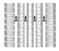
One way to tell when it is time for new tires is to check the treadwear indicators, which appear when the tires have only 1/16 inch (1.6 mm) or less of tread remaining. The vehicle needs new tires if any of the following statements are true:
