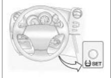
Press and hold the tire pressure warning reset switch until the tire pressure warning light flashes slowly on/off three times.
