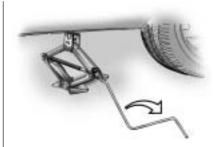
Turn the jack handle clockwise. Raise the vehicle far enough off the ground so there is enough room for the compact spare tire to fit underneath the wheel well.
