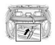
4. Attach the center hook to the center head restraint.
