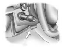
The adjustment lever is located on the left side of the steering column.
