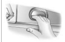
Close the liftgate by using the handle to pull it down.
