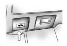
Pull the release handle, located below the instrument panel to the left of the steering wheel.
