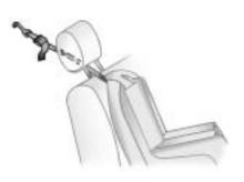
If the position you are using has an adjustable headrest or head restraint and you are using a single tether, raise the headrest or head restraint and route the tether under the headrest or head restraint and in between the headrest or head restraint posts.
