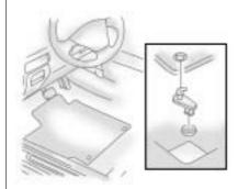
To remove the floor mat, pull up on the rear of the mat to disconnect it from the locator hooks.
