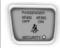
The words ON and OFF will be visible during the system check. When the system check is complete, either the word ON or the word
