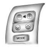
For vehicles with audio steering wheel controls some audio controls can be adjusted at the steering wheel. They include the following:
