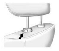
To lower the head restraint, press the button, located on the top of the seatback, and push the restraint down.
