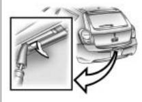
Press the tabs in to disengage them and remove the license plate lamp assembly.
