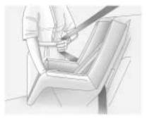
Pull the rest of the shoulder belt all the way out of the retractor to set the lock.
