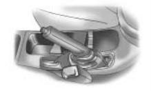
To release the parking brake, hold the brake pedal down. Pull the parking brake lever up until you can press the release button. Hold the release button in as you move the lever all the way down.
