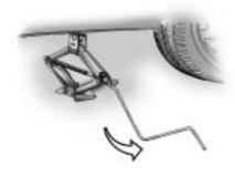
Turn the jack handle counterclockwise. Lower the jack completely.
