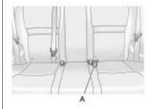
The buckle for the center rear passenger position (A) has the word CENTER on it.
