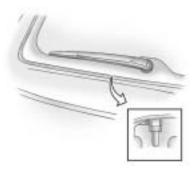
Disengage the two pins and disconnect the rear wiper arm by pulling them up.
