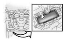
The fuse block is located under the instrument panel on the driver side of the vehicle.
