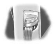
Push down on the release button and move the height adjuster to the desired position. The adjuster can be moved up by pushing on the front of the height adjuster.
