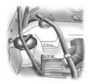
If you need more coolant, add the proper DEX-COOL® coolant mixture at the coolant recovery tank, but be careful not to spill it.
