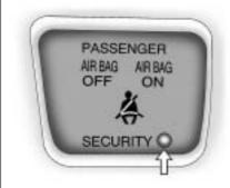
The security light is in the center of the instrument panel. It comes on if there is a problem with arming or disarming the theft-deterrent system. The security light flashes when the system is armed.
