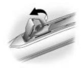
Push the release lever and slide the wiper assembly toward the driver side of the vehicle.
