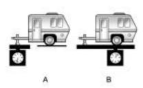
The trailer tongue (A) should weigh 10 to 15 percent of the total loaded trailer weight (B).
