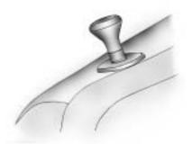
Pull up on the lock release knob, located on the top outboard side of the seatback.
