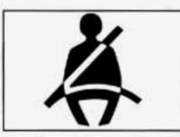
The safety belt light will also come on and stay on for about 20 seconds, then it will flash for about 55 seconds. If the driver's belt is already buckled, neither the chime nor the light will come on.
