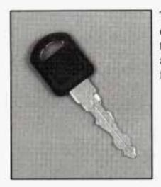
This vehicle has one double-sided key for the ignition, liftgate and door locks. It will fit with either side up.
