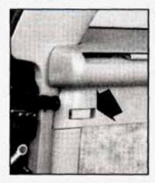
To remove the jack cover, pull up on the latch(es) on the cover. Remove the wheel blocks, jack and wheel wrench.
