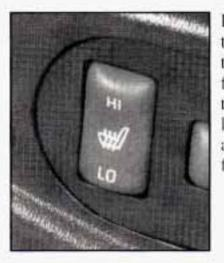
If you have this feature, the control is located on the side of the seat. This feature will quickly heat the lower cushion and lower back of the driver and front passenger seats for added comfort.
