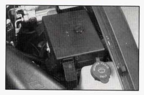
The fuse block is under the hood at the driver's side of the engine compartment.
