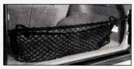
A convenience net in the rear of your vehicle helps keep small items, like gloves and light clothing in place during sharp turns or quick stops and starts.
