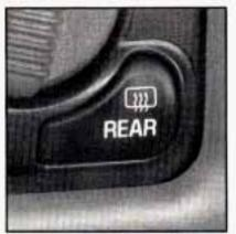
To turn on the rear window defogger, find the switch marked REAR with the defog symbol on the lower right corner of your climate control system.
