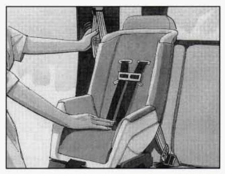
5. To tighten the belt, feed the shoulder belt back into the retractor while you push down on the child restraint. If you're using a forward-facing child restraint, you may find it helpful to use your knee to push down on the child restraint as you tighten the belt. Push and pull the child restraint in different directions to be sure it is secure.
