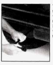
To remove the spare, insert the chisel end of the wheel wrench, on an angle, into the hole in the rear bumper. Be sure the chisel end of the wheel wrench connects into the hoist shaft.
