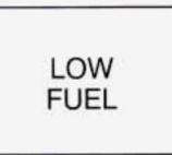
This light comes on when the fuel tank is low on fuel.
