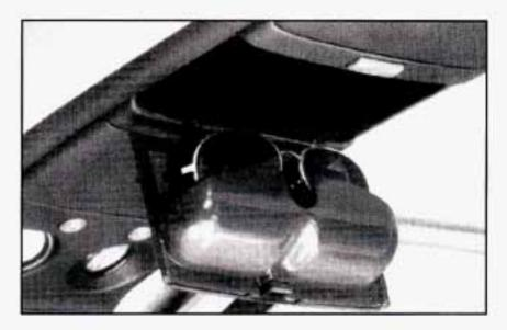
To open the sunglasses storage compartment in the overhead console, press the release button. Then pull the compartment down.
