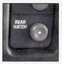
This button on the passenger's side of the steering column allows you to release the liftgate glass from inside the vehicle.
