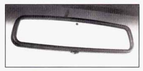
This mirror automatically changes to reduce glare from headlamps behind you. A photocell on the back of the mirror senses when it is becoming dark outside. Another photocell built into the mirror surface senses when headlamps are behind you. At night, when the glare is too high, the mirror will gradually darken to reduce glare (this change may take a few seconds). The mirror will return to its clear daytime state when the glare is reduced.
