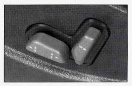
Move the lever under the front of the passenger's seat toward the driver's door to unlock it. Slide the seat to where you want it. Then release the lever and try to move the seat with your body to make sure the seat is locked into place. Horizontal Control: Raise the front of the seat by raising the forward edge of the button. Lower the front of the seat by lowering the forward edge of the button. Move the seat forward by moving the whole button toward the front of the vehicle.
