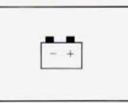
The charging system light will come on briefly when you turn on the ignition, but the engine is not running, as a check to show you it is working.
