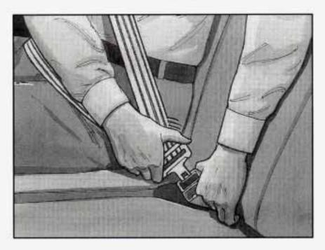
Pick up the latch plate and pull the belt across you. Don't let it get twisted. The shoulder belt may lock if you pull the belt across you very quickly. If this happens, let the belt go back slightly to unlock it. Then pull the belt across you more slowly. 2. Push the latch plate into the buckle until it clicks.
