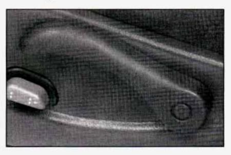
To adjust the seatback, lift the lever on the outer side of the seat.
