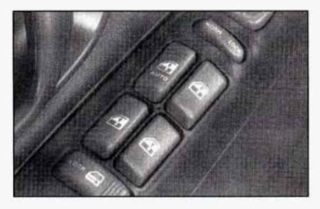
The power windows controls are on each of the side doors. With power windows, the switches control the windows when the ignition is on or when Retained Accessory Power (RAP) is present. (See "Retained Accessory Power" in the Index.) The driver's door has a switch for the passenger windows as well. There are individual controls on each of the side doors.
