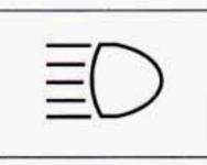
When the high beams are on, this indicator light on the instrument panel will also be on.
