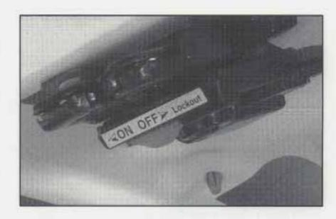
To turn the lockout on, slide the switch all the way to the left. To turn the lockout off, slide the switch all the way to the right.
