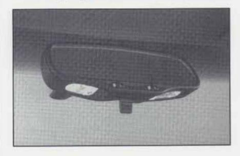
This mirror can be adjusted two ways. First, to adjust the angle of the mirror, move the mirror to a position that allows you see out the back window. To adjust the height of the mirror, adjust the arm that connects the mirror to the windshield.
