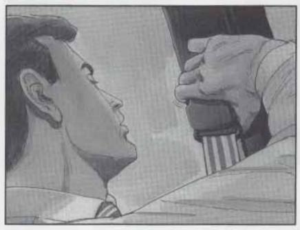
To move it down, squeeze the release button and move the adjuster to the desired position. You can move the adjuster up just by pushing up on the shoulder belt guide. After you move the adjuster to where you want it, try to move it down without squeezing the release button to make sure it has locked into position. Adjust the height so that the shoulder portion of the belt is centered on your shoulder. The belt should be away from your face and neck, but not falling off your shoulder.
