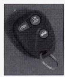
In addition, the system illuminates the interior lights for a set period of time. The remote lock control system consists of a receiver, which is located in the vehicle, and two hand-held transmitters.
