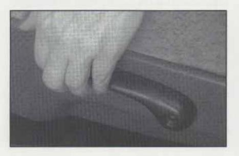
To adjust the seatback, lift the lever on the outer side of the seat and move the seatback to where you want it. Release the lever and ensure the handle returns to the original position and the seatback is securely locked.
