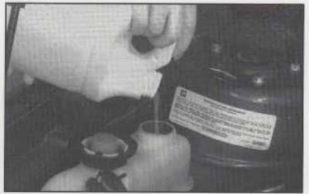
Then fill the coolant surge tank with the proper mixture, up to FULL COLD mark or slightly higher.
