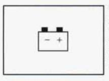
The charging system indicator light will come on when you turn on the ignition, but the engine is not running, as a check to show you it is working.
