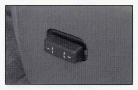
The power seat button is located on the lower, left side of the driver's seat. This button allows you to move the seat up, down, forward and backward. It also moves the front of the seat up or down and the rear of the seat up or down. Move the seat higher by lifting and holding the bottom of the button. Lower the seat by pushing and holding the top of the button.
