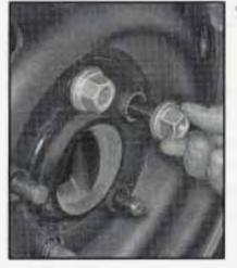
Replace the wheel nuts with the cone end of the nuts toward the wheel Tighten each nut by hand or with the wheel wrench until the wheel is held against the hub.
