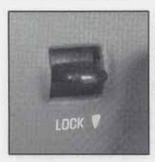
With the power door locks, you can unlock or lock all of the doors of your vehicle from the driver's or front passenger's door lock switch.
