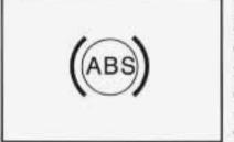
With the anti-lock brake system, this light will come on when you turn your ignition on or start your engine and it will stay on for three seconds. That's normal.
