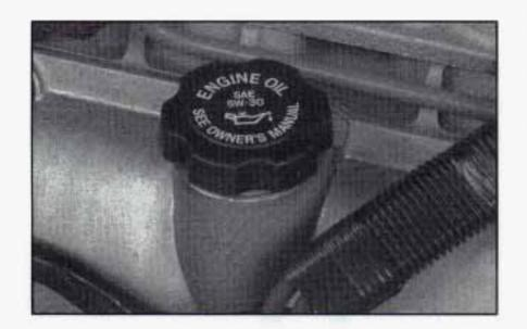
The engine oil fill cap is located on the front of the engine.
