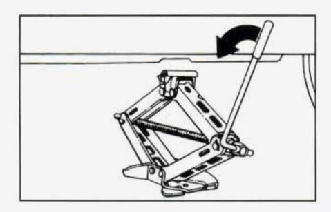
Lower the vehicle by turning the wheel wrench to the left. Lower the jack completely.
