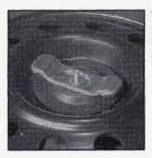
Turn the wing nut to the left and remove it. Then lift off the adapter and remove the spare tire.
