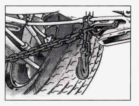
Attach T-hook chains to the T-hook slots in the floor pan support rails, just ahead of the rear wheels, on both sides. These slots are to be used when loading and securing to car-carrier equipment.
