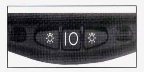
The mirror includes two map lamps, automatic dimming function and an eight-point compass display in the upper corner of the mirror face. When the compass display is turned on, the compass automatically calibrates as the vehicle is driven.
