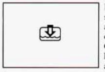
If this light comes on, your system is low on coolant and the engine may overheat. See "Engine Coolant" in the Index and have your vehicle serviced as soon as you can.
