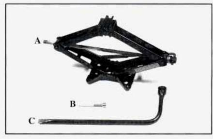
The tools you'll be using include the jack (A), extension and protector/guide (B) and wheel wrench (C). Removing the Flat Tire and Installing the Spare Tire
