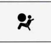
There is an air bag readiness light on the instrument panel, which shows an air bag symbol.
