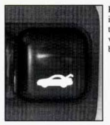
Press the button on the instrument panel to unlock the trunk from inside your vehicle. Your vehicle must be in PARK (P).
