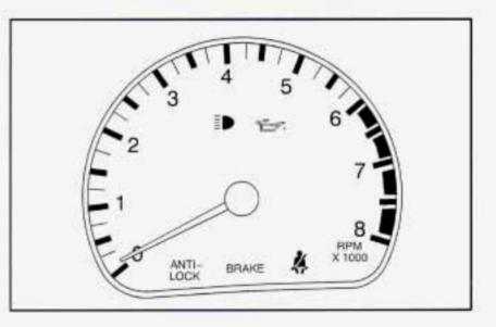
Your trip odometer (trip mode) tells you how far you have driven since you last reset it. To set it to zero, press the TRIP RESET button on the left side of the instrument panel. The tachometer displays the engine speed in thousands of revolutions per minute (rpm).
