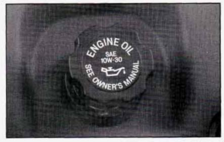
Be sure to fill it enough to put the level somewhere in the proper operating range. Push the dipstick all the way back in when you're through.
