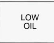
If the LOW OIL light on the instrument panel comes on, it means you need to check your engine oil level right away.
