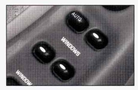
Switches on the driver's door armrest control each of the windows when the ignition is on. In addition, each passenger door has a switch for its own window.
