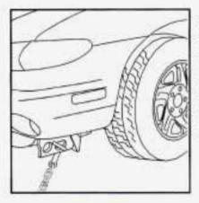
Attach T-hook chains in front of the wheels, into the slots of the front shipping brackets on the cradle (both sides). Insert the hook from the inward side of the slot and not the outward side.
