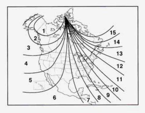
Press and hold both map lamp buttons on the bottom of the mirror, between five and eight seconds, until the zone number appears in the display.  Press the right lamp button to increase the zone numbers or press the left lamp button to decrease the zone numbers. After you have selected your zone number, the display will show a compass direction after five seconds. (Compass calibration may be necessary. See "Compass Calibration" following.)
