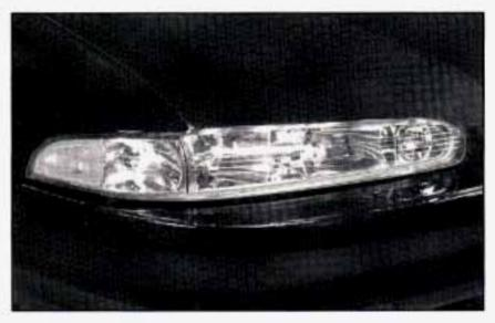
Your vehicle has a modular headlamp system. These headlamps have horizontal and vertical aim indicators. The aim has been optically pre-set at the factory and should need no further adjustment.
