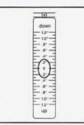
It is recommended that the upper limit not exceed plus 0.4 degrees from the center of the bubble. Other drivers may flash their high beams at you if your adjustment is much above plus 0.4 degrees. If you find that the headlamp aiming needs adjustment, follow these steps:
