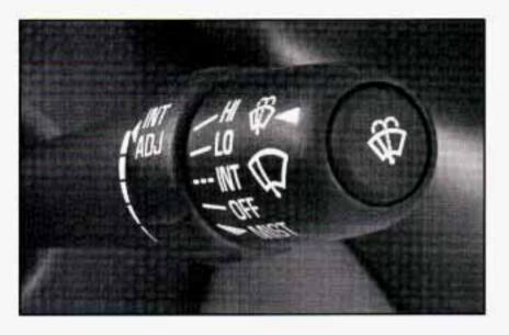
At the end of the right-hand lever on the steering wheel, there is a wiper symbol. To spray washer fluid on the windshield, push the button on the end of the lever. The wipers will run for several sweeps and then either stop or return to your preset speed.
