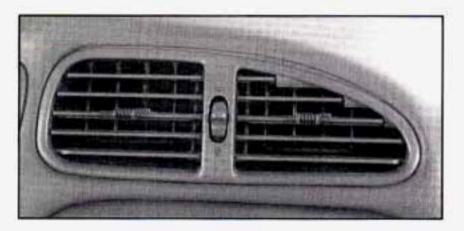
Adjust the direction of airflow by moving the louvered vents. To completely shut off airflow to the outlet move the thumbwheel down. To open the outlet for airflow move the thumbwheel up.
