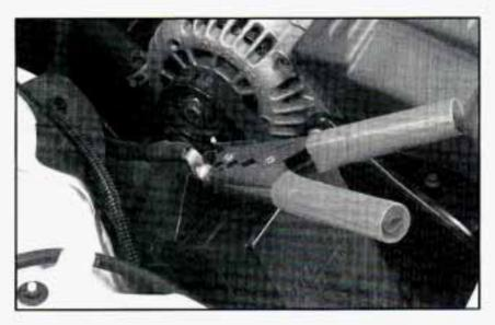
Connect the red positive (+) cable to the positive (+) terminal of the vehicle with the dead battery. Use a remote positive (+) terminal.
