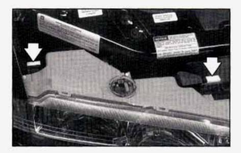
Pull straight up on the two headlamp retainers to release the assembly locator tabs. At the same time hold the headlamp assembly in position by applying a little pressure against the headlamp lens. This prevents the lamp from falling out.
