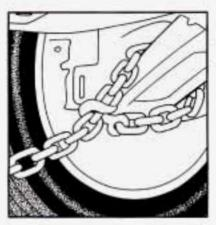
Attach a separate safety chain around the outboard end of each lower arm.
