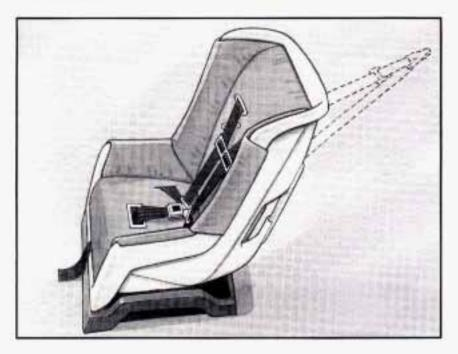
If your child restraint has a top strap, it should be anchored. If you need to have an anchor installed, you can ask your Oldsmobile retailer to put it in for you. If you want to install an anchor yourself, your retailer can tell you how to do it.
