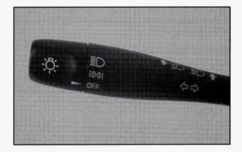
■D Turn the end of the lever to this symbol to turn on the headlamps and other operating lamps.
