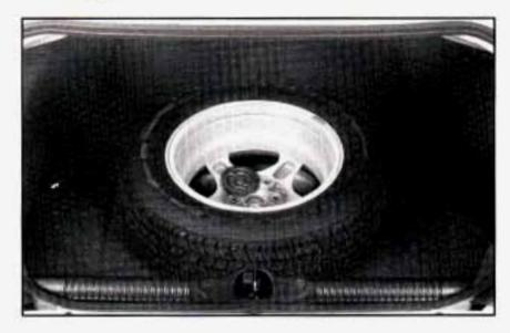
When storing a full-size tire you must use the extension to help avoid wheel surface damage. Use extension and protector/guide located in foam holder.
