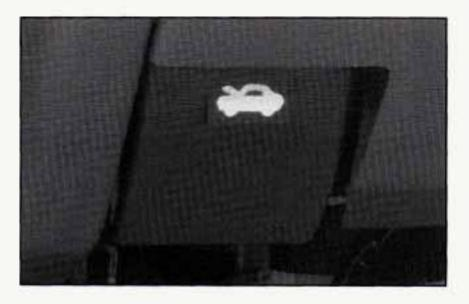
To open the hood, first pull the handle inside the vehicle. It is located below the instrument panel on the left-hand side.
