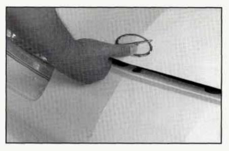
Then go to the front of the vehicle and release the secondary hood release. Lift the hood.
