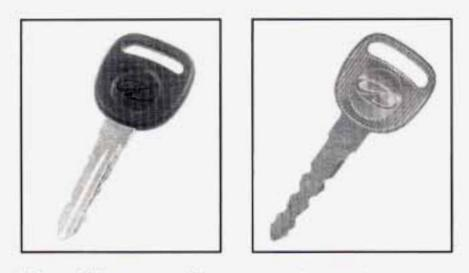
Your vehicle comes with two master keys and one spare key. The master key can be used for the ignition, as well as all door locks, trunk and storage compartments. The third key is provided as a spare key. These keys don't have key plugs. Your Oldsmobile retailer or Roadside Assistance has a code for your key.
