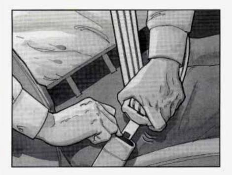
To unlatch the belt, just push the button on the buckle. The belt should go back out of the way.
