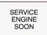
Your vehicle is equipped with a computer which monitors operation of the fuel, ignition and emission control systems.
