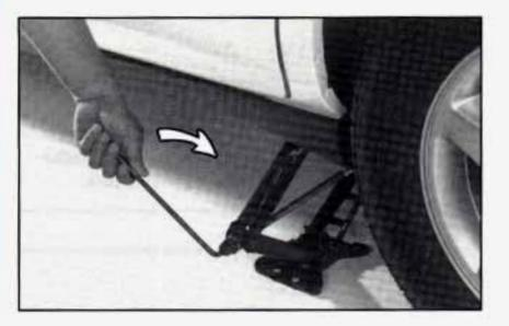
Raise the vehicle by turning the jack handle to the right. Raise the vehicle far enough off the ground for the spare tire to fit under the vehicle.
