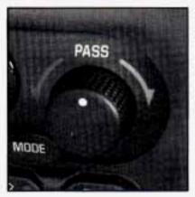
The right (PASS) knob adjusts the air temperature on the passenger's side so it is warmer or cooler than the temperature set by the driver.
