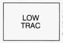
When your anti-lock system is adjusting brake pressure to help avoid a braking skid, this light will come on. See "Low Traction Light" in the Index.
