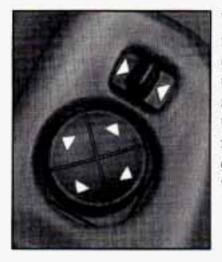
The power mirror control is near the driver's window, on the armrest. Switch the upper control to the left to adjust the left mirror or to the right to adjust the right mirror. Then press the lower control in the direction you want to move the mirror.
