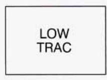
When your anti-lock system is adjusting brake pressure to help avoid a braking skid, this light will come on.
