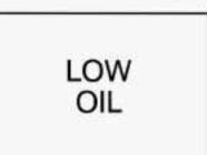
Your engine is equipped with an oil level monitoring system. When the ignition is turned on, the LOW OIL level light will briefly flash.
