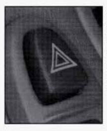
Press the switch located on your instrument panel to make your front and rear turn signal lamps flash on and off. Your hazard warning flashers work no matter what position your key is in, and even if the key isn't in.
