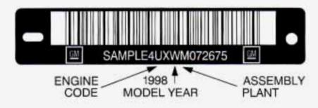
This is the legal identifier for your vehicle. It appears on a plate in the front corner of the instrument panel, on the driver's side. You can see it if you look through the windshield from outside your vehicle. The VIN also appears on the Vehicle Certification and Service Parts labels and the certificates of title and registration.
