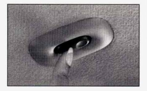
To open the power sunroof, press the rear of the switch once and the power sunroof will fully open. This is the express-open feature. During operation, press the switch again to stop the power sunroof at a desired position.
