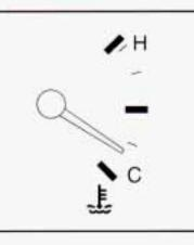
You have a gage that shows the engine coolant temperature. If the gage moves into the red area, your engine is too hot.
