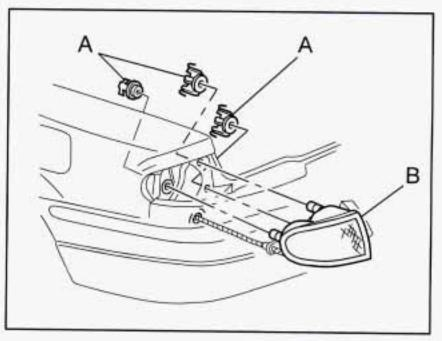
Remove the plastic wing nuts (A). (Pliers may be required to remove the wing nuts.)
