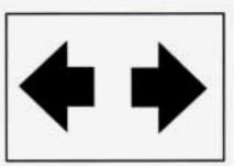
An arrow on the instrument panel will flash in the direction of the turn or lane change. To signal a lane change, just raise or lower the lever until the arrow starts to flash. Hold it there until you complete your lane change. The lever will return by itself when you release it.
