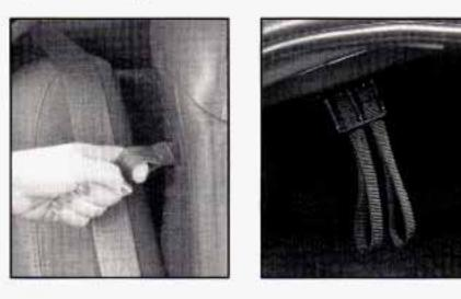
Pull the seat tab latch forward to fold down the rear seatback or pull the remote release straps in the trunk. To return the seat to its original position, push it back up and make sure it latches.
