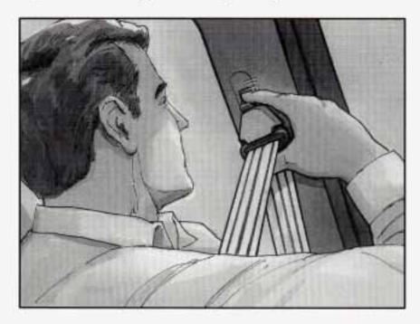
To move it down, squeeze the release lever and move the height adjuster to the desired position. You can move the adjuster up just by pushing up on the shoulder belt guide. After you move the adjuster to where you want it, try to move it down without squeezing the release lever to make sure it has locked into position.
