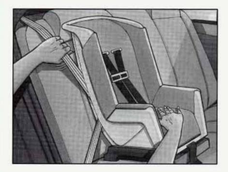
5. To tighten the belt, feed the shoulder belt back into the retractor while you push down on the child restraint. If you're using a forward-facing child restraint, you may find it helpful to use your knee to push down on the child restraint as you tighten the belt. Push and pull the child restraint in different directions to be sure it is secure.
