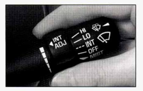
You can control the windshield wipers by turning the band with the wiper symbol on it. This lever is located on the right-hand side of the steering wheel. For a single wiping cycle, turn the band to MIST. Hold it there until the wipers start, then let go. the wipers will stop after one cycle. If you want more cycles, hold the band on MIST longer.
