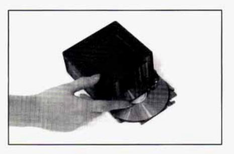
You must first load the magazine with discs before you can play a compact disc. Each of the 12 trays holds one disc. Press the button on the back of the magazine and pull gently on one of the trays. Load the trays from bottom to top, placing a disc on the tray label side down. If you load a disc label side up, the disc will not play and an error will occur. Gently push the tray back into the magazine slot. Repeat this procedure for loading up to 12 discs in the magazine.
