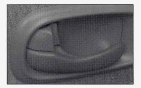
The rear doors do not have power door lock switches. The manual lever on each front and rear door works only on that door's lock. It won't lock or unlock all the doors.
