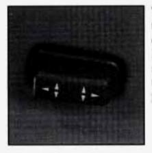
This switch is designed to imitate the movements of your seat cushion. It is located on the left side of the driver's or the right side of the passenger's seat cushion.
