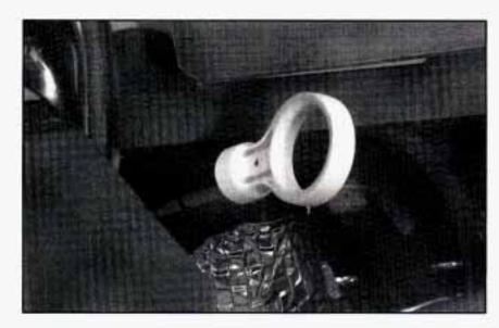
The engine oil dipstick is the yellow loop near the front of the engine.
