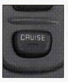
Push the cruise control button on the instrument panel to turn it on.
