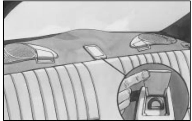
Anchor the top strap to this bracket. Once you have the top strap anchored, you'll be ready to secure the child restraint itself.
