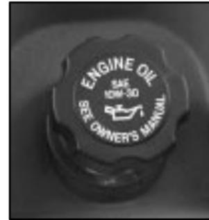
The engine oil fill cap is located toward the front of the engine compartment near the yellow looped engine oil dipstick.
