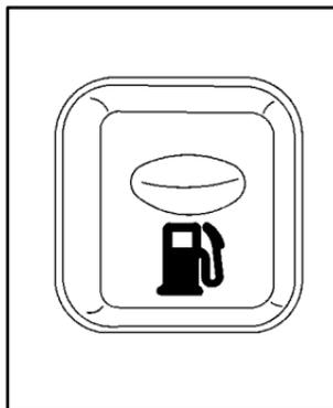
The button for the fuel door is located on the instrument panel, to the left of the steering column.
