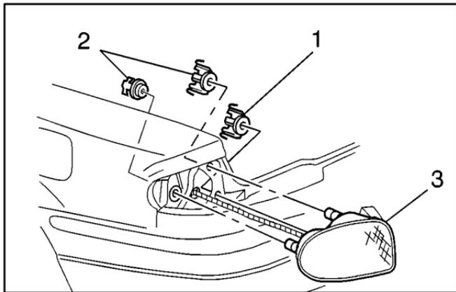
1. Unscrew the wing nut inside of the trunk (1) behind the taillamp to be changed (if equipped with a convenience net, unhook the net).
