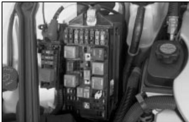
Some fuses are in the underhood electrical center on the passenger's side of the engine compartment.
