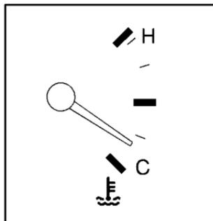
You have a gage that shows the engine coolant temperature. If the gage moves into the red area, your engine is too hot.
