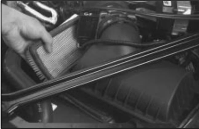
5. Hold the air box cover and air duct assembly up in position while removing the air filter element from the air box.
