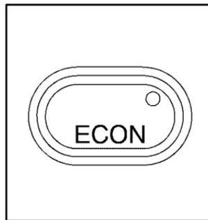
If your vehicle is equipped with this button, you can turn the compressor on and off.
