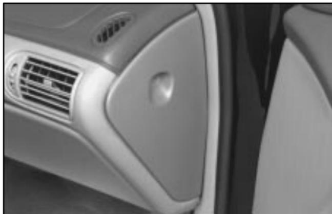
These fuses are located in a fuse block on the passenger's side of the instrument panel. Pull off the right side cover to expose the fuses.
