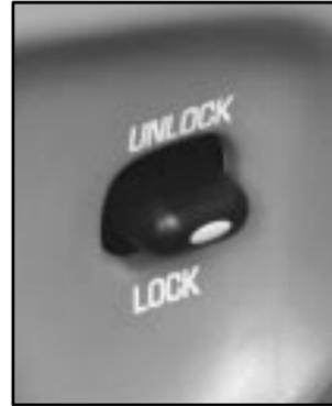
Press the power door lock switch located on the door near the handle to lock or unlock all doors.
