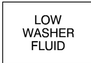
This light will come on when your ignition is on to check the bulb and will come on when your washer fluid is low.
