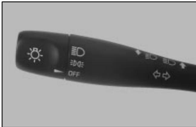
The lamp controls are located on the multifunction lever on the left of the steering wheel. They control these systems:
