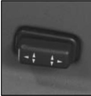
This switch is designed to imitate the movements of your seat cushion. It is located on the left side of the driver's or the right side of the passenger's seat cushion.
