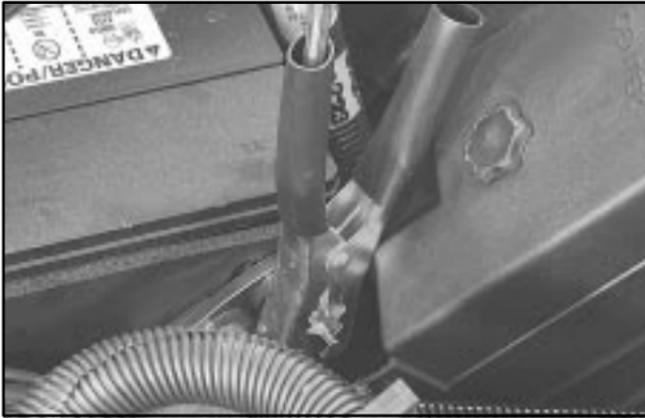
9. Now connect the black negative (-) cable to the good battery's negative (-) terminal.
