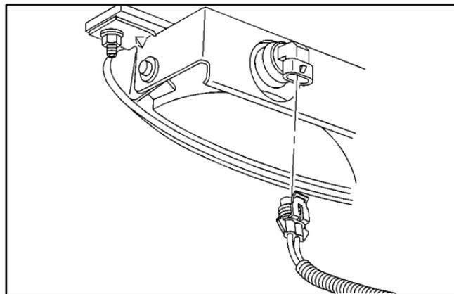
1. Remove the deflector located below the front fascia by removing the two bolts.
