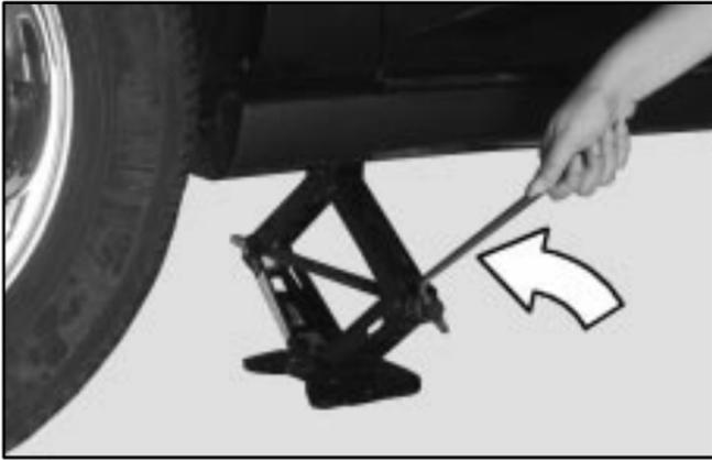
7. Lower the vehicle by turning the jack handle counterclockwise. Lower the jack completely.
