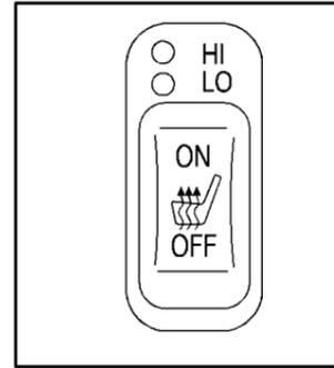
If your vehicle is equipped with this feature, both the driver's and passenger's heated seat switches are located on the instrument panel near the comfort controls. The driver's switch is on the left, and the passenger's on the right.
