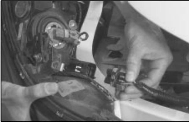
3. Disconnect the wiring harness from the headlamp assembly.
