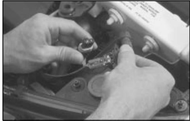
4. Lift the tabs to remove the bulb from the assembly.
