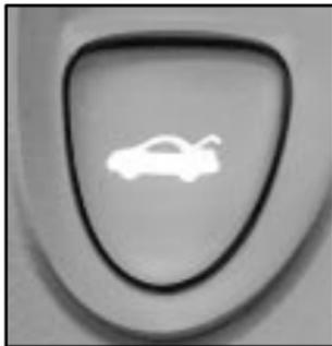
Press the trunk release button located on the lower portion of the driver's door to release the trunk lid. The trunk release lockout switch must be OFF for this button to work.
