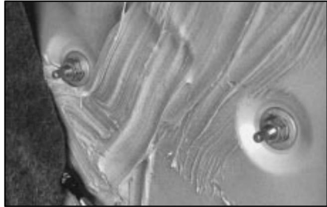
4. Remove the three 10 mm nuts holding the lamp in place and remove the lamp assembly.
