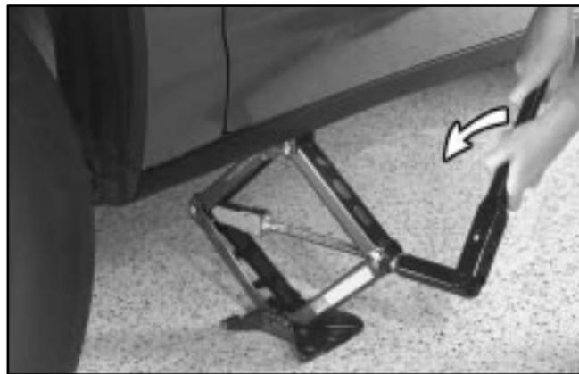
10. Lower the vehicle by turning the wheel wrench counterclockwise on the jack. Lower the jack completely.
