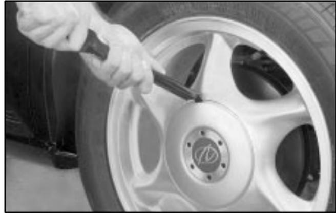
Insert the hooked end of the wheel wrench in one of the two small notches in the center cover and pry the cover off. Do not drop the cover or lay it face down, as it could be scratched or damaged.
