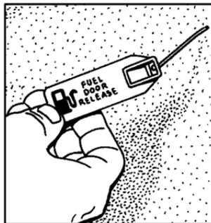
To do so, first open the trunk. The release mechanism is located on the driver's side of the vehicle, at the top of the trunk compartment. Pull the tab toward you to release the fuel door.
