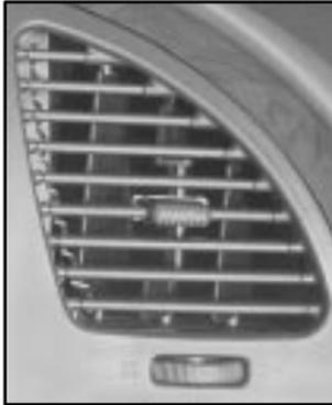
The direction of the air can be controlled by adjusting or closing the outlets in the instrument panel.
