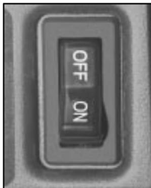
The trunk release lockout switch in the glove box allows you to secure items in the trunk and disable the fuel door release and the HomeLink<sup>®</sup> Transmitter.
