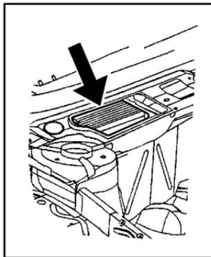
The passenger compartment air filter is located on the passenger side at the base of the windshield and can be accessed through a removable panel under the hood of the vehicle. See “Engine Compartment Overview” in the Index for more information on location.
