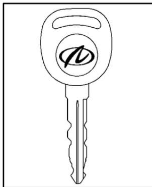
Your vehicle is equipped with the PASS-Key III (Personalized Automotive Security System) theft-deterrent system. PASS-Key III is a passive theft-deterrent system.
