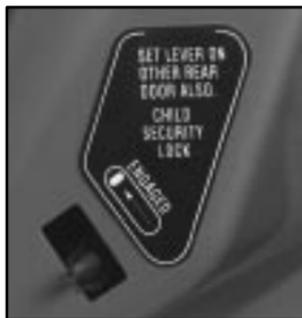
Your vehicle is equipped with rear door security locks that help prevent passengers from opening the rear doors of your vehicle from the inside.
