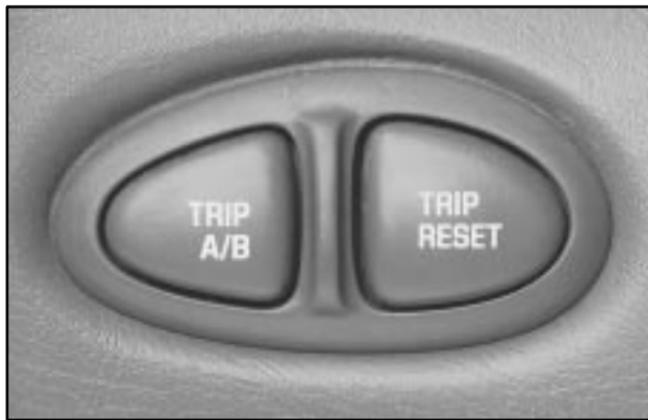
Press the TRIP A/B button to change which trip odometer is displayed.
