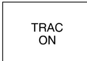
When your traction control system is limiting wheel spin, this light will come on.
