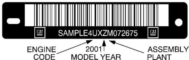
This is the legal identifier for your vehicle. It appears on a plate in the front corner of the instrument panel, on the driver's side. You can see it if you look through the windshield from outside your vehicle. The VIN also appears on the Vehicle Certification and Service Parts labels and the certificates of title and registration.
