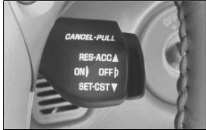
1. Push the cruise control switch located at the end of the lever in to ON.
