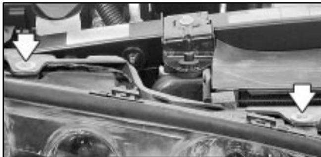
1. Remove the two bolts with a 10 mm socket.
