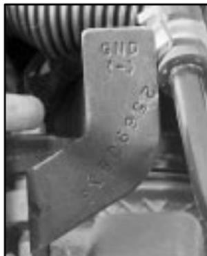
If you have the 4.0L V8 engine, your vehicle has a remote negative terminal, marked "GND", located near the power steering fluid reservoir. Attach the cable to the remote negative terminal provided.
