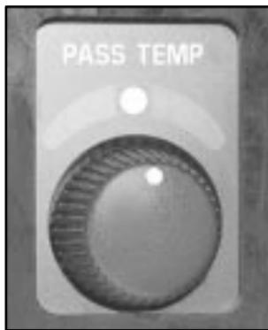
With this feature, the right front seat passenger can control the comfort setting for their own zone. To use this feature, turn the knob on the passenger's door to a cooler or warmer setting.
