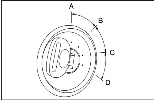
**LOCK (A):** This is the only position in which you can remove the key. This position locks your ignition, steering wheel and transaxle. It's a theft-deterrent feature.
