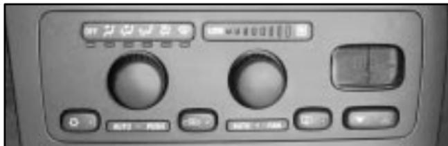
Your vehicle is equipped with either a Single Zone or a Dual Zone Automatic Electronic Climate Control System. You can use the automatic setting or override the automatic setting by using the manual controls. Your vehicle also has the flow-through ventilation system described later in this section.
