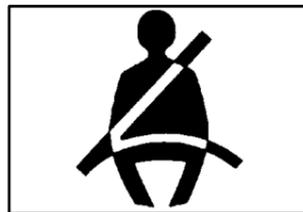
The safety belt light will also come on and stay on for about 20 seconds, then flash for about 55 seconds.
