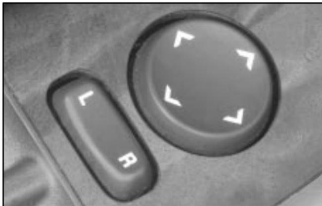
The controls on the driver's door operate both outside rearview mirrors. Move the L/R switch to the left (L) to select the driver's side rearview mirror, or to the right (R) to select the passenger's side rearview mirror.
