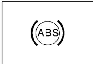
With the anti-lock brake system, the light(s) will come on when you start your engine and may stay on for several seconds. That's normal.
