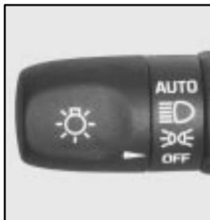
The headlamp control is located on the turn signal/multifunction lever.
