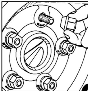
9. Put the wheel nuts back on with the rounded end of the nuts toward the wheel. Tighten each nut by hand until the wheel is held against the hub.
