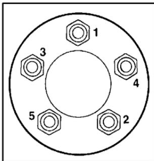
11. Using the wheel wrench, tighten the wheel nuts firmly in a crisscross sequence as shown.
