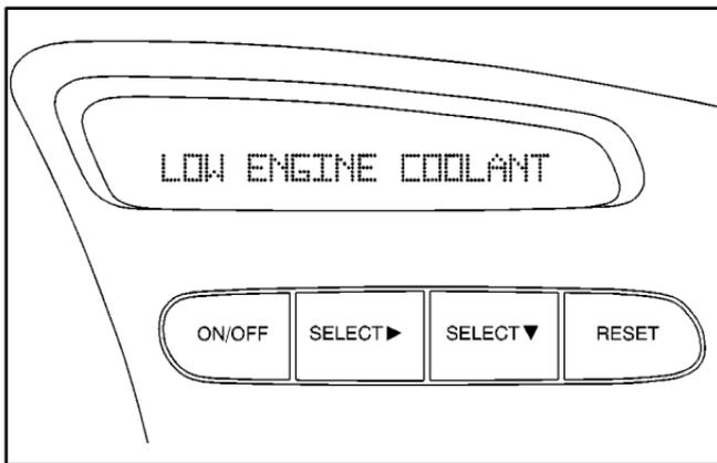
If the LOW ENGINE COOLANT DIC message comes on and stays on, it means you're low on engine coolant.
