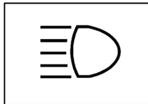
When the high beams are on, this light on the instrument panel cluster will also be on.
