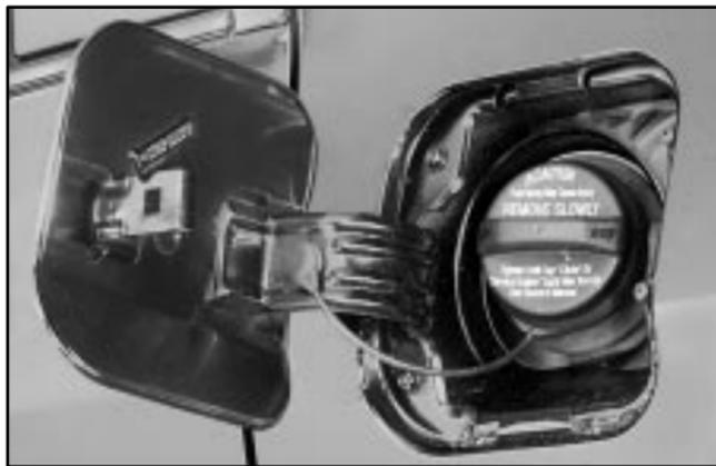
The cap is behind a hinged door on the driver's side of the vehicle.
