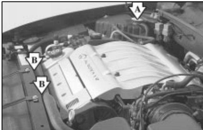
A. Coolant Surge Tank with Pressure Cap
