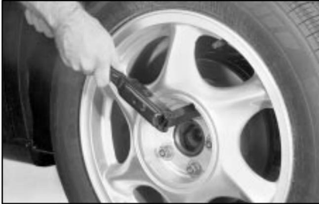
1. Position the wheel wrench securely over the wheel nuts to loosen, but don't remove them.
