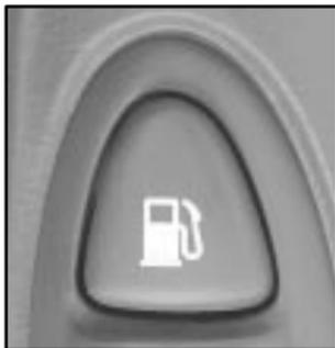
To open the fuel door, press the button located on the driver's door trim near the trunk release button.
