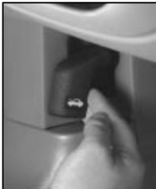
To open the hood, first pull the hood release handle, located to the left of the steering wheel under the instrument panel.
