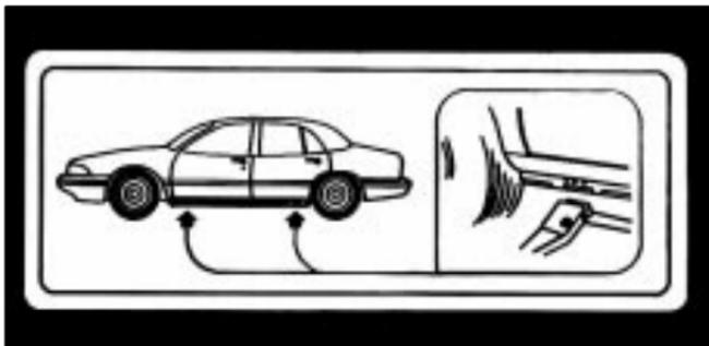
4. Near each wheel well is a notch in the frame to position the jack head. Position the jack under the vehicle and raise the jack head until it fits firmly against the sheet metal. Do not raise the vehicle yet. Put the compact spare near you.
