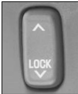
With power door locks, you can lock or unlock all the doors of your vehicle using the driver's or the front passenger's door lock switch.
