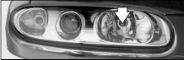
2. Measure the distance from the ground to the aim dot on each lamp; if left low beam, subtract two inches. Record this distance.
