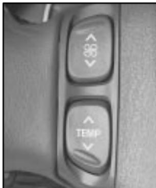
Some heating and cooling controls can be adjusted at the steering wheel. Other touch controls also operate some audio controls. See “Audio Steering Wheel Controls” later in this section.
