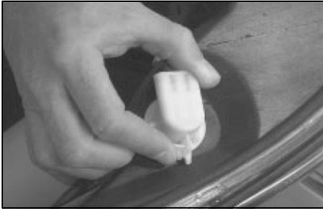
4. Tip the headlamp assembly and while pressing the release, turn the bulb and socket counterclockwise to remove them.
