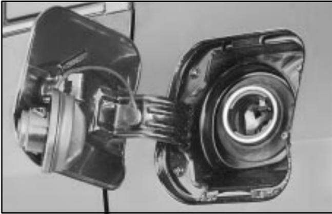
While refueling, hang the tethered cap from the hook on the fuel door.
