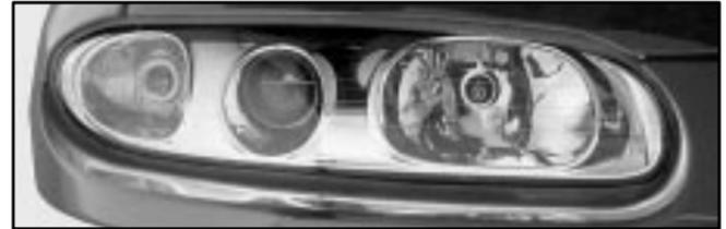
Your vehicle has a visual optical headlamp aiming system equipped with horizontal aim indicators. The aim has been pre-set at the factory and should need no further adjustment. This is true even though your horizontal aim indicators may not fall exactly on the “0” (zero) marks on their scales.
