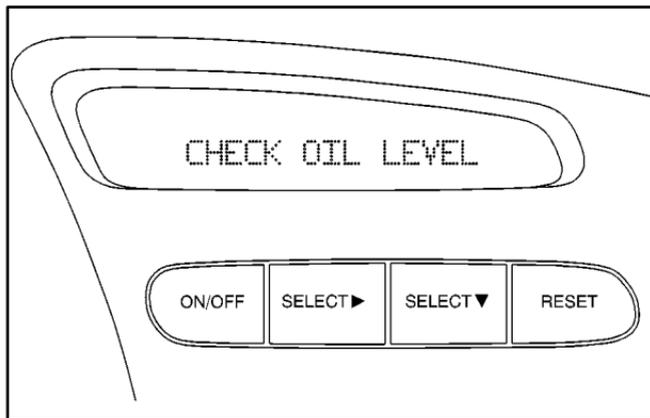
If the CHECK OIL LEVEL message appears on the instrument panel, it means you need to check your engine oil level right away. For more information, see “DIC Warnings and Messages” in the Index.
