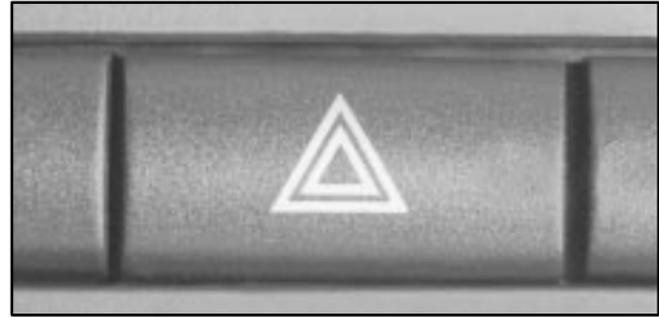
To turn on the hazard warning flashers, press and release the button located in the center of the instrument panel. The indicators for the turn signals will flash on and off.
