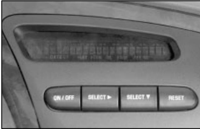
The Driver Information Center (DIC) displays information in either English or metric. When the system is on or off, push the ON/OFF button down for three seconds to change the display between English and metric. This will also change the digital screen for the climate control system between English and metric.
