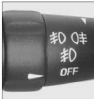
To turn on only the front fog lamps, turn the fog lamp band to the single fog lamp symbol. To turn on both the front and rear fog lamps, turn the fog lamp band to the double fog lamp symbol.
