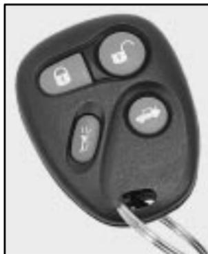
The driver's door will unlock and the exterior lights will flash twice when the unlock symbol is pressed.
