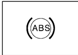
If there's a problem with the anti-lock brake system, this warning light will stay on. See "Anti-Lock Brake System Warning Light" in the Index.
