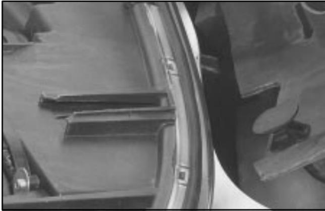
6. Slide the lamp assembly back into place by lining up the track on the bottom of the assembly with the guide on the vehicle. Then connect the outboard snap and secure the lamp assembly with the two bolts.
