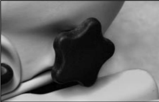
The knob that controls this feature is located on the outboard side edge of the seat. Turn the knob towards the front of the vehicle to increase lumbar support. Turn the knob towards the rear of the vehicle to decrease lumbar support.
