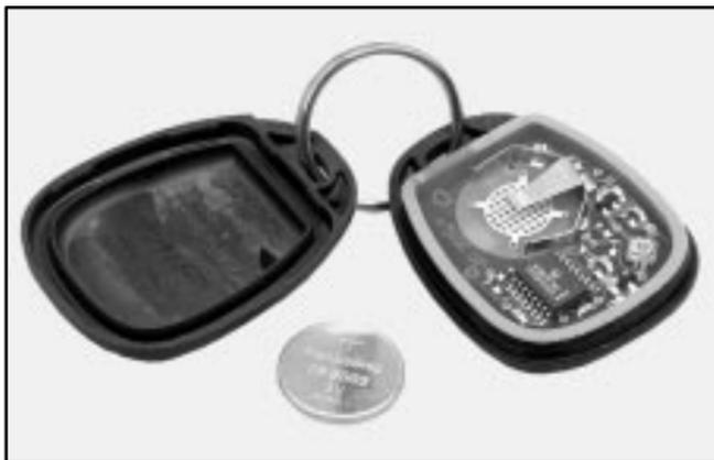
For battery replacement, use a Duracell® battery, type DL-2032, or a similar type.
