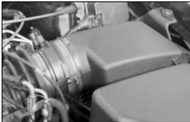
The engine air cleaner and filter are on the driver's side of the engine compartment. See "Engine Compartment Overview" in the Index for more information on location.
