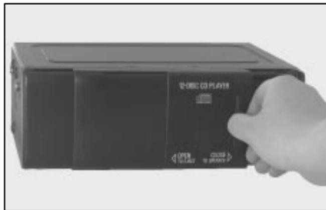
Close the door by sliding it all the way to the right. When the door is closed, the changer will begin checking for discs in the magazine. This will continue for up to one and a half minutes depending on the number of discs loaded.
