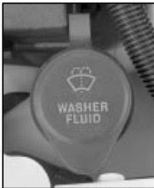
The windshield washer fluid reservoir is located at the front of the engine compartment on the passenger's side. See "Engine Compartment Overview" in the Index for more information on location.
