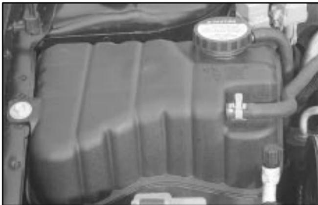
The engine coolant surge tank is located on the passenger's side of the engine compartment. See "Engine Compartment Overview" in the Index for more information on location.
