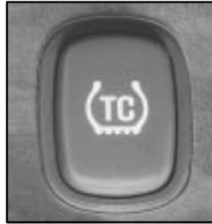
To turn the system off, press the TC button on the center console.
