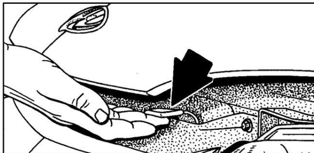
Then go to the front of the vehicle and pull up on the secondary hood release.
