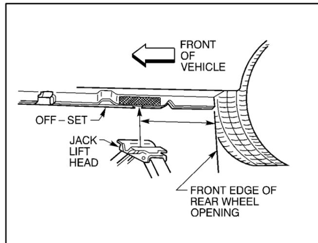
For jacking at the vehicle's rear location, put the jack lift head about 6 inches (15 cm) from the front edge of the rear wheel opening or just behind the off-set as shown.
