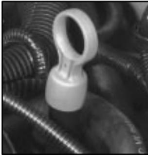
The transaxle fluid dipstick handle is the red loop near the rear of the engine compartment. See “Engine Compartment Overview” in the Index for more information on location.
