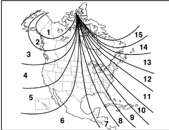
2. Make sure the compass is in calibration mode. See “Compass Calibration” in the Index. Press the on/off button to display the zone number.
