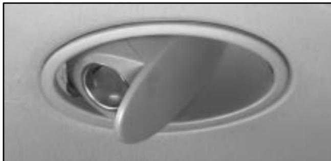
The accessory power outlets are located on the passenger's lower left side and below the comfort controls on the instrument panel.
