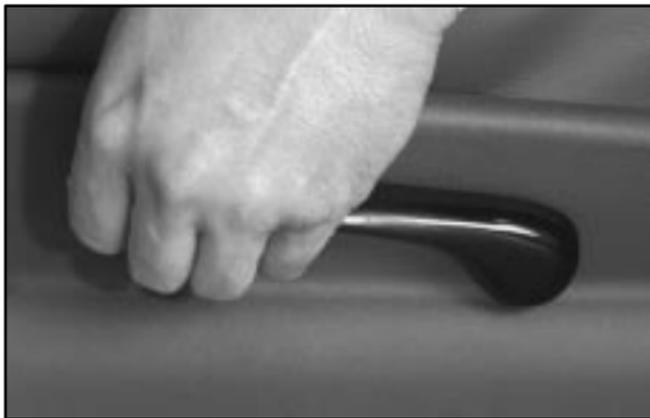
The levers for the driver's and the passenger's front seatbacks are located on the outboard side of each seat cushion. Lift the lever to release the seatback, then move the seatback to where you want it. Release the lever to lock the seatback in place. Pull up on the lever without pushing on the seatback and the seatback will move forward.
