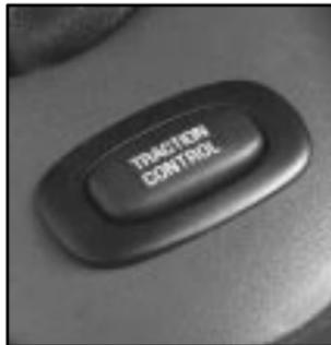
To turn the system on or off, press the TRACTION CONTROL button on the console.
