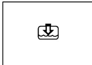
If this light comes on, your system is low on coolant, and the engine may overheat.
