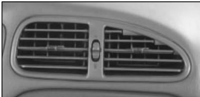
Adjust the direction of airflow by moving the vents. To completely shut off airflow to the outlet move the thumbwheel down. To open the outlet for airflow move the thumbwheel up.
