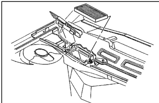
The passenger compartment air filter is located underneath the hood just below the windshield wiper arm on the passenger's side of the vehicle (underneath the air inlet grille).
