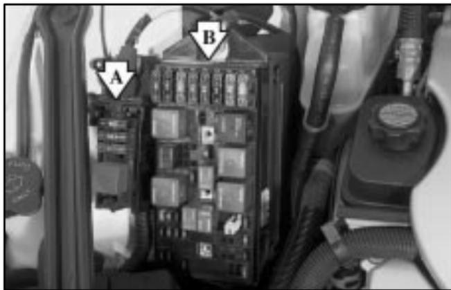
A. Accessory Wiring Junction Fuse Block
