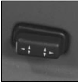
This switch is designed to imitate the movements of your seat cushion. It is located on the outboard side of both the driver's and the passenger's seat cushion.
