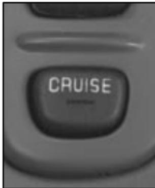
1. Press the CRUISE button on the right side of the instrument panel to turn it on. A light on the button will indicate that the system is on.
