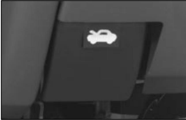
To open the hood, first pull the handle inside the vehicle. It is located below the instrument panel on the driver's side.
