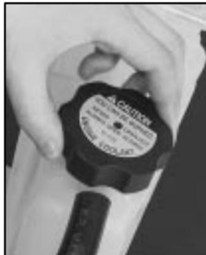
1. You can remove the coolant surge tank pressure cap when the cooling system, including the coolant surge tank pressure cap and upper radiator hose, is no longer hot.
