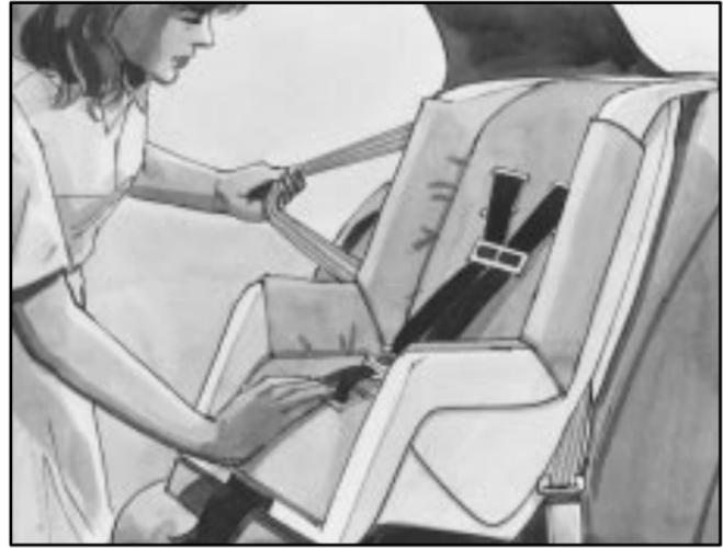
4. Some vehicles have a child restraint locking feature on the shoulder belt retractor. You can tell if your vehicle has this feature by pulling the shoulder belt all the way out of the retractor. Then, let the belt go back a few inches, and try to pull the belt out again. If you can't pull the belt out because it has locked, it means the retractor has the child restraint locking feature.
