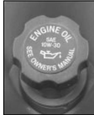
The engine oil fill cap is located toward the front of the engine compartment near the yellow looped engine oil dipstick. See "Engine Compartment Overview" in the Index for more information on location.
