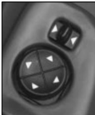
The power mirror controls are located near the driver's window, on the armrest.
