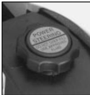
The power steering fluid reservoir is toward the middle of the engine compartment, on the passenger's side. See "Engine Compartment Overview" in the Index for more information on location.
