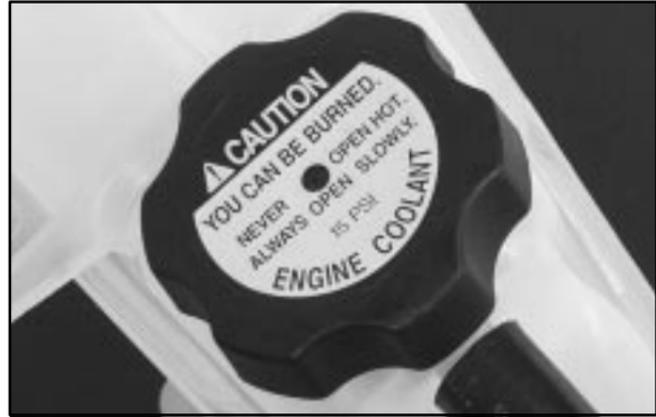
The coolant surge tank is located in the engine compartment toward the rear of the engine on the passengers' side of the vehicle. See "Engine Compartment Overview" in the Index for more information on location.
