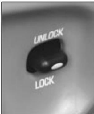
Press the power door lock switch located on either front door near the handle to lock or unlock all the doors.
