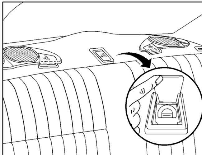
Anchor the top strap to one of these anchor points. Be sure to use an anchor point located on the same side of the vehicle as the seating position where the child restraint will be placed.
