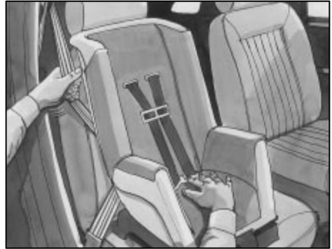
6. Push and pull the child restraint in different directions to be sure it is secure.
