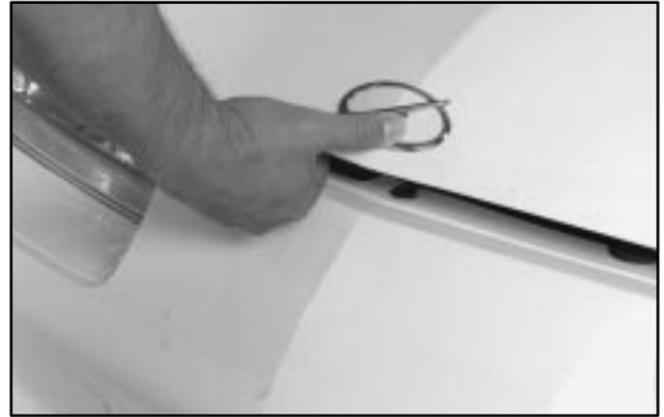
Then go to the front of the vehicle and release the secondary hood latch. Lift the hood.
