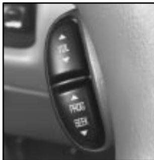
If your vehicle has this feature, you can control certain radio functions using the buttons on your steering wheel.
