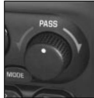
The PASS knob adjusts the air temperature on the passenger's side so it is warmer or cooler than the temperature set by the driver.
