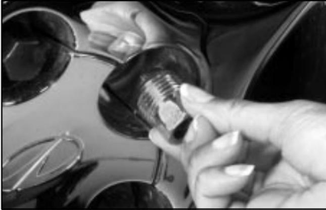
1. Using the wheel wrench, remove the plastic caps and loosen all of the wheel nuts. Don't remove them yet.
