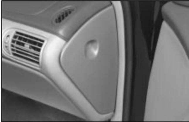
These fuses are located in a fuse block on the passenger's side of the instrument panel. Pull off the passenger's side cover to expose the fuses.
