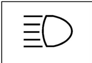
To change your headlamps from low beam to high beam, push the lever away from you. To change back to low beam, pull the lever toward you.
