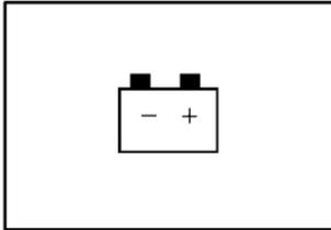
The charging system light will come on briefly when you turn the ignition key to ON as a check to show you it's working. Then it should go out.
