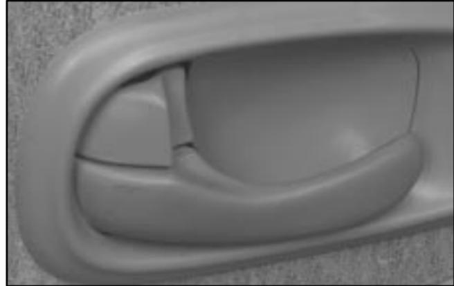
From the inside, use the manual lever. Each door has a lever that works only on that door's lock. The lever won't unlock or lock all the doors. Push the lever rearward to unlock and forward to lock.
