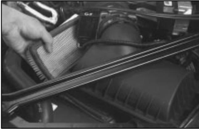
5. Hold the air box cover and air duct assembly up in position while removing the old air filter element from the air box.
