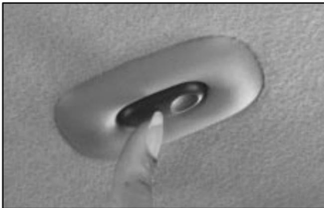
The sunroof includes a sliding glass panel and a sunshade. The switch works only when the ignition or retained accessory power (RAP) is active. See “Retained Accessory Power (RAP)” in the Index.
