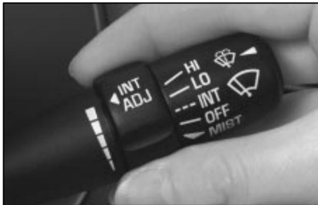
You can control the windshield wipers by moving the lever with the wiper symbol on it up or down. This lever is located on the right side of the steering wheel.
