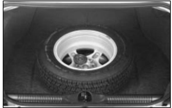
When storing a full-size tire, you must use the extension to help avoid wheel surface damage. Use the extension and protector/guide located in the foam holder. To store a full-size tire, place the tire in the trunk with the valve stem facing down and the protector/guide through a wheel bolt hole. Remove the protector and attach the retainer securely. When returning the compact spare to the trunk, put the protector/guide back in the foam holder. Store the cover as far forward as possible.
