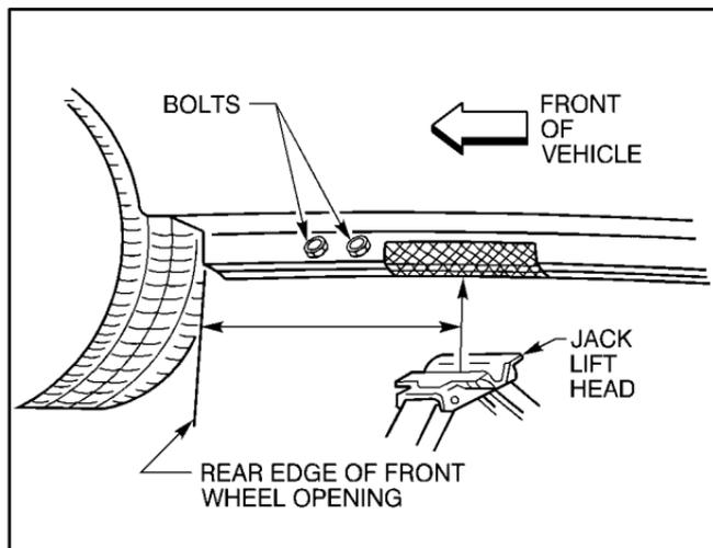
For jacking at the vehicle's front location, put the jack lift head about 8 inches (20 cm) from the rear edge of the front wheel opening or just behind the two bolts as shown.
