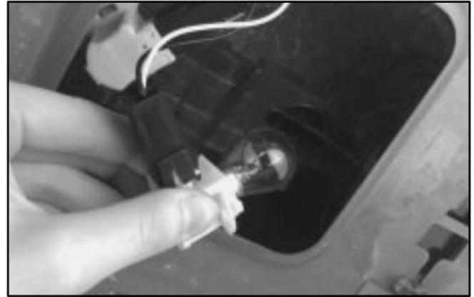
3. Remove the old bulb from the socket by turning it one quarter turn counterclockwise.
