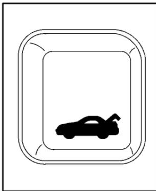
Press the button on the left side of the instrument panel to unlock the trunk from inside your vehicle. Your vehicle must be in PARK (P).
