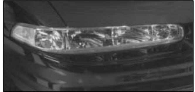
Your vehicle has a headlamp system equipped with horizontal and vertical aim indicators. The aim has been pre-set at the factory and should need no further adjustment. This is true even though your vertical and horizontal aim indicators may not fall exactly on the “0” (zero) marks on their scales.
