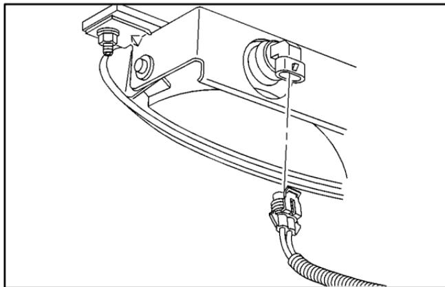
2. Reach up from underneath the front of the vehicle and remove the electrical connector from the bulb assembly.
