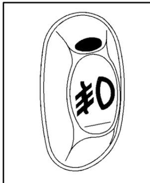
To turn the fog lamps on, press the top of the fog lamp switch located on the left side of the instrument panel.
