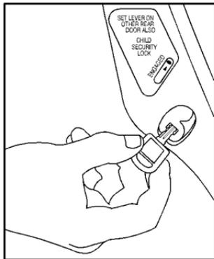
Your vehicle is equipped with rear door security locks that help prevent passengers from opening the rear doors of your vehicle from the inside.
