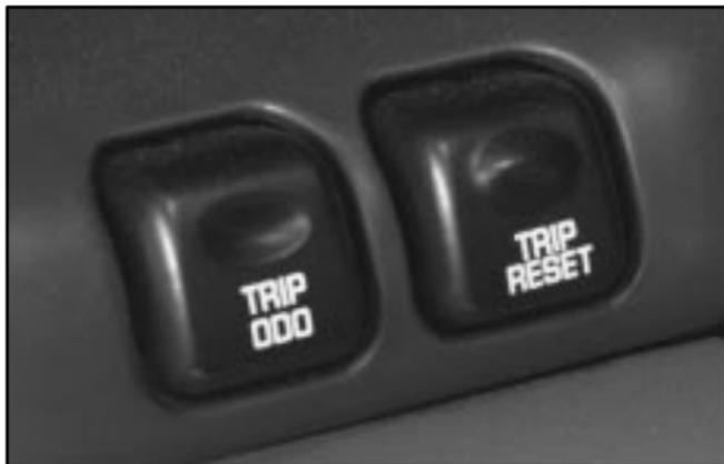
Your trip odometer (trip mode) tells you how far you have driven since you last reset it. To set it to zero, press and hold the TRIP RESET button on the left side of the instrument panel for two to three seconds.
