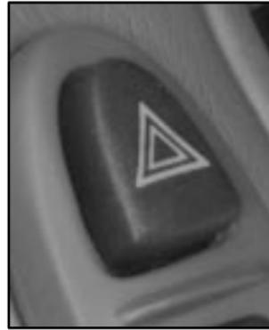
Press the switch located on your instrument panel to make your front and rear turn signal lamps flash on and off.
