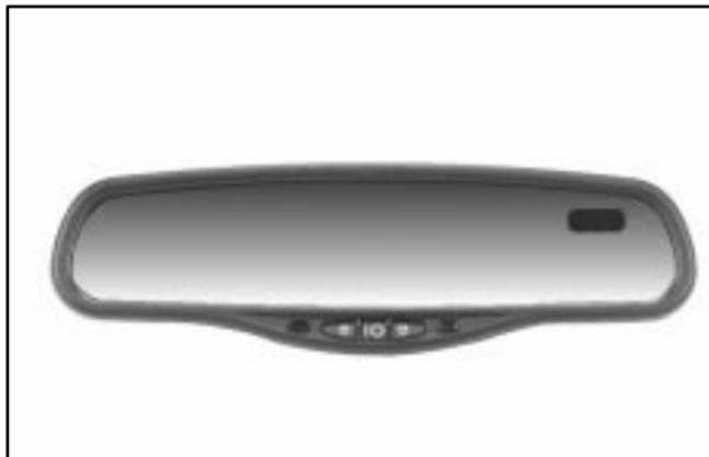
This mirror automatically changes to reduce glare from headlamps behind you. A time delay feature prevents rapid changing from the day to night positions while driving under lights and through traffic.
