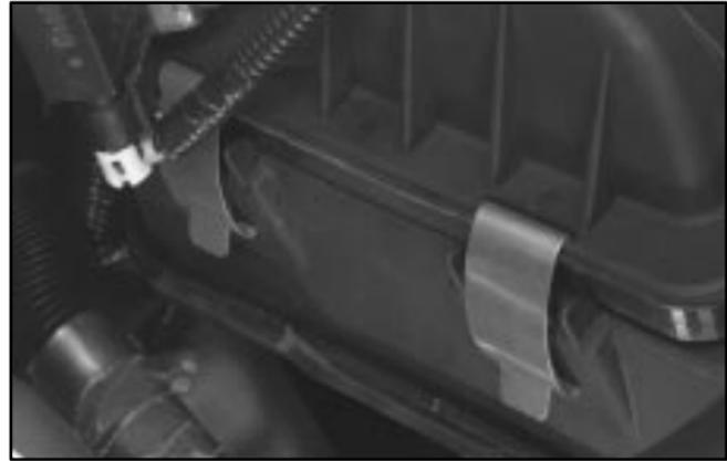
3. Unhook the two hold-down clips located on the air box cover.
