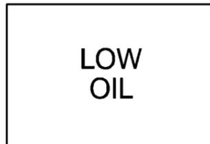
Your engine is equipped with an oil level monitoring system. When the ignition is turned to ON, the LOW OIL light will briefly come on.
