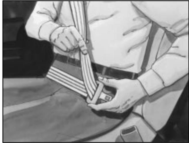
If the belt stops before it reaches the buckle, tilt the latch plate and keep pulling until you can buckle the belt.
