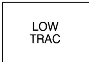
When the Precision Control System is active, the LOW TRAC light will come on.
