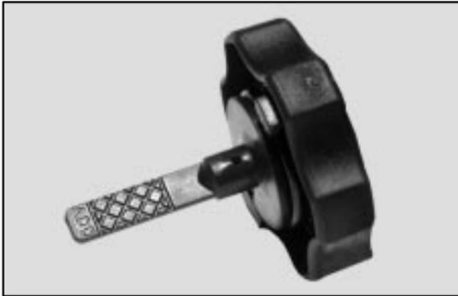
The level should be at the the cross-hatched area. If necessary, add only enough fluid to bring the level up to the mark.
