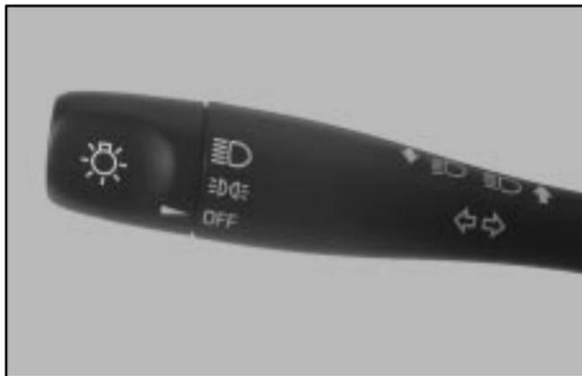
The lamp controls are located on the multifunction lever on the left of the steering wheel. They control the following systems:
