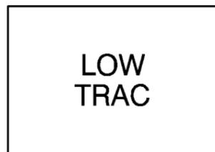
This light will come on when your traction control system is limiting wheel spin. See “Traction Control System Active Light” in the Index.
