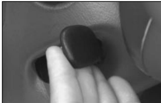
A tilt wheel allows you to adjust the steering wheel before you drive. You can also raise it to the highest level to give your legs more room when you exit and enter the vehicle.
