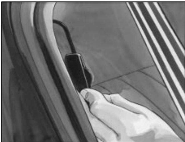
1. Pull the elastic cord out from between the edge of the seatback and the interior body to remove the guide from its storage clip.
