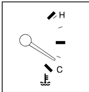
You have a gage that shows the engine coolant temperature. If the gage moves into the shaded area near the hot mark, your engine is too hot.
