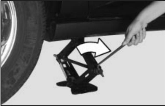
3. Raise the vehicle by turning the jack handle clockwise. Raise the vehicle far enough off the ground for the spare tire to fit under the vehicle.
