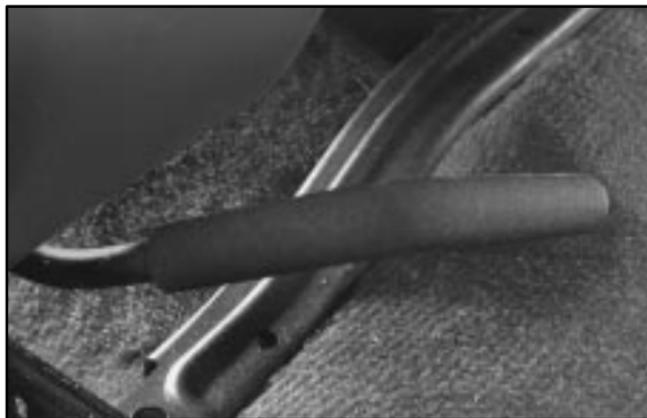
Lift the lever, located under the front of the seat, upward using a twisting motion. This will unlock the seat. Slide the seat to where you want it and release the lever. Try to move the seat back and forth with your body to be sure the seat is locked into place.
