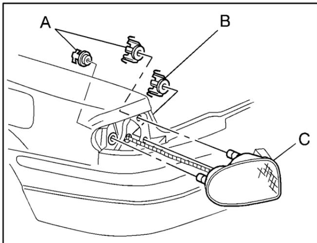
1. Unscrew the wing nut inside of the trunk (B) behind the taillamp to be changed. If equipped with a convenience net, unhook the net.
