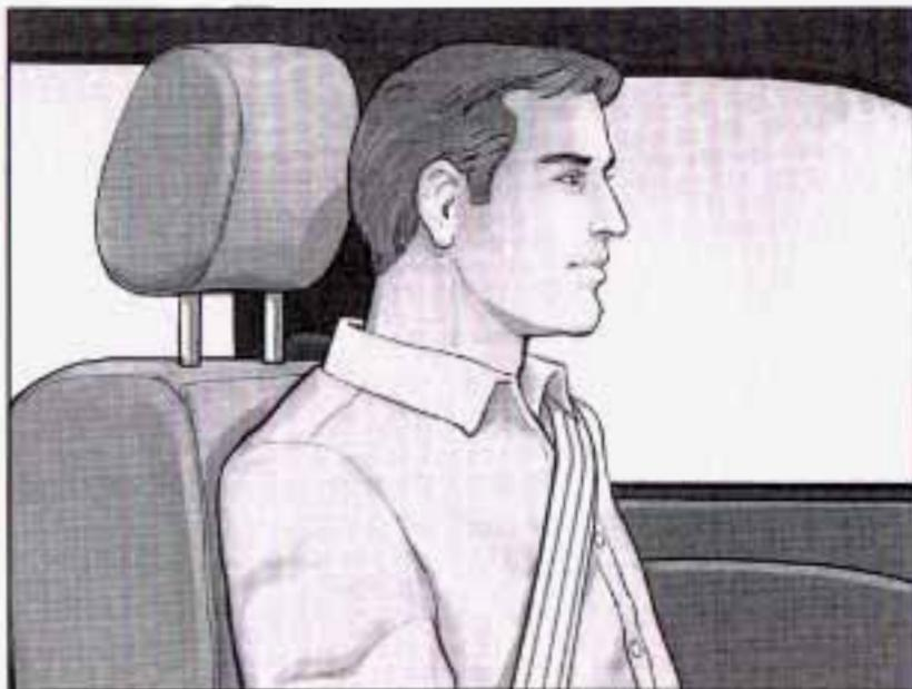
Adjust your head restraint so that the top of the restraint is closest to the top of your head. This position reduces the chance of a neck injury in a crash.
