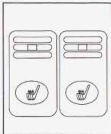
Your vehicle may have this feature. If it does, the heated seat switches are located in the instrument panel switchbank.
