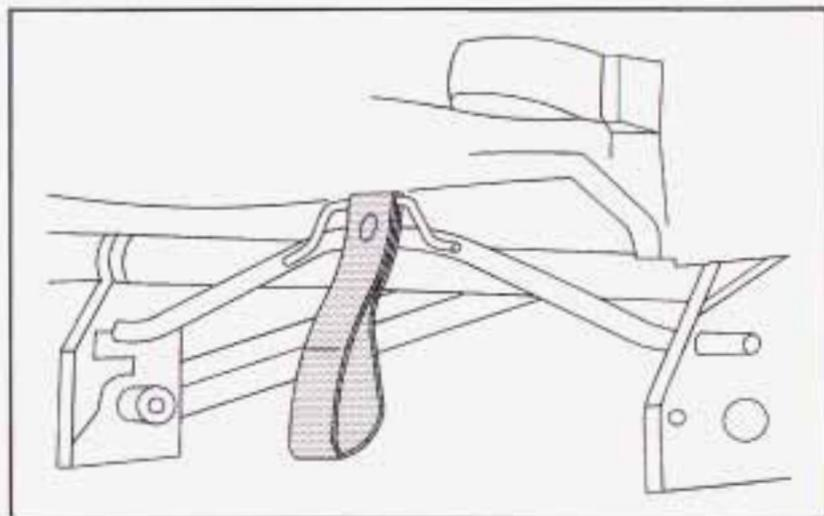
2. From behind the bench seat, pull the nylon strap at the center of the base of the seat to release the rear latches from the floor pins.
