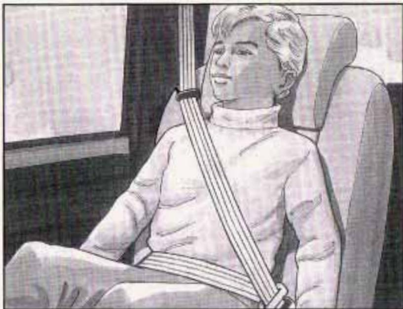
4. Buckle, position and release the safety belt as described in *Rear Seat Passengers on page 1-39*. Make sure that the shoulder belt crosses the shoulder.
