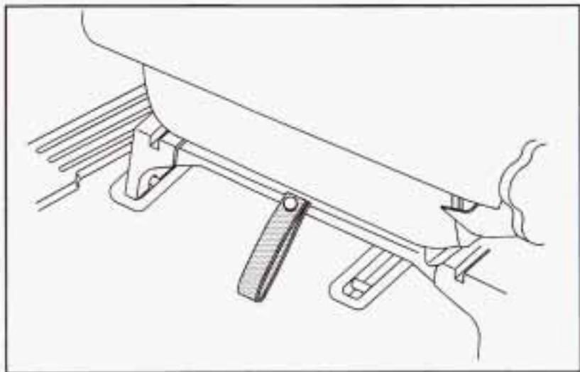
1. Pull the nylon strap behind the chair to release the rear hooks from the floor pins.
