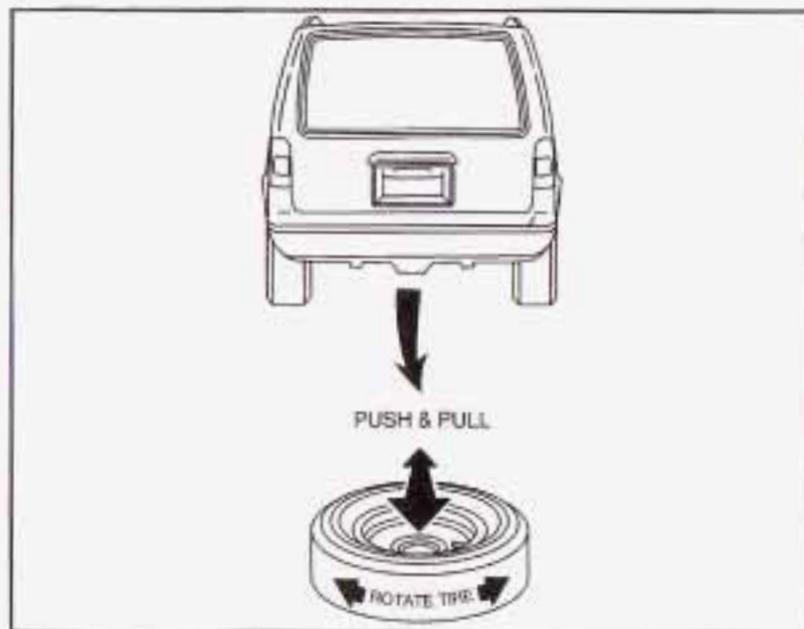
6. Make sure the tire is stored securely. Push, pull, and then try to rotate or turn the tire. If the tire moves, use the folding wrench to tighten the cable. Put back all tools as they were stored in the jack storage compartment and put the compartment cover back on.
