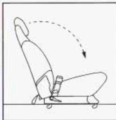
2. Fold the seatback flat on the seat, by either pulling on the nylon strap on the rear of the seat or lifting up on the lever located on the front of the seatback. If the seat adjusts, slide it all the way back.
