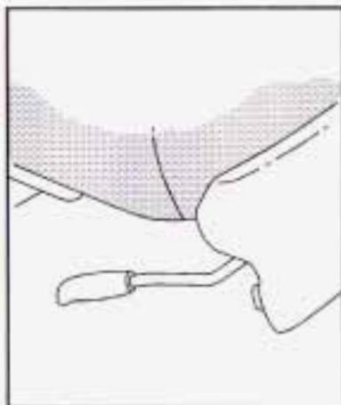
Use the lever located on the front of the seat to adjust the seat forward or rearward. Pull up the lever to unlock the seat. Slide the seat to where you want it and release the lever.
