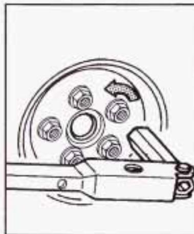
1. Loosen the wheel nuts – but do not remove them – using the folding wrench. (Turn the handle about 180 degrees, then flip the handle back to the starting position. This avoids taking the wrench off the lug nut for each turn.)
