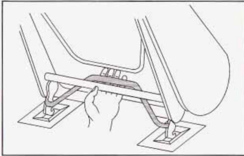
1. Squeeze the angled bar toward the solid crossbar while placing the front hooks of the bench seat onto the front two floor pins.
