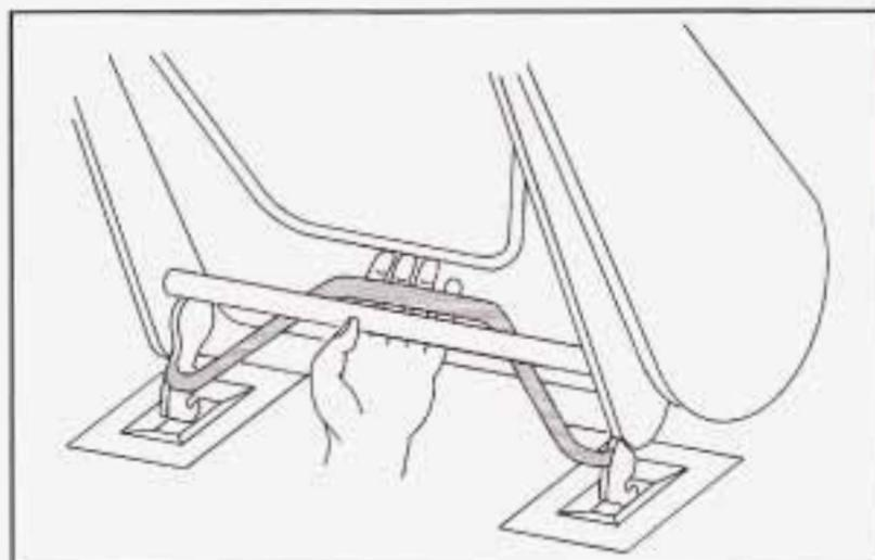
3. To unlatch the front latches, squeeze the angled bar toward the straight crossbar.
