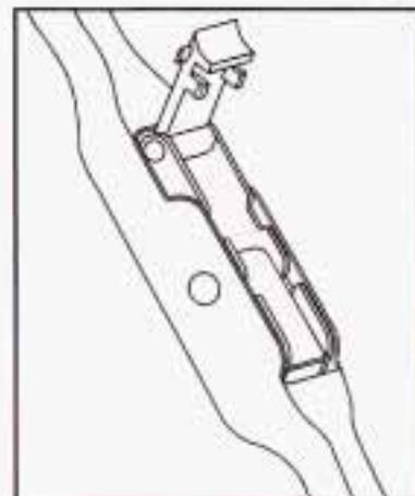
4. While holding the wiper arm away from the glass, push the release clip from under the blade.
