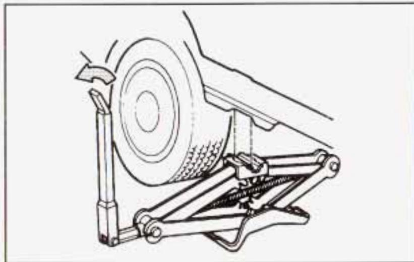
8. Lower the vehicle by attaching the folding wheel wrench to the jack and turning the wrench counterclockwise. Lower the jack completely.
