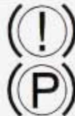
When your brake fluid falls to a low level, your brake warning light will come on. See *Brake System Warning Light* on page 3-44.
