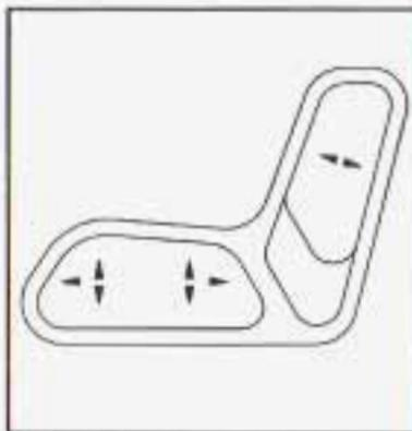
If your vehicle has this feature, the eight-way power seat controls are located on the outboard sides of both the driver's and the front passenger's seats.
