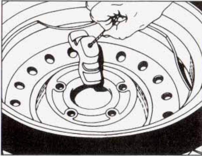
3. To remove the compact spare tire from the cable, tilt the retainer at the end of the cable so it can be pulled up through the wheel opening.
