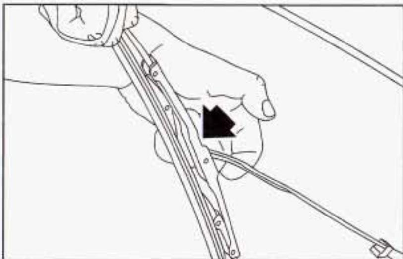
5. Push the release clip at the connecting point of the blade and the arm up. Then pull the blade assembly down toward the glass to remove it from the wiper arm.
