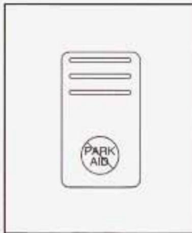
URPA can be turned off by pressing the rear park aid disable switch located in the instrument panel switchbank. When the system is disabled an indicator light will be lit on the switch. You will not see any lights on the rear display if the switch is in the off position.
