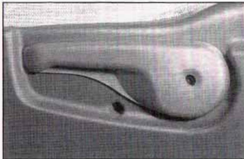
To adjust the manual seatback, pull up on the lever located on the outboard sides of both the driver's and the front passenger's seat. It is easier to recline the seat if you lean forward, taking your weight off the seatback.
