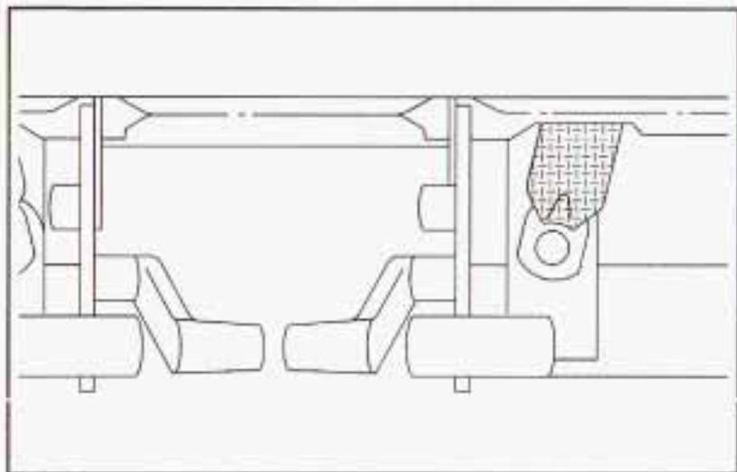
4. From behind the bench seat, push up the release handles at the base of the seat to release the latches from the floor pins.
