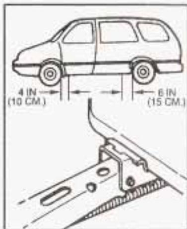
2. Near each wheel, there is a notch in the vehicle's body. Position the jack and raise the jack head until it fits firmly into the notch in the vehicle's frame nearest the flat tire.
