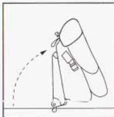
3. Release the rear set of hooks from the floor pins by pulling the nylon strap located at the base of the seat; hang on to the strap as the seat folds forward.
