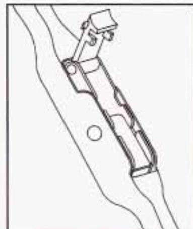
4. While holding the wiper arm away from the glass, push the release clip from under the blade.
