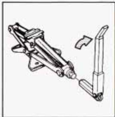
3. Attach the folding wrench to the jack, and turn the wrench clockwise to raise the jack head a few inches.
