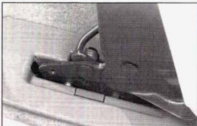
If the front latches are not attaching correctly, check that the seat is in the full rear position.
