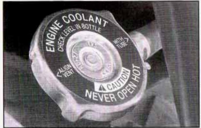
8. Then replace the pressure cap. At any time during this procedure if coolant begins to flow out of the filler neck, reinstall the pressure cap. Be sure the arrows on the pressure cap line up with the vent tube.
