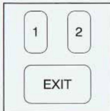
If your vehicle has this feature, the controls are located to the left of the steering column and are used to program and recall the driver's seat settings.
