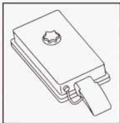
This fuse block is located in the engine compartment, in front of the windshield washer fluid reservoir. See *Engine Compartment Overview* on page 5-12 for more information on location.
