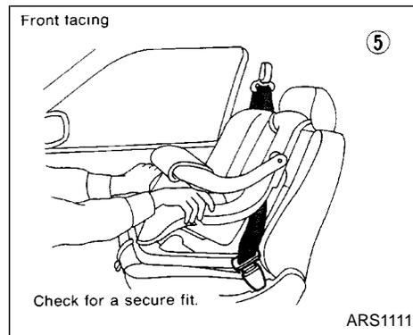
3. Pull on the shoulder belt until all of the belt is fully extended. At this time, the retractor is in the automatic locking mode (child restraint mode). It reverts back to emergency locking mode when the belt is fully retracted.
