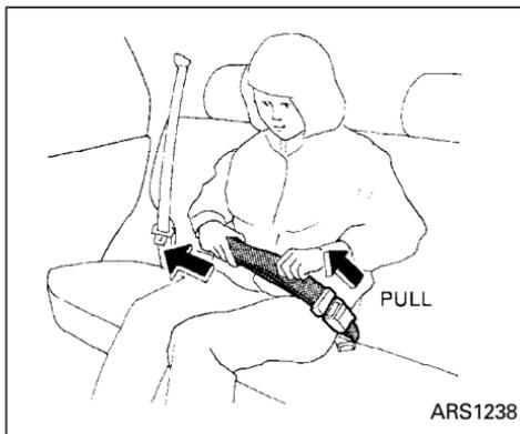
2. Tighten the belt by pulling the free end of the belt away from the tongue.
