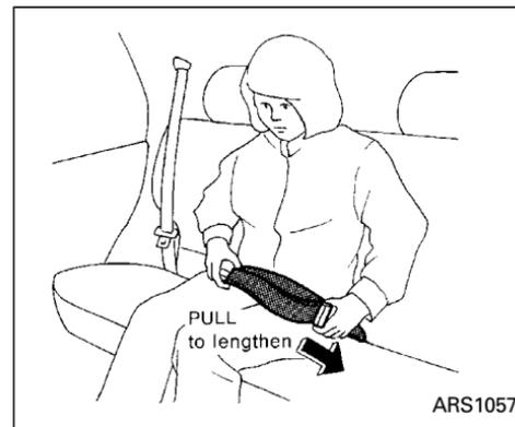
4. Loosen the belt by holding the tongue at a right angle to the belt, then pull on the belt.
