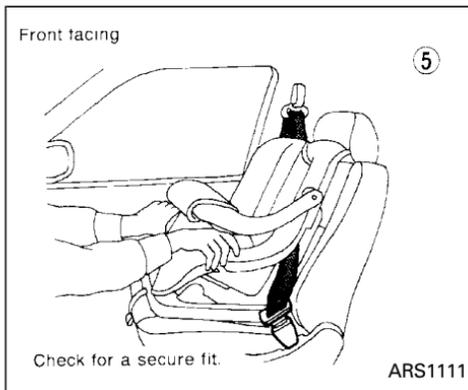
5. Before placing the child in the child restraint, use force to tilt the child restraint from side to side, and tug it forward to make sure it is securely held in place.
