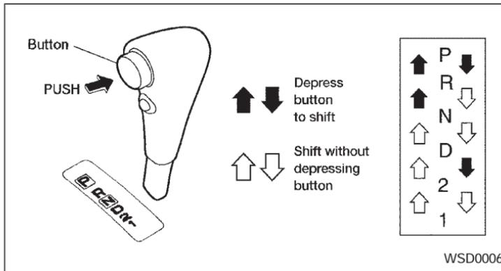
**The shift selector lever cannot be moved out of P (Park) and into any of the other gear positions if the ignition key is turned to LOCK or if the key is removed.**
