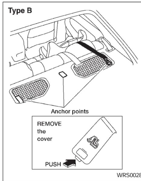
Remove the anchor cover from the anchor point which is located directly behind the child seat.
