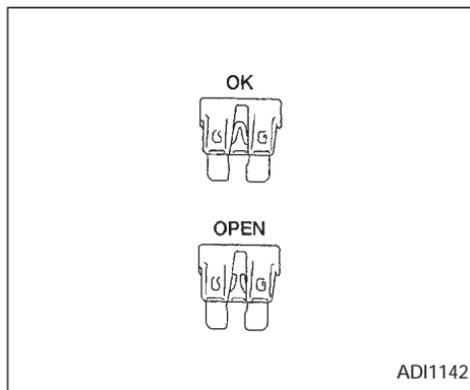
3. Remove the fuse with the fuse puller. The fuse puller is located in the center of the fuse block.
