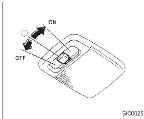
The interior light has a three-position switch.
