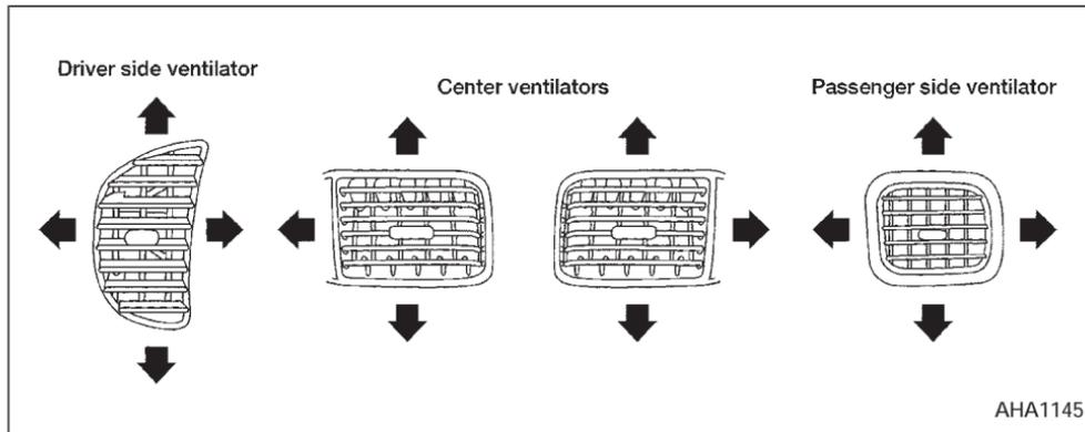
Adjust air flow direction by moving the ventilator slide.
