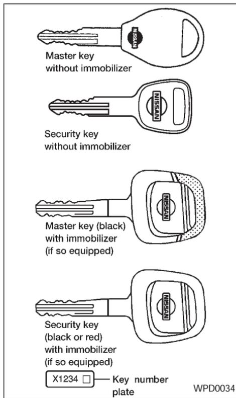
A key number plate is supplied with your keys. Record the key number and keep it in a safe place (such as your wallet), not in the vehicle. If you lose your keys, see an authorized NISSAN dealer for duplicates by using the key number. NISSAN does not record key numbers so it is very important to keep track of your key number plate.
