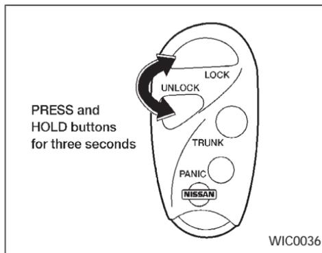
The hazard lights will flash once and the horn will sound once to confirm that the horn beep feature has been reactivated.
