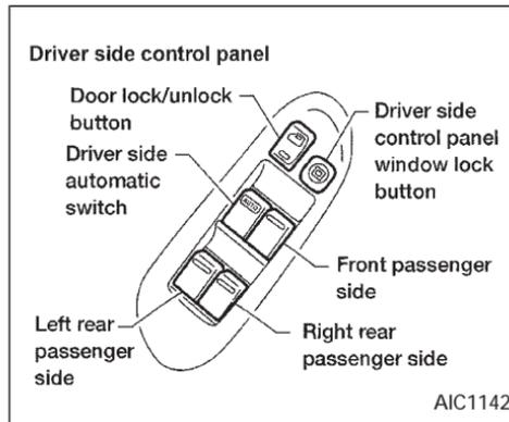
The power windows operate only when the ignition key is in the ON position.
