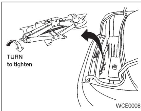
7. Install the jack in its storage area and tighten the jack screw clockwise.
