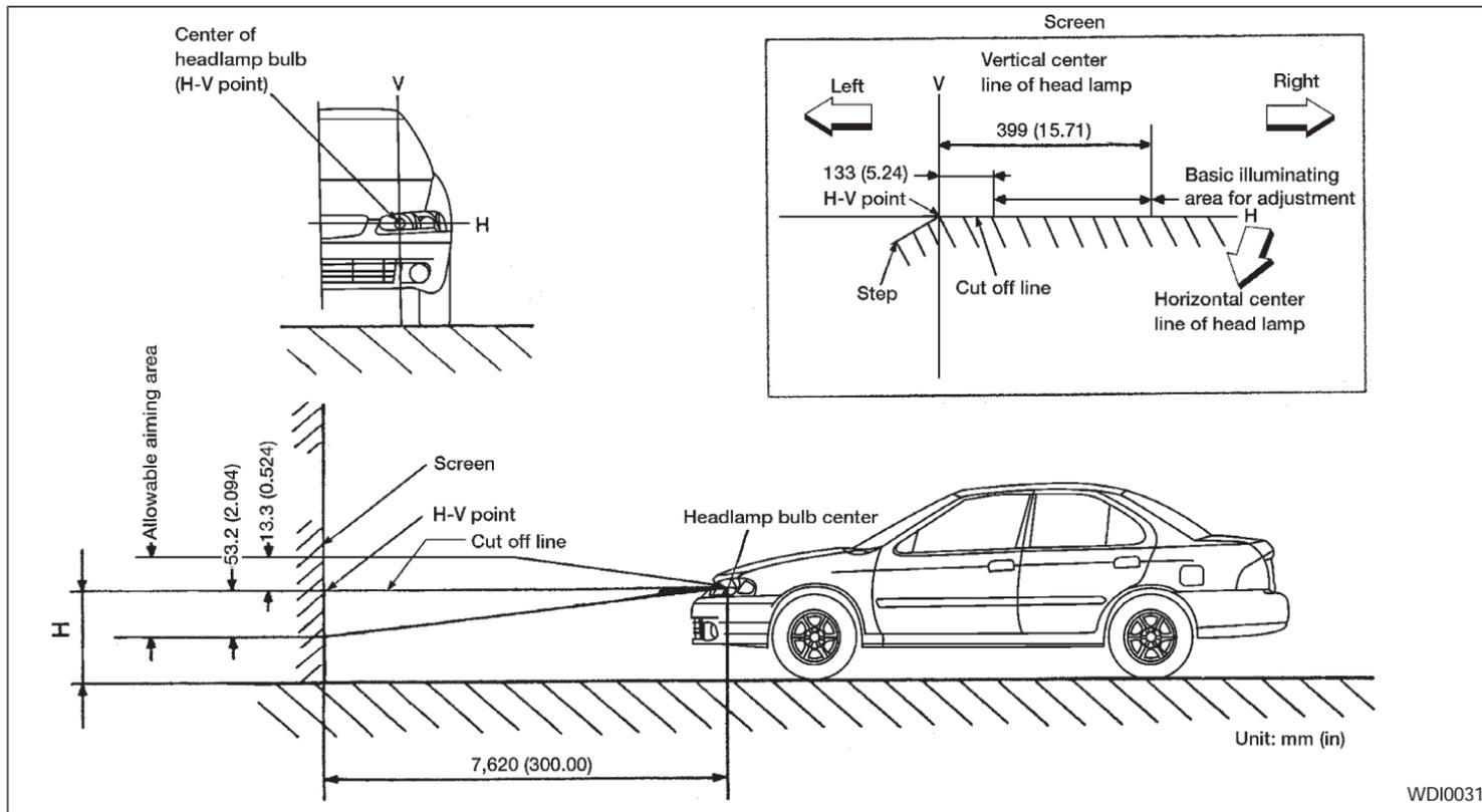
If the vehicle front body has been repaired and/or the headlight assembly has been replaced, check aiming. Use the aiming chart shown in the illustration.
