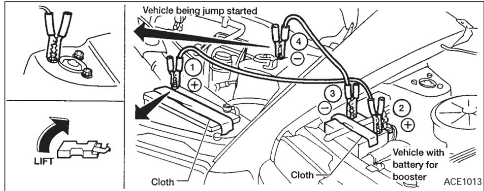
**Always follow the instructions below. Failure to do so could result in damage to the charging system and cause personal injury.**
