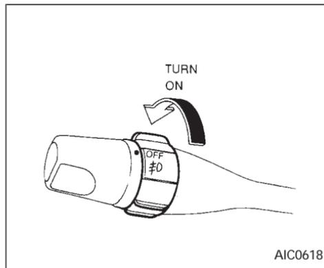
To turn the front fog lights on, rotate the switch to the
