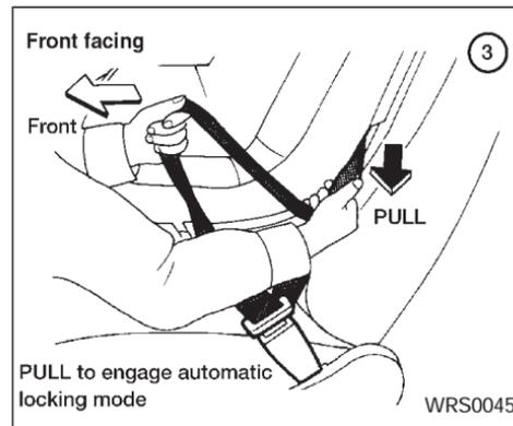
3. Pull on the shoulder belt until all of the belt is fully extended. At this time, the seat belt retractor is in the automatic locking mode (child restraint mode). It reverts back to emergency locking mode when the seat belt is fully retracted.
