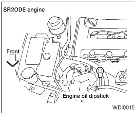
3. Turn off the engine. **Wait a few minutes for the oil to drain back into the oil pan.**
