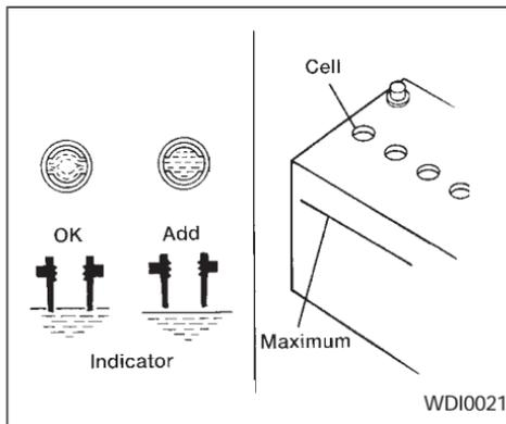
2. Check the fluid level in each cell.
