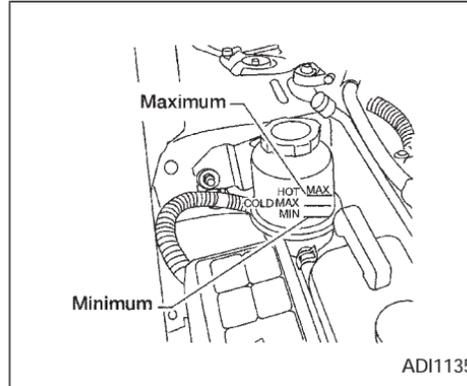
Check the fluid level in the reservoir.
