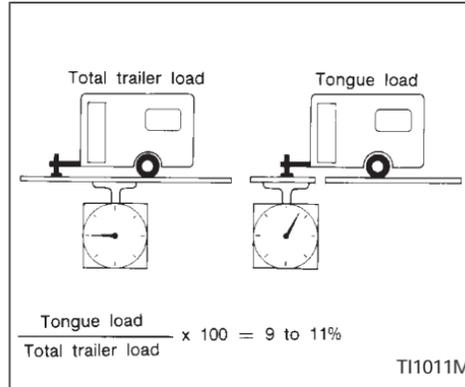
Your new vehicle was designed to be used primarily to carry passengers and cargo. Remember that towing a trailer places additional loads on your vehicle's engine, drive train, steering, braking and other systems.
