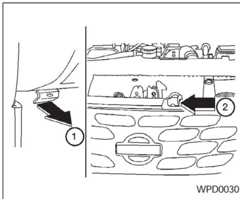
1. Pull the hood lock release handle ① located below the driver side instrument panel. The hood will spring up slightly.
