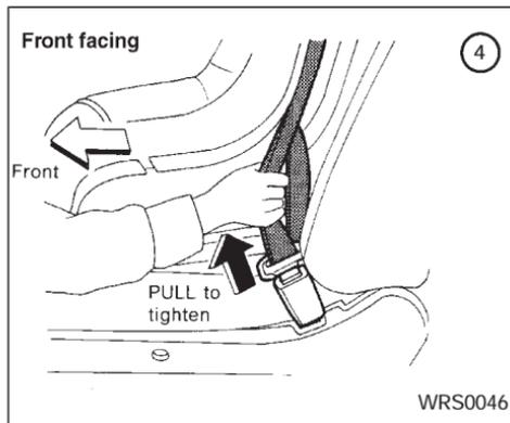
4. Allow the seat belt to retract slightly. Pull up on the seat belt to remove any slack in the belt.
