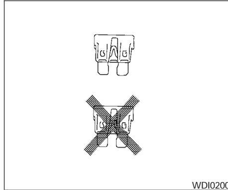
5. If the fuse is open, replace it with a new fuse.
