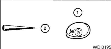
If you wax the surface of the hood, be careful not to let wax get into the washer nozzle ①. This may cause clogging or improper windshield washer operation. If wax gets into the nozzle, remove it with a needle or small pin ②.
