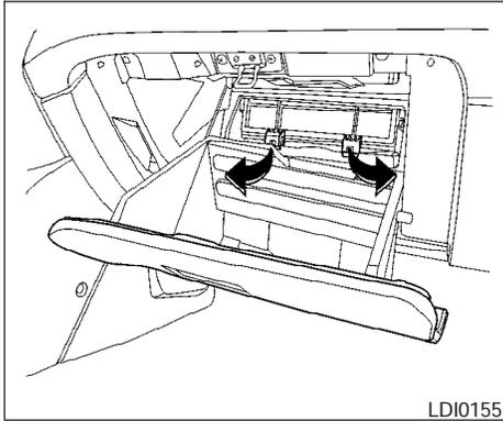
2. Remove the filter cover from the intake unit by disengaging the 2 hook tabs at the bottom of the cover.
