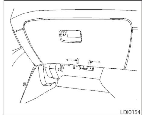
1. Remove the 2 lower glove box hinge pins. Remove the glove box from the opening and let it hang by the cord.
