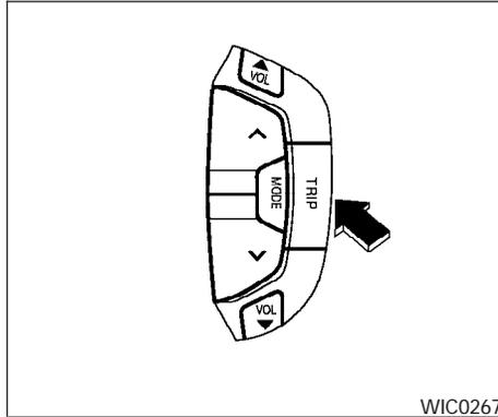
When the ignition switch is turned ON, modes of the trip computer can be selected by pushing the trip mode switch on the steering wheel switch for audio controls or by the trip computer change button. The following modes can be selected:
