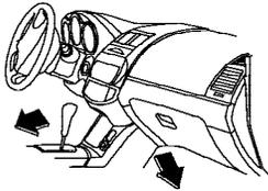
← : Air passed through heater core
