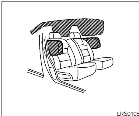
Supplemental side-impact air bag and curtain side-impact air bags system (if so equipped)
