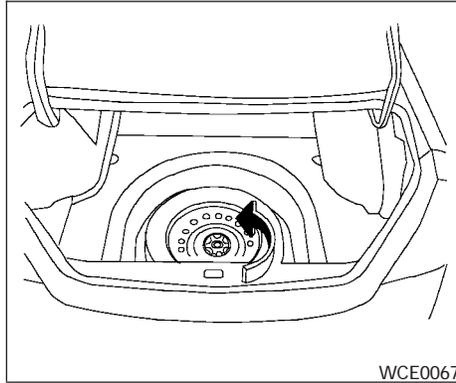
Removing the bolt-on wheel cover (if so equipped)
