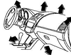
← : Air passed through heater core
