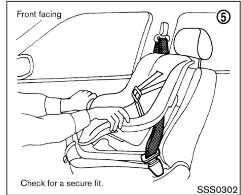
5. Before placing the child in the child restraint, use force to tilt the child restraint from side to side, and tug it forward to make sure that it is securely held in place. It should not move more than 1 inch (25 mm).
