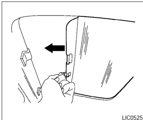
To close the skyview roof shade, pull the tab to draw out the shade. Lock the shade in place by positioning the rod on the holder.
