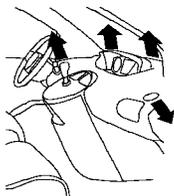
← Air passed through heater core
