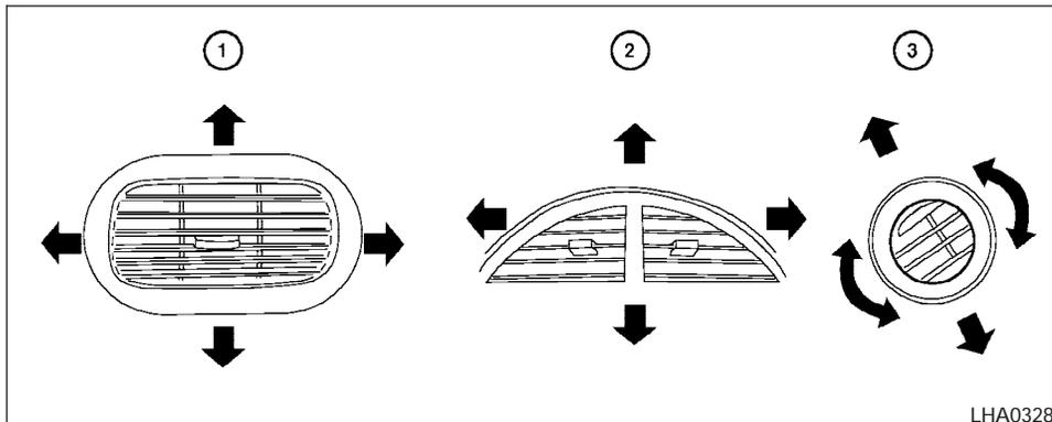
Adjust air flow direction for the driver and passenger side ①, center ②, and rear passenger side ③ ventilators by moving the ventilator slide and/or ventilator assemblies.
