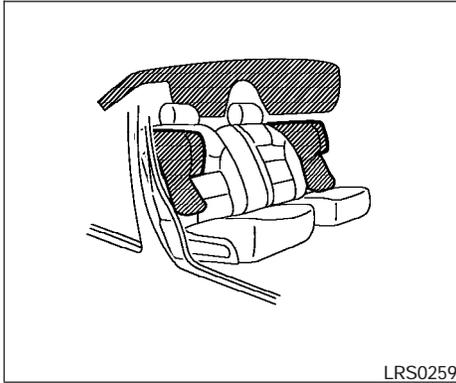
Supplemental side-impact air bag (if so equipped) and curtain side-impact air bag system
