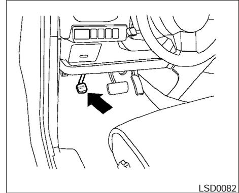
**To engage:** Firmly depress the parking brake.
