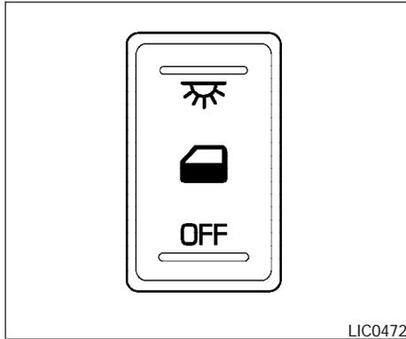
The lights on demand switch allows the driver to select one of three lighting modes for the room lights. The room lights are the map lights, personal lights and puddle lamps (if so equipped). The lights on demand switch operates regardless of ignition switch position.
