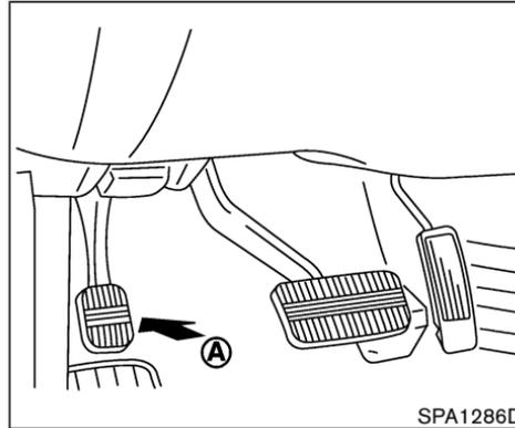
**To apply:** Fully depress the parking brake pedal
