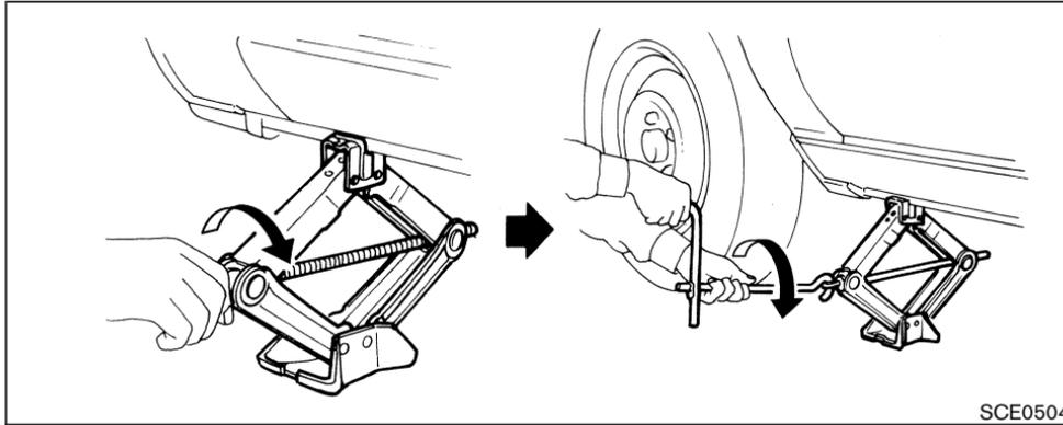
**The jack should be used on level firm ground.**
