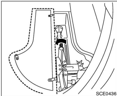
5. Securely store the flat tire and jacking equipment in the vehicle.
