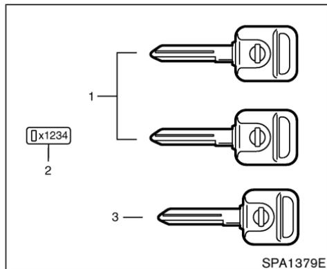
1. Master keys (with built-in transponder chip)
