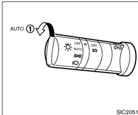
The autolight system can turn on the headlights automatically when it is dark, turn off the headlights when it is light, and keep the headlights on for up to 45 seconds after you turn the ignition switch to the OFF position and open any door then close all the doors. The headlight off time can be adjusted on the system setting display. See the “4. Display screen, heater, air conditioner and audio system” section.
