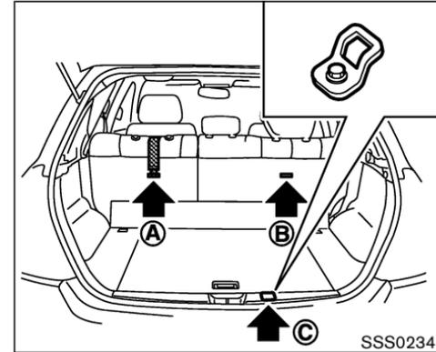
If your child restraint has a top tether strap, it must be secured to the anchor point provided behind its position.
