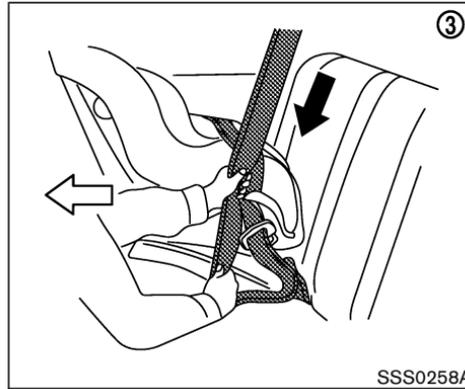
3. Pull on the shoulder belt until all of the belt is fully extended. At this time, the belt retractor is in the automatic locking mode (child restraint mode). It reverts back to emergency locking mode when the belt is fully retracted.
