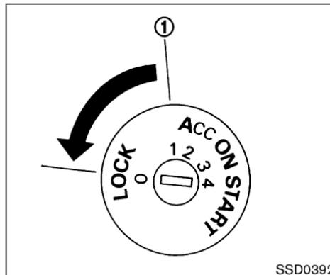
On CVT (Continuously Variable Transmission) models, the ignition lock is designed so that the key cannot be turned to LOCK and removed until the shift lever is moved to the P (Park) position.
