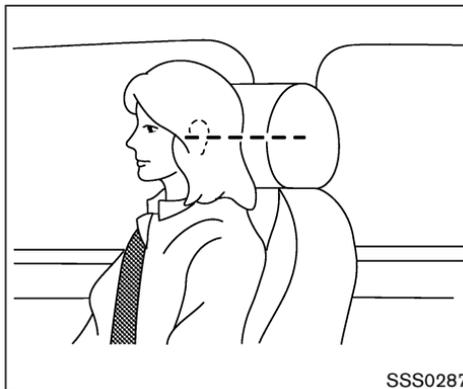
Adjust the head restraints as illustrated so the center is level with the center of your ears.
