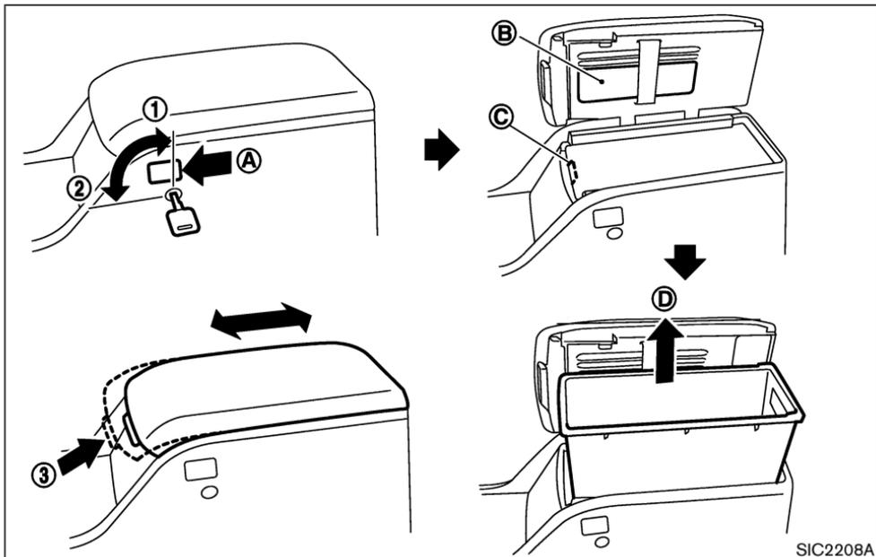
The inside of the console box lid is designed to be used as a holder **(B)** such as pen, etc. There is a power outlet **(C)** inside the console box.
