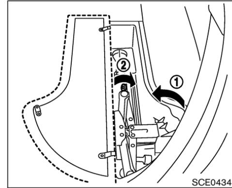
Pull up the floor cover ① as illustrated and remove ② the jack and tools.
