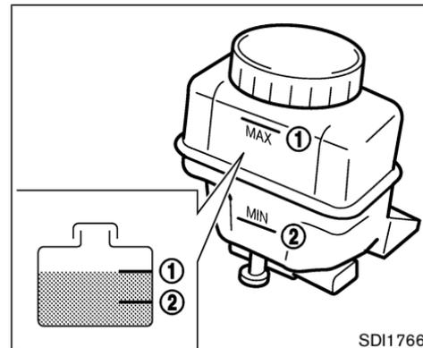
Check the fluid level in the reservoir. If the fluid is below the MIN line (2) or the brake warning light comes on, add Genuine NISSAN Super Heavy Duty Brake Fluid or equivalent **DOT 3** fluid up to the MAX line (1). If fluid must be added frequently, the system should be thoroughly checked by a NISSAN dealer.
