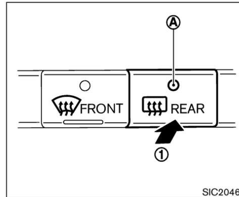
To defog/defrost the rear window glass and outside mirrors (if so equipped), start the engine and push the switch on ①. The indicator light (A) will come on. Push the switch again to turn the defroster off.
