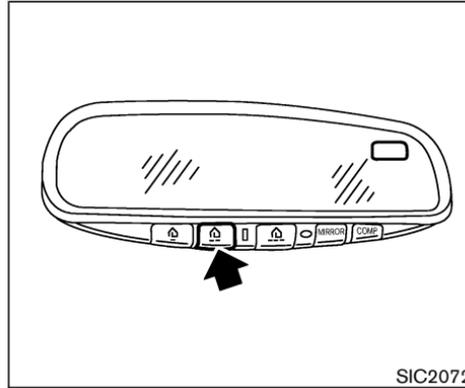
3. Using both hands, simultaneously push and hold both the HomeLink® button you want to program and the hand-held transmitter button. DO NOT release the buttons until step 4 has been completed.
