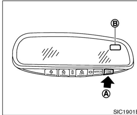
When the COMPASS switch **(A)** is pushed, the compass display **(B)** will indicate the direction the vehicle is heading.
