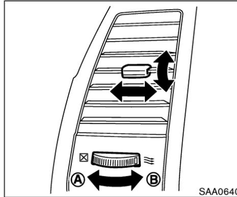
Open or close, and adjust the air flow direction of ventilators.
