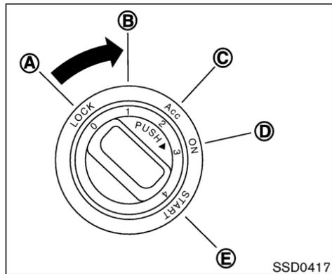
The ignition lock is designed so that the ignition switch cannot be turned to LOCK and removed until the shift lever is moved to the P (Park) position.
