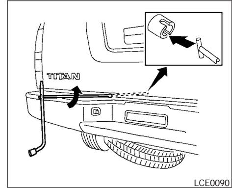
4. Fit the square end of the jack rod into the square hole of the wheel nut wrench to form a handle.
