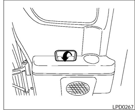
From the inside, pull the inside door handle toward you. The door will unlock automatically.
