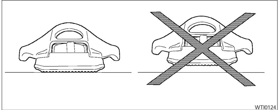
5. There should be no gap between the bottom of the cleat and the top of the channel. Tighten the center bolt hand tight (20-40 inch pounds).
