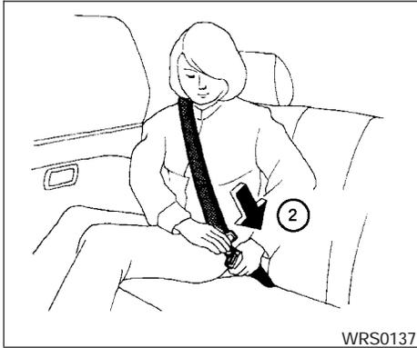
② Slowly pull the seat belt out of the retractor and insert the tongue into the buckle until you hear and feel the latch engage.
