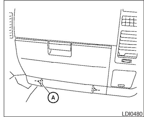
1. Remove the 2 lower glove box hinge pins
