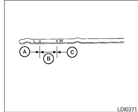
5. Remove the dipstick again and check the oil level. It should be between the H (High) and L (Low) marks (B). This is the normal operating oil level range. If the oil level is below the L (Low) mark (A), remove the oil filler cap and pour recommended oil through the opening. **Do not overfill (C).**
