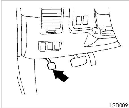
**To engage:** Firmly depress the parking brake.
