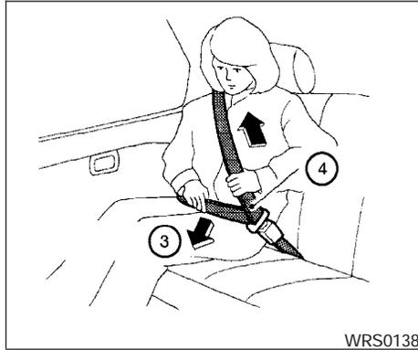
③ Position the lap belt portion **low and snug on the hips** as shown.
