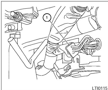
3. Locate the jumper harness connector under the lower portion of the instrument panel. The connector is taped to the wiring harness ① as indicated.
