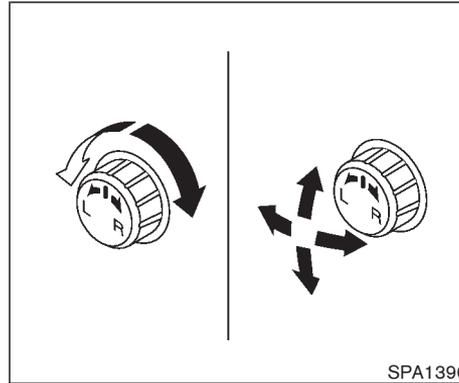
The outside mirror will operate only when the ignition switch is in the ACC or ON position.
