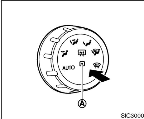
To defog/defrost the rear window glass and outside mirrors, start the engine and push the switch on. The indicator light (A) will come on. Push the switch again to turn the defroster off.
