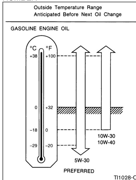
**SAE 5W-30 viscosity oil is preferred for all ambient temperatures. SAE 10W-30 or 10W-40 viscosity oil may be used if the ambient temperature is above 0°F (-18°C).**
