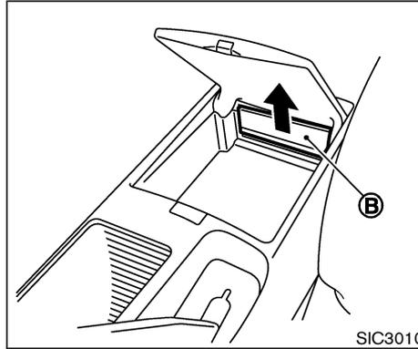
If objects (coins, etc.) fall into the rear section of the center console box, remove the rear wall ⑤ of the box as shown, and pick up the objects.
