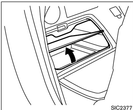
The rear floor box has another storage space under the bottom plate.
