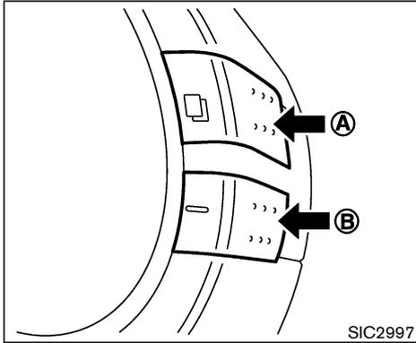
Switches for the trip computer are located on the side of the combination meter panel. To operate the trip computer, push the side of the switches as shown above.
