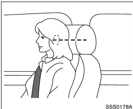
Adjust the head restraints so the center is level with the center of your ears.
