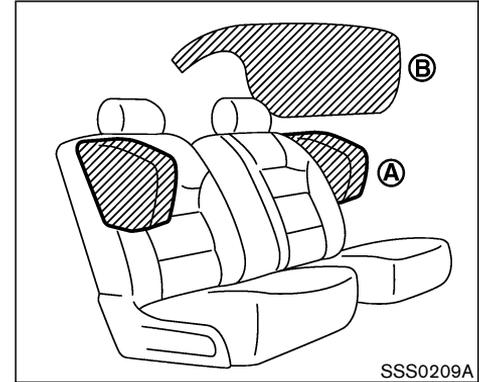
Supplemental side air bag and curtain side-impact air bag systems (if so equipped)
