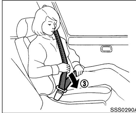
**belt and release it. Then smoothly pull the belt out of the retractor.**
