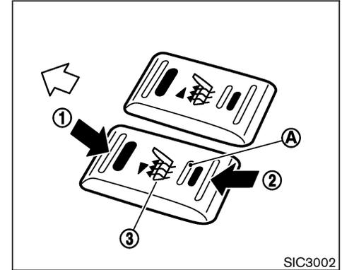
The seats are warmed by built-in heaters. The switches are located on the center console.
