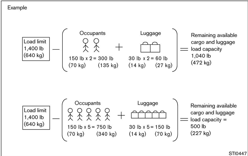
Steps for determining correct load limit
