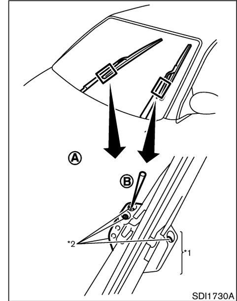
**If necessary, clean the windshield washer nozzle **(A)** with a needle or small pin **(B)**.**
