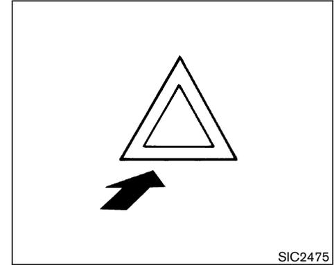
Push the switch (located on the front part of the center console) on to warn other drivers when you must stop or park under emergency conditions. All turn signal lights will flash.
