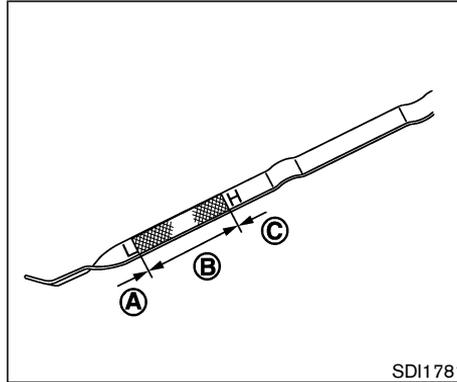
5. Remove the dipstick again and check the oil level. It should be between the H and L marks (B). If the oil level is below the L mark (A), remove the oil filler cap and pour recommended oil through the opening. **Do not overfill (C).**
