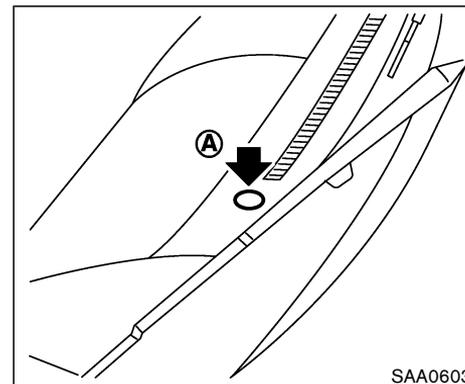
Sensor (A) on the instrument panel helps maintain a constant temperature; do not put anything on or around this sensor.
