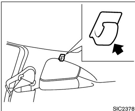
The hooks are located above the side windows as shown in the illustration.
