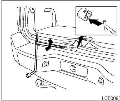
5. Fit the square end of the jack rod into the square hole of the wheel nut wrench to form a handle.
