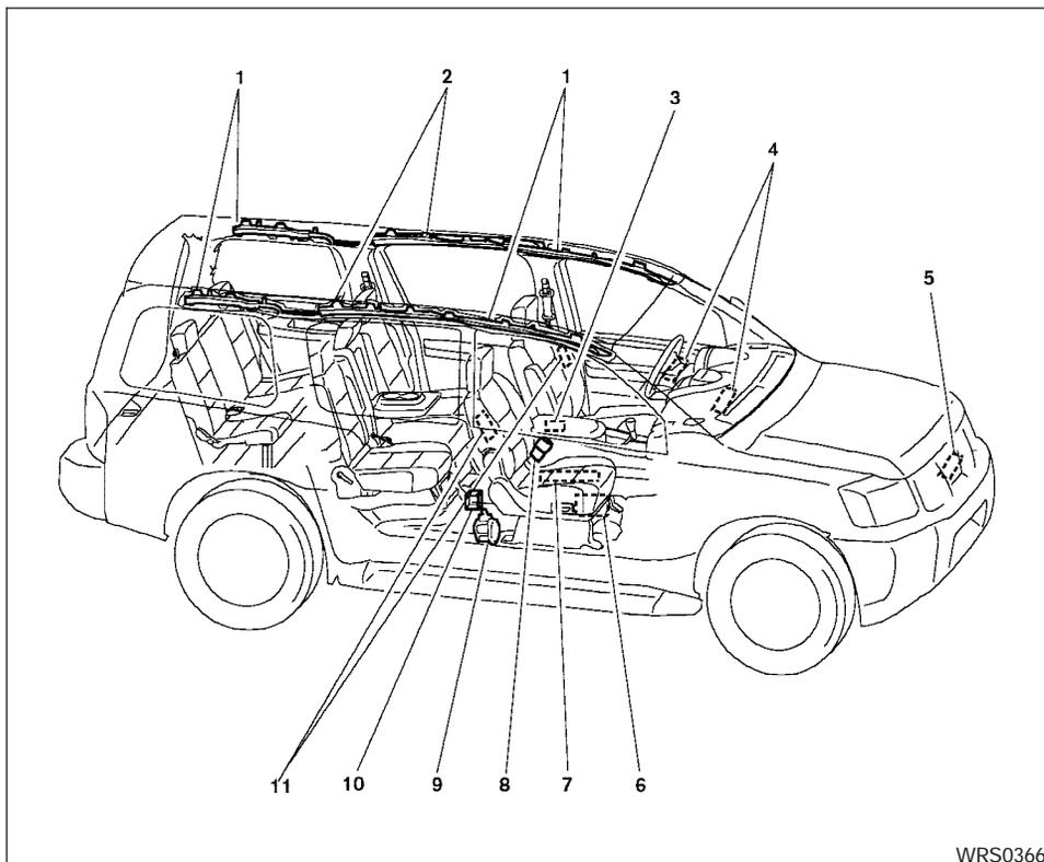
1. SRS curtain side-impact and rollover air bag modules
