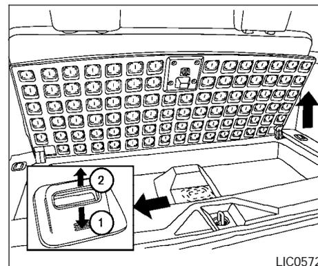
To access the floor storage area, push down ① to raise the handle, then pull up on the handle ② to lift the luggage board.
