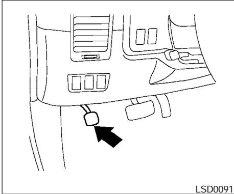
**To engage:** Firmly depress the parking brake.
