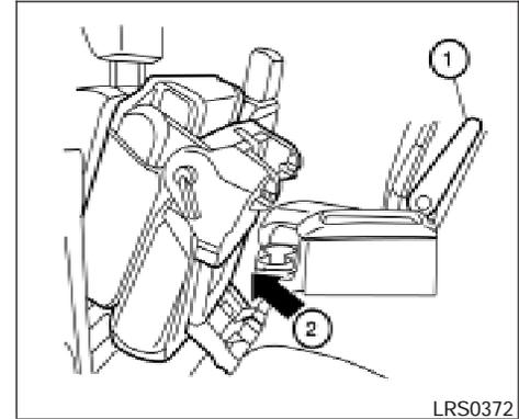
Then ② lift up on the lower corner of the seat base and tip the 2nd row captain's chair forward. To exit the 3rd row bench seat lift up on the same latch and fold the seatback forward onto the seat base. Then lift up on the seat base and tip it forward.
