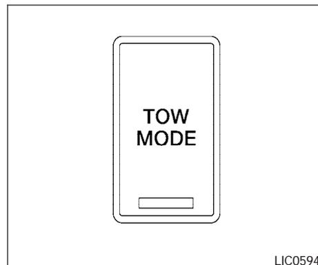
Tow mode should be used when pulling a heavy trailer or hauling a heavy load. Using tow mode at other times may cause unnecessary transmission shifting and reduced fuel economy.
