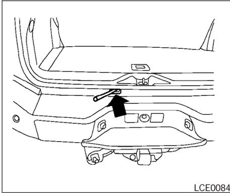
4. Assemble the two pieces of the jack rod. Find the oval-shaped opening above the middle of the license plate. Pass the T-shaped end of the jack rod through the opening and direct it toward the spare tire winch, located directly above the spare tire.
