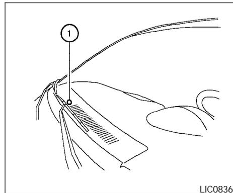
**Be sure you do not put anything on top of the autolight sensor ① located on top of the instrument panel. The autolight sensor controls the autolight; if it is covered, the autolight sensor reacts as if it is dark out and the headlights will illuminate. If this occurs while parked with the engine off and the key in the ON position, your vehicle’s battery could become discharged.**
