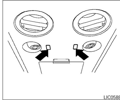
The personal lights on the overhead console can be swiveled 360 degrees. To turn on the light, press the button. Press the button again to turn off the light.
