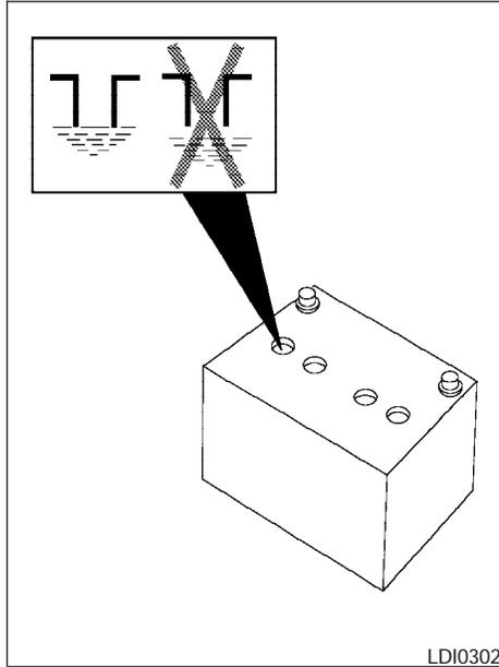
2. Check the fluid level in each cell. If it is necessary to add fluid, add only distilled water to bring the level up to the bottom of the filler opening. **Do not overfill.**
