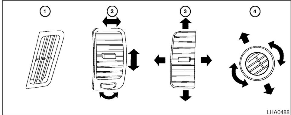
Adjust air flow direction for the driver and passenger side windows①, driver and passenger front ② center③, rear passenger compartment ④ and rear center console (if so equipped) ventilators⑤ by moving the ventilator slide and/or ventilator assemblies.
