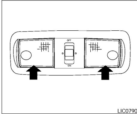
To turn the personal lights on, press the switches. To turn them off, press the switches again.
