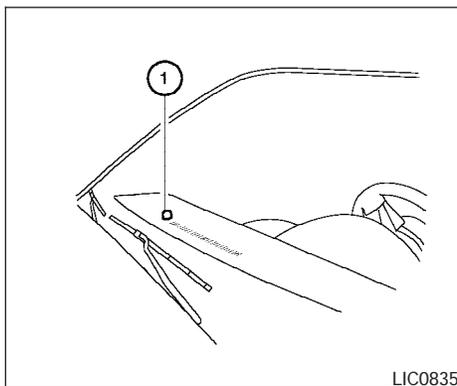
**Be sure you do not put anything on top of the autolight sensor ① located on the top side of the instrument panel. The autolight sensor controls the autolight; if it is covered, the autolight sensor reacts as if it is dark out and the headlights will illuminate. If this occurs while parked with the engine off and the key in the ON position, your vehicle's battery could become discharged.**
