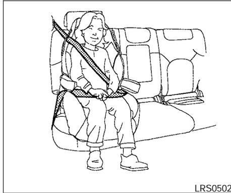
low back booster seat ① is chosen, the vehicle seat back must be at or above the center of the child's ears. If the seat back is lower than the center of the child's ears, a high back booster seat ② should be used.
