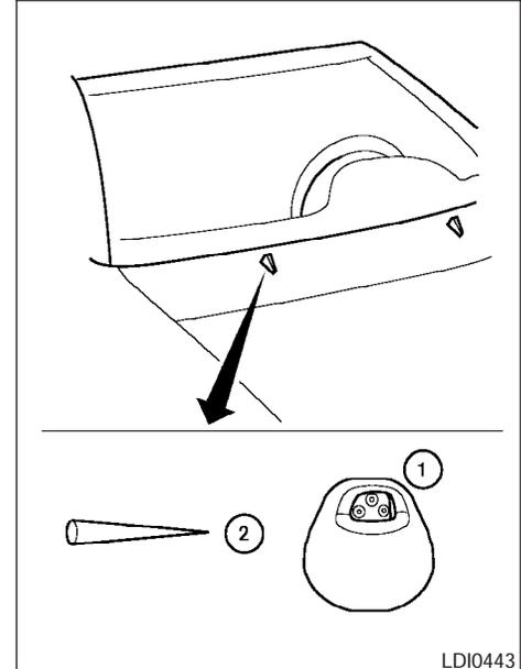
If you wax the surface of the hood, be careful not to let wax get into the washer nozzle ①. This may cause clogging or improper windshield washer operation. If wax gets into the nozzle, remove it with a needle or small pin ②.
