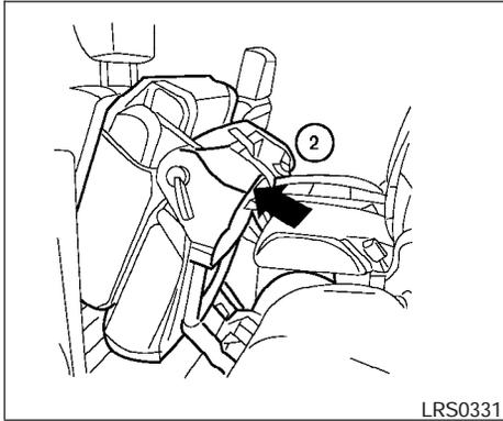
Then ② lift up on the lower corner of the seat base and tip the outboard seating position of the 2nd row bench seat forward. To exit the 3rd row bench seat lift up on the same latch and fold the seatback forward onto the seat base. Then lift up on the seat base and tip it forward.
