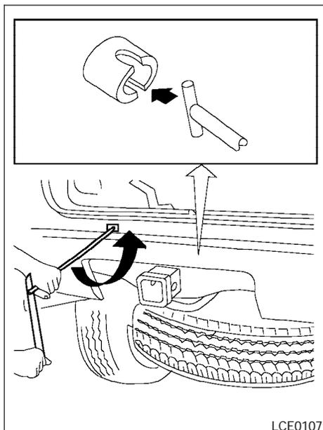
5. Fit the square end of the jack rod into the square hole of the wheel nut wrench to form a handle.
