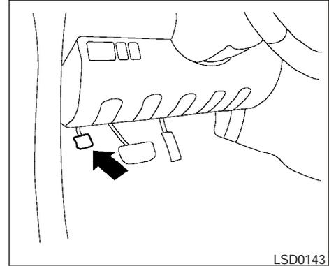
**To engage:** Firmly depress the parking brake.
