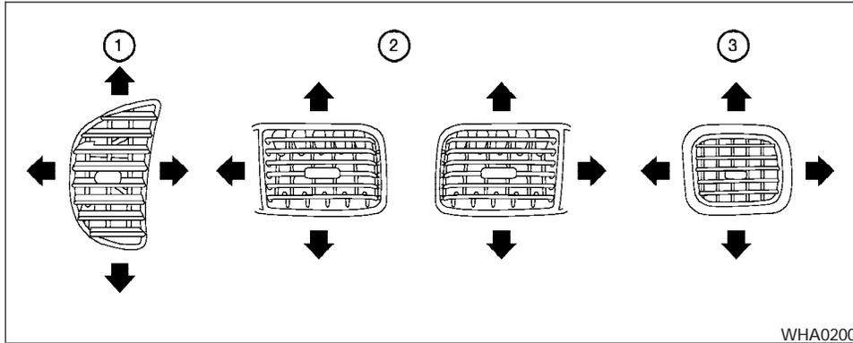
Adjust air flow direction for the driver's side ①, center ②, and passenger side ③ ventilators by moving the ventilator slide and/or ventilator assemblies.
