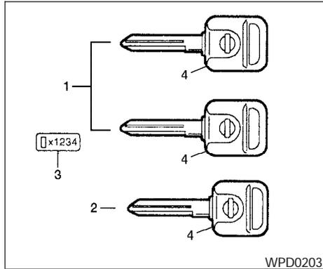
1. Two master keys (black) with transponder chip (if so equipped) and chrome NISSAN brand symbol on one side
