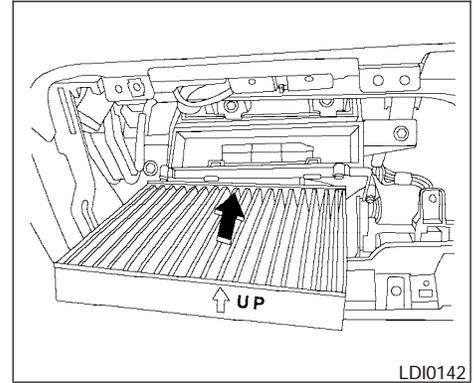
NOTE: The filter is marked "UP" with an arrow. The end of the filter with the arrow should face the rear of the vehicle.
