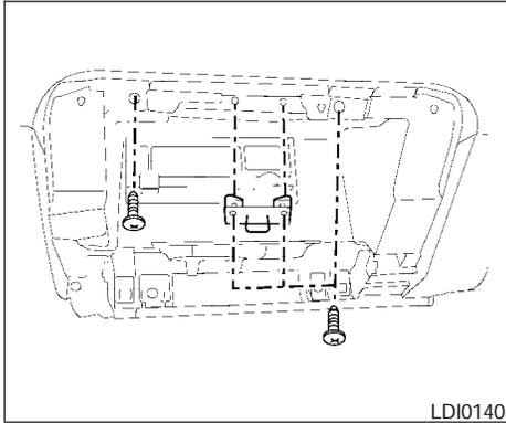
2. Remove the two screws securing the glove box frame.
