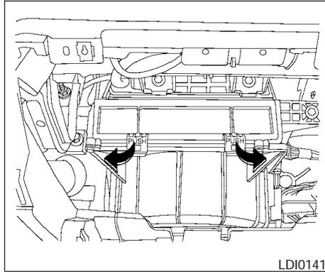
5. Remove the filter cover from the intake unit by disengaging the two hook tabs at the bottom of the cover. Remove the filter.
