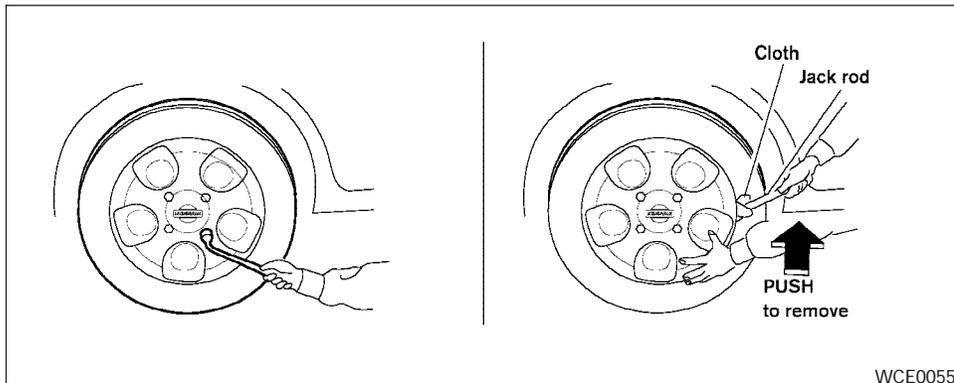
Removing bolt-on wheel cover (if so equipped)
