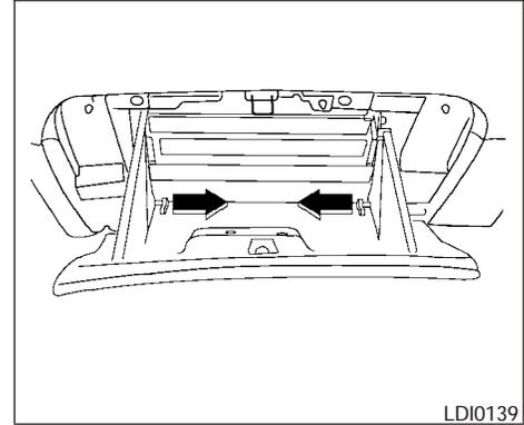
1. Remove the glove box door by removing the two lower hinge pins.
