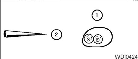
If you wax the surface of the hood, be careful not to let wax get into the washer nozzle ①. This may cause clogging or improper windshield washer operation. If wax gets into the nozzle, remove it with a needle or small pin ②.
