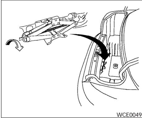
6. Install the jack in its storage area and tighten the jack screw clockwise.
