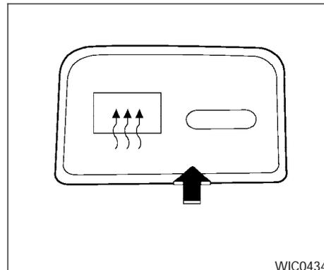
To defrost the rear window glass, start the engine and push the rear window defroster switch on. The rear window defroster indicator light on the switch comes on. Push the switch again to turn the defroster off.
