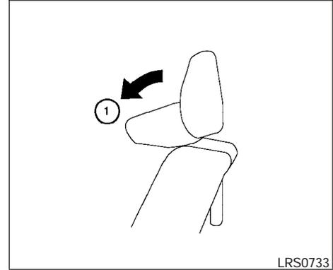
2. Fold down the rear head restraint. Pull the head restraint down and rotate to the lower position ①.
