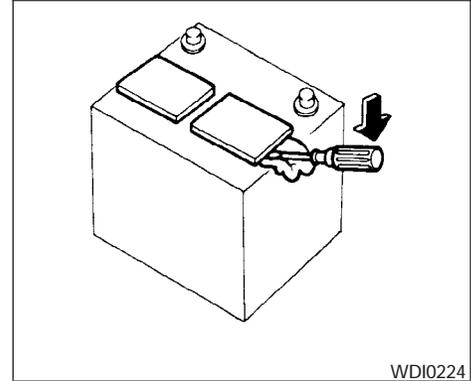
1. Remove the battery caps with a screwdriver as shown. Use a cloth to protect the battery case.
