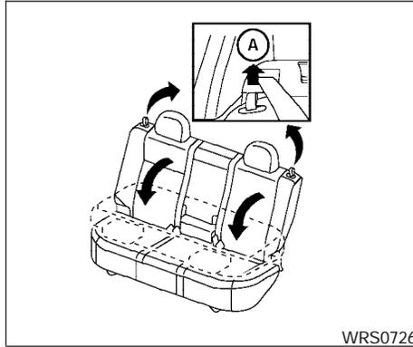
2. Pull up on the strap **A** located on the top outboard side of the seat to be folded.
