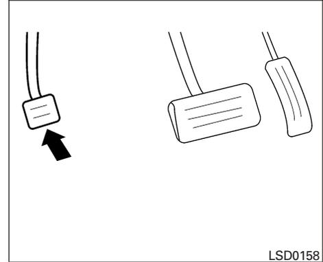
**To engage:** Firmly depress the parking brake.
