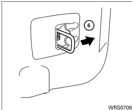
6. The rear seat anchors are spring loaded and can be folded into the side panels to maximize cargo space. The anchors are held in the folded position by the items in the cargo area. When the load is removed from the cargo area, the rear seat anchors automatically return to the unfolded position.
