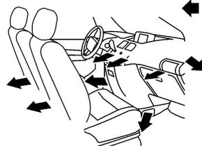
←:Air passed through heater core
