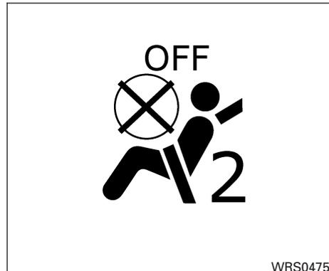
7. If the booster seat is installed in the front passenger seat, turn the ignition switch to the ON position. The front passenger air bag status light
