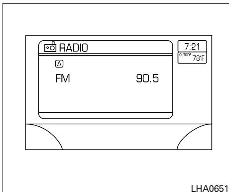
Any time audio information is shown on the main part of the screen, HVAC information will be displayed on the lower part of the screen. HVAC information will be shown even if "Audio" is selected to be displayed on the lower part of the screen.
