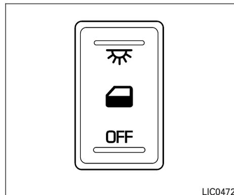
The lights on demand switch allows the driver to select one of three lighting modes for the interior lights. The lights on demand switch operates regardless of ignition switch position.
