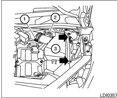
The air cleaner filter should not be cleaned and reused. Replace it according to the maintenance log shown in the “NISSAN Service and Maintenance Guide.” When replacing the filter, wipe the inside of the air cleaner filter housing and the cover with a damp cloth.
