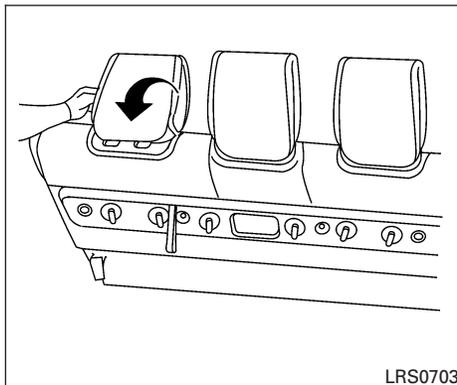
7. Reverse this process to return the bench seat to a seating position. **Make sure to properly return the head restraints to the upright position, push the bench seat down into the floor, and pull back on the seatback until they latch into place.**
