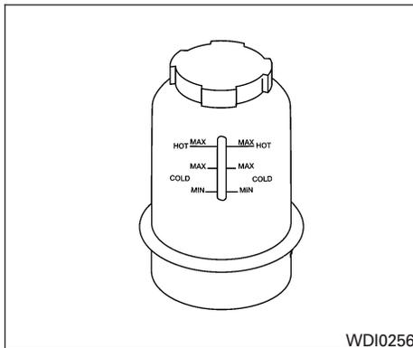
The fluid level should be checked using the HOT MAX range on the power steering fluid reservoir at fluid temperatures of 122° - 176°F (50° - 80°C) or using the COLD MAX range on the power steering fluid reservoir at fluid temperatures of 32° - 86°F (0° - 30°C).
