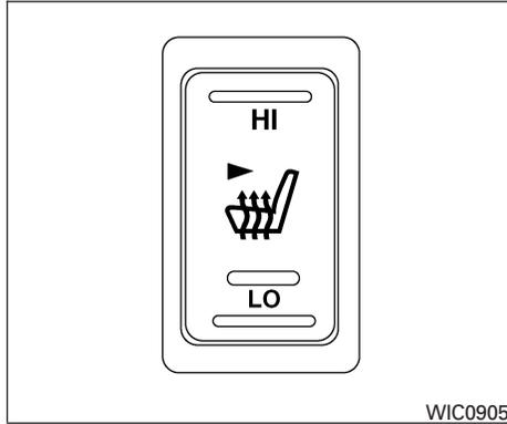
The front seats are warmed by built-in heaters (if so equipped). The switches are located at the sides of the seats.
