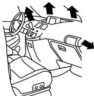
←:Air passed through heater core
