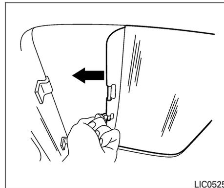
To close the SkyView roof sunshade, pull the tab to draw out the shade. Lock the shade in place by positioning the rod on the holder.
