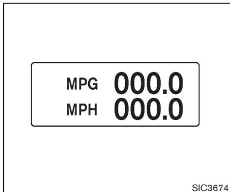
Average fuel consumption (MPG or l (liter)/100 km) and speed (MPH or km/h)
