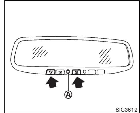
1. To begin, push and hold the 2 outer HomeLink® buttons (to clear the memory) until the indicator light (A) blinks (after 20 seconds). Release both buttons.
