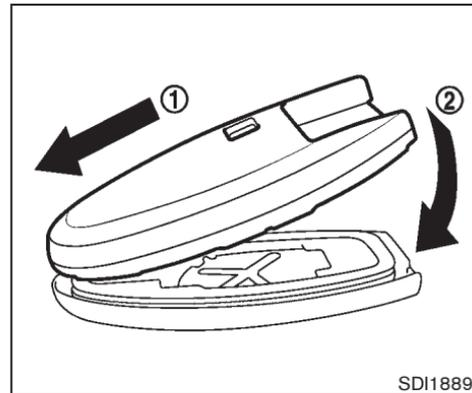
4. Align the tips of the upper and lower parts, and then push them together until it is securely closed.
