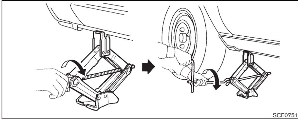
2. Loosen each wheel nut one or two turns by turning counterclockwise with the wheel nut wrench. **Do not remove the wheel nuts until the tire is off the ground.**
