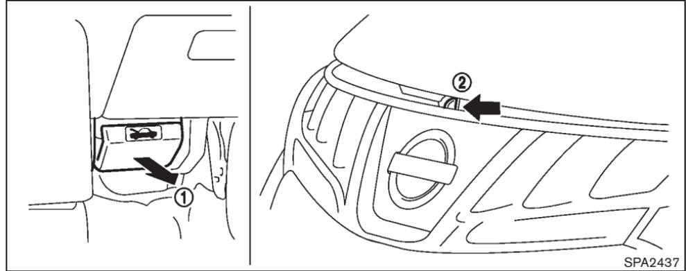
1. Pull the hood lock release handle ① located below the instrument panel; the hood will then spring up slightly.
