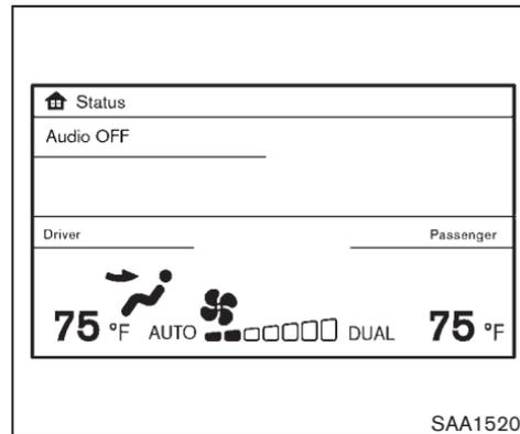
For the models with the color display screen, push the "STATUS" button to display the heater and air conditioner status screen. (See "HOW TO USE STATUS BUTTON" earlier in this section.)
