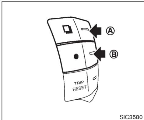
Current fuel consumption → Average fuel consumption and speed → Elapsed time and trip odometer → Distance to empty (dte) → Outside air temperature (ICY) → Setting → Warning check
