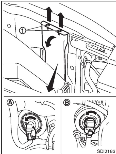
Disconnect the battery negative cable before replacing bulbs.
