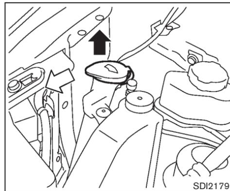
Fill the window washer fluid reservoir periodically. Add window washer fluid when the low window washer fluid warning light illuminates.
