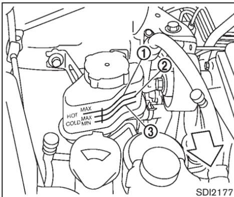
Check the fluid level in the reservoir.
