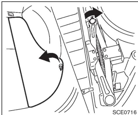
6. Remove the jacking tools and the spare tire.
