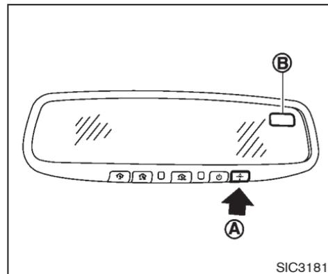
When the ignition switch is pushed to the ON position, the compass display (B) will indicate the direction of the vehicle’s heading.
