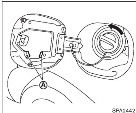
The fuel-filler cap is a ratcheting type. Turn the cap counterclockwise to remove. To tighten, turn the cap clockwise until ratcheting clicks are heard.
