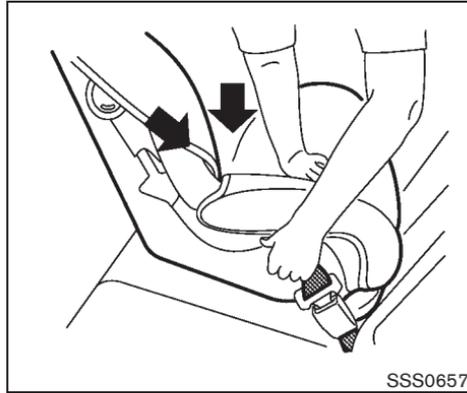
5. Remove any additional slack from the child restraint; press downward and rearward firmly in the center of the child restraint with your hand to compress the vehicle seat cushion and seatback while pulling up on the seat belt.
