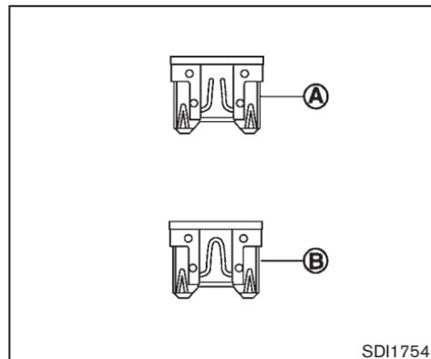
5. If the fuse is open (A), replace it with a new fuse (B). Spare fuses are stored in the passenger compartment fuse box.
