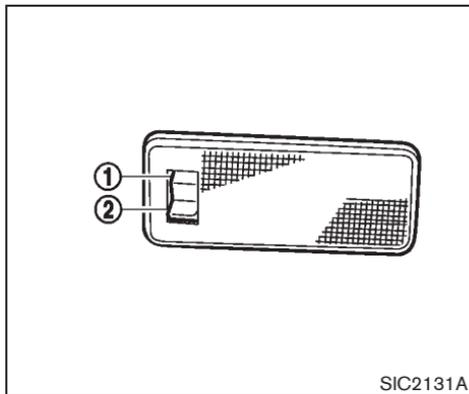
When the switch is in the ON position ①, the light illuminates while the lift gate is opened. When the lift gate is closed, the light will turn off.
