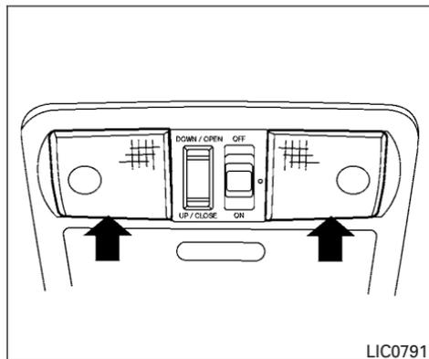
To turn the map lights on, press the switches. To turn them off, press the switches again.
