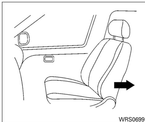
1. **If you must install a booster seat in the front seat, move the seat to the rear-most position.**
