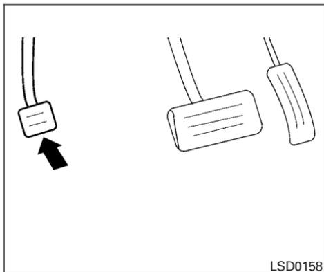
**To engage:** Firmly depress the parking brake.
