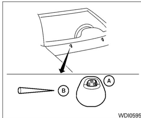
If you wax the surface of the hood, be careful not to let wax get into the windshield washer nozzle (A). This may cause clogging or improper windshield washer operation. If wax gets into the nozzle, remove it with a needle or small pin (B).
