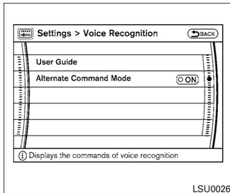
4. Highlight the “Alternate Command Mode” key and press the **ENTER** button.
