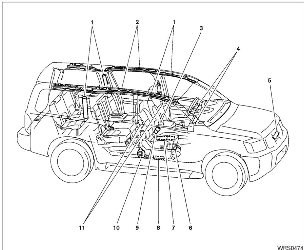
1. Roof-mounted curtain side-impact and rollover supplemental air bag inflators
