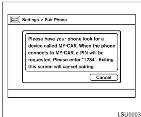
3. When a PIN code appears on the screen, operate the Bluetooth® cellular phone to enter the PIN code.
