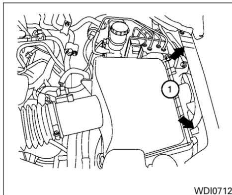
The air cleaner filter should not be cleaned and reused. Replace it according to the maintenance log shown in the "NISSAN Service and Maintenance Guide."
