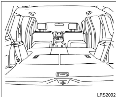
5. The carpet panel flap provides a level cargo floor when the 3rd row seats are also folded flat.
