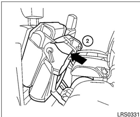
Then ② lift up on the lower corner of the seat base and tip the outboard seating position of the 2nd row bench seat forward. To exit the 3rd row bench seat, lift up on the same seatback latch and fold the seatback forward onto the seat base. Then lift up on the seat base and tip it forward.
