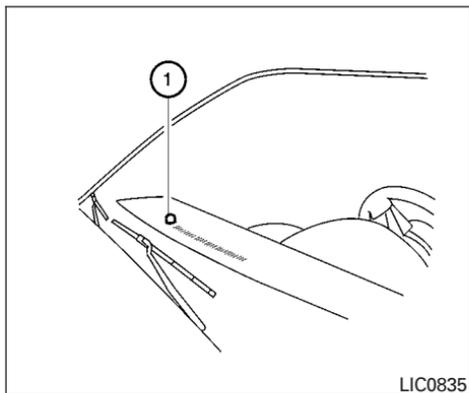
**Be sure you do not put anything on top of the autolight sensor ① located on the top side of the instrument panel. The autolight sensor controls the autolight; if it is covered, the autolight sensor reacts as if it is dark out and the headlights will illuminate. If this occurs while parked with the engine off and the ignition switch placed in the ON position, your vehicle's battery could become discharged.**
