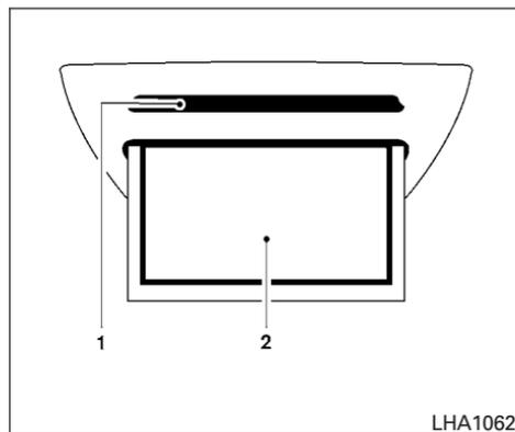
1. Infrared transmitter lens\*
