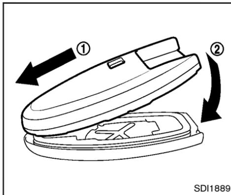
4. Align the tips of the upper and lower parts, and then push them together until it is securely closed.
