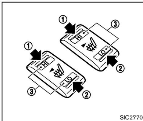
The seats are warmed by built-in heaters. The switches located on the instrument panel can be operated independently of each other.
