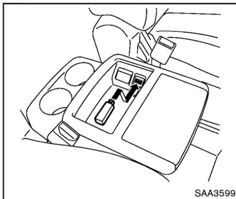
**USB MEMORY OPERATION (models with center multi-function control panel)****Audio main operation**
