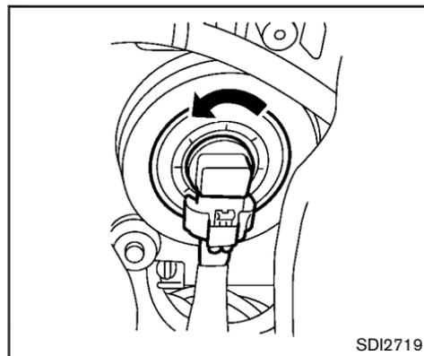
Disconnect the battery negative cable before replacing bulbs.
