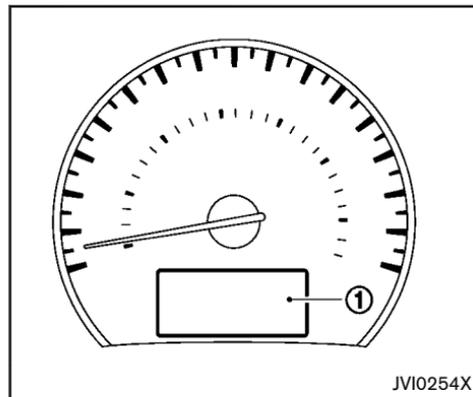
The dot matrix liquid crystal display  $\text{①}$  is located in the speedometer, and it displays, the key operation information and other warnings and information.
