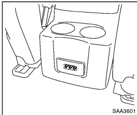
**AUXILIARY INPUT JACKS (if so equipped)**
