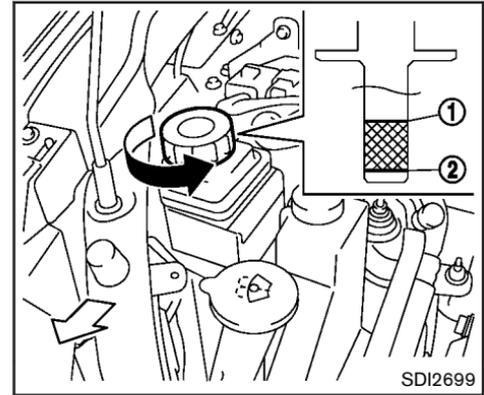
Check the fluid level in the reservoir.
