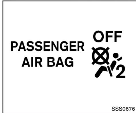
7. If the booster seat is installed in the front passenger seat, push the ignition switch to the ON position. The front passenger air bag status light
