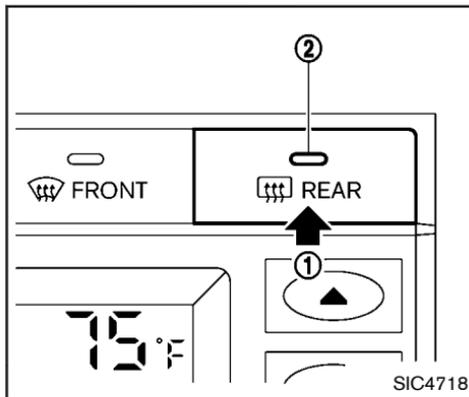
To defog/defrost the rear window glass and outside mirrors (if so equipped), start the engine and push the switch ① on. The indicator light ② will come on. Push the switch again to turn the defroster off.
