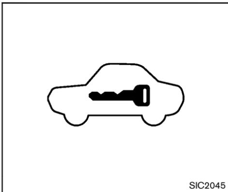
about 30 seconds the vehicle security system automatically shifts into the armed phase. The security light begins to flash once every approximately 3 seconds. If, during this 30-second pre-arm time period, the door is unlocked, or the ignition switch is pushed to ACC or ON, the system will not arm.
