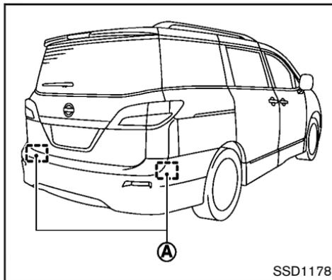
The BSW system uses radar sensors (A) installed near the rear bumper to detect other vehicles beside your vehicle in an adjacent lane.
