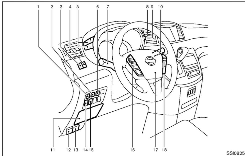
9. TRIP/RESET switch for twin trip odometer (P.2-6)
