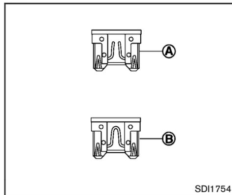
5. If the fuse is open ①, replace it with a new fuse ②. Spare fuses are stored in the passenger compartment fuse box.
