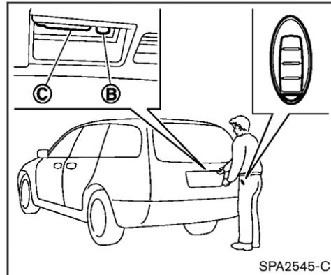
When you carry the Intelligent Key with you, you can lock or unlock all doors by pushing the door handle request switch **(A)** or the lift gate request switch **(B)** within the range of operation.
