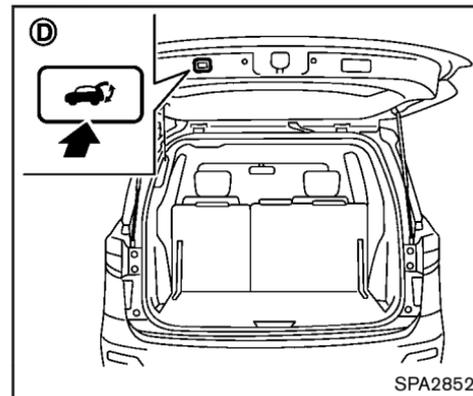
Power lift gate switch — Lift gate
