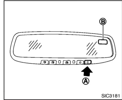
When the ignition switch is pushed to the ON position, the compass display
