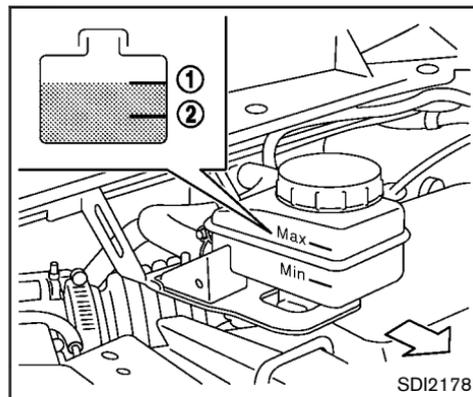
Check the fluid level in the reservoir. If the fluid is below the MIN line ② or the brake warning light comes on, add Genuine NISSAN Super Heavy Duty Brake Fluid or equivalent **DOT 3** fluid up to the MAX line ①. If fluid must be added frequently, the system should be checked by a NISSAN dealer.
