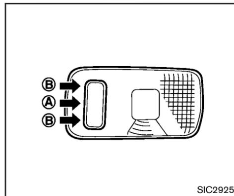
When the switch is in the DOOR position (A), the light illuminates while the lift gate is opened. When the lift gate is closed, the light will turn off.
