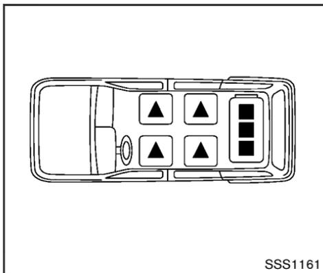
The illustration shows the seating positions equipped with adjustable headrests.
