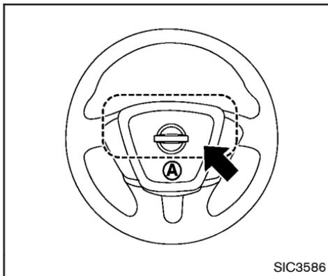
To sound the horn, push the pad area **A** of the steering wheel.
