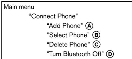
Use the Connect Phone commands to manage the phones connecting to the vehicle or to enable the Bluetooth® function on the vehicle.
