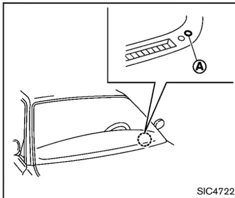
**Be sure not to put anything on top of the photo sensor **A** located on the top of the instrument panel. The photo sensor controls the autolight; if it is covered, the photo sensor reacts as if it is dark and the headlights will illuminate.**
