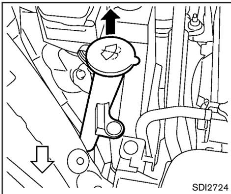
Fill the window washer fluid reservoir periodically. Add window washer fluid when the low washer fluid warning appears on the dot matrix liquid crystal display.
