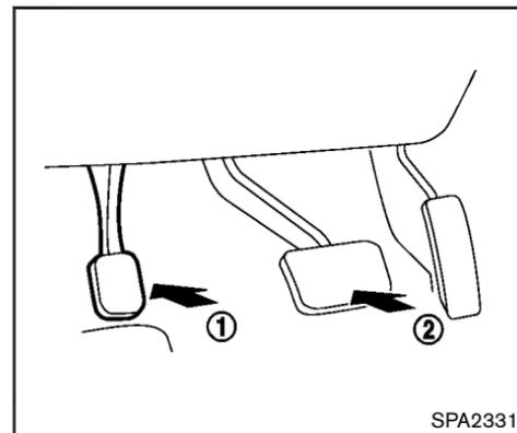
**To apply:** Fully depress the parking brake pedal (1).
