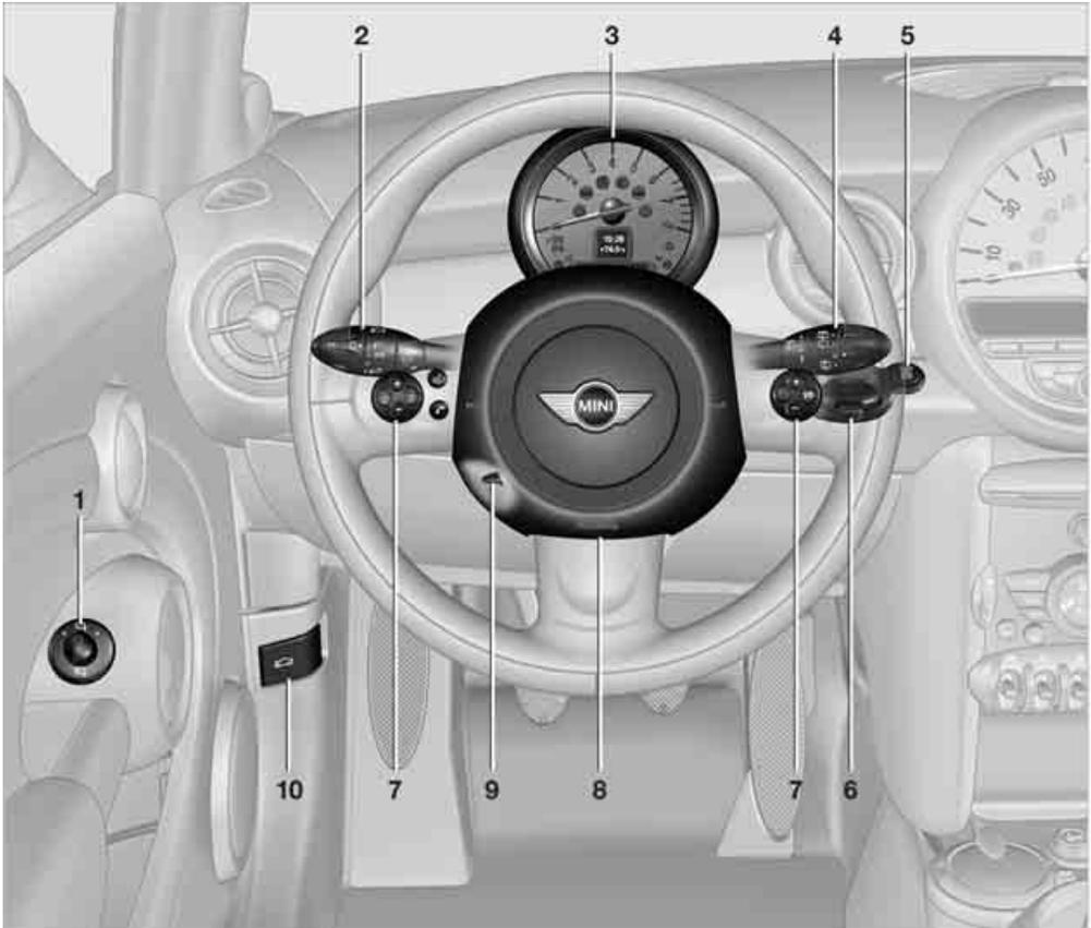
1 Adjusting the exterior mirrors, folding them in and out\* 33
