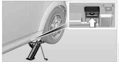
2. During jacking up, insert the jack head in the square recess of the jacking point.
