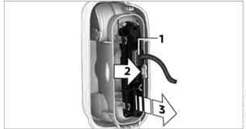
4. Screw out the respective bulb counterclockwise.
