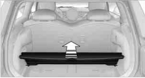
Raise the level load floor and fold it up toward the front, arrow.
