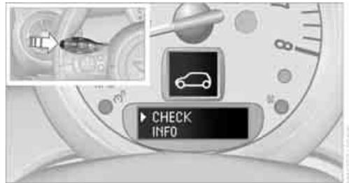
4. Hold the button down. "CHECK OK" appears if there are no Check Control messages. If a Check Control message has been stored, the corresponding message is displayed.
