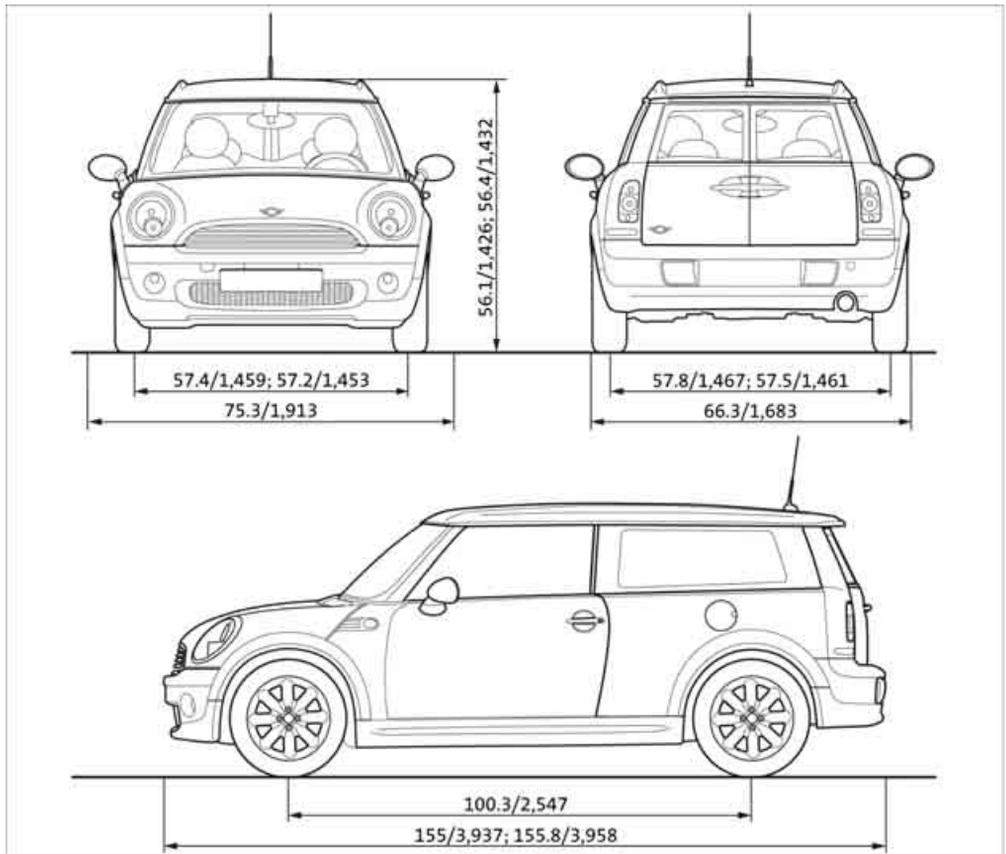
All dimensions given in inches/mm. Smallest turning circle diam.: 36 ft/11 m.
