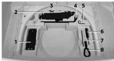
In vehicles with the space-saver spare tire, the tire change set with the onboard tool kit is located beneath the floor mat or level load floor in the cargo bay.
