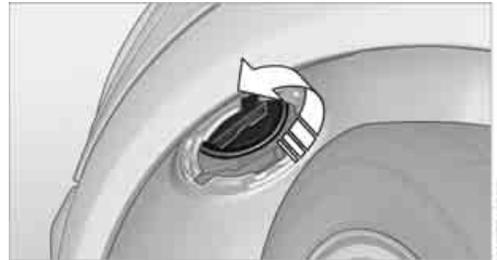
4. Screw out the bulb counterclockwise.
