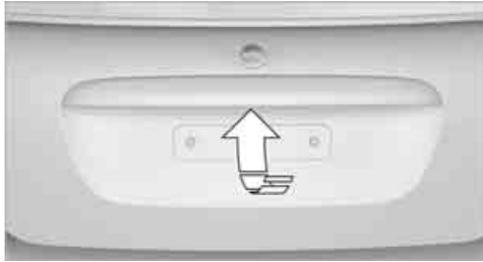
Press the button in the handle, arrow, or the
