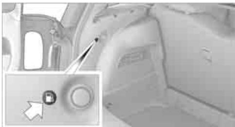
Pull on the green knob with the fuel pump symbol; the fuel filler door opens.
