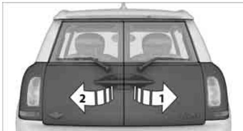
Press the button in the handle or the
