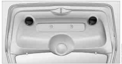
The handle recesses on the interior trim panel of the tailgate make it easier to pull it down.
