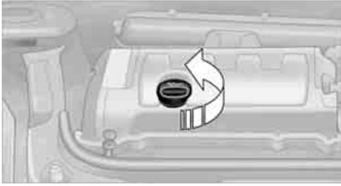
Do not add the maximum quantity of 1 US quart/1 liter of engine oil until the oil level has dropped to just above the lower mark on the dipstick, page 107.
