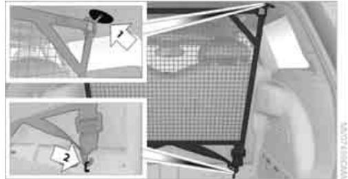
2. Insert each partition net mounting pin all the way into its respective rear mount in the headliner, arrow 1, and push it forward.
