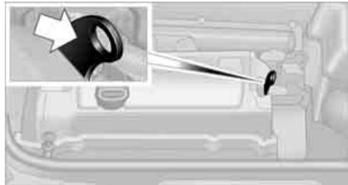
5. Attach the second terminal clamp of the minus/- jumper cable to the negative terminal of the battery or to the engine or body ground of the vehicle to be started.
