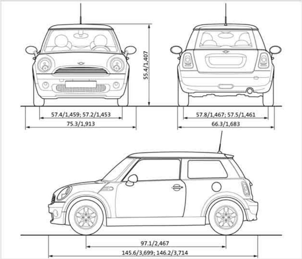
All dimensions given in inches/mm. Smallest turning circle diam.: 35 ft 2 in/10.7 m.
