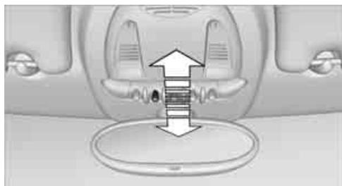
To switch the interior lamps on/off.
