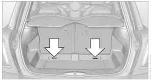
There are two additional anchors for child-restraint systems with tether straps, arrows. When the vehicle is equipped with a level load floor\*, the anchors are covered. Their positions are labeled.
