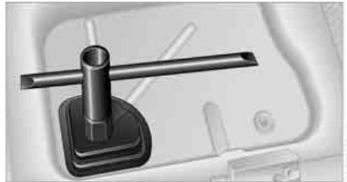
3. Screw the lifting handle from the onboard tool kit onto the thread.
