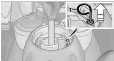
3. Take the hub cover remover 1 out of the onboard tool kit and insert it in the loop on the front passenger side.
