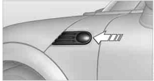
2. Screw out the bulb holder counterclockwise.
