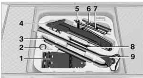
On vehicles with a space-saver spare tire, the tire change set with onboard tools is stored under the floor mat in the cargo bay.
