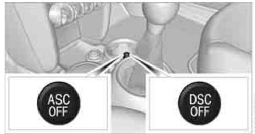
Press the button repeatedly until the indicator lamp for the ASC or DSC comes on. ASC or DSC are deactivated. Stabilizing and drive-output promoting actions are no longer executed.
