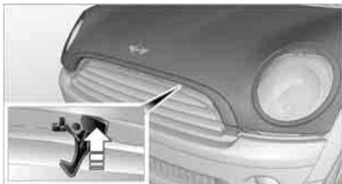
**⚠** To avoid damage, make sure that the wiper arms are against the windshield before you open the bonnet. ◀
