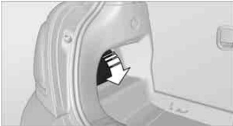
2. Screw out the desired bulb counterclockwise, arrows 1. Additional bulbs are located behind the sidewall of the cargo bay, arrow 2.
