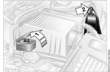
The illustration shows the auxiliary jump-starting terminal on the MINI COOPER S and the MINI COOPER S Convertible. In the MINI COOPER S and the MINI COOPER S Convertible, the auxiliary jump-starting terminal, arrow 1, acts as the positive battery terminal, refer to view of engine compartment on page 120. The cover is marked with a +.
