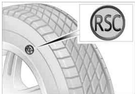
You will recognize Run-Flat Tires by a circular symbol containing the letters RSC on the side of the tire.
