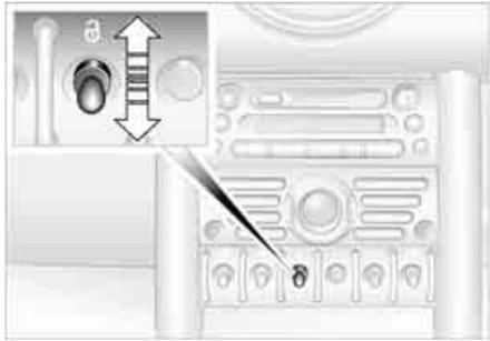
This switch locks or unlocks the doors and tailgate when the front doors are closed, but the anti-theft system is not activated. The fuel filler door remains unlocked.
