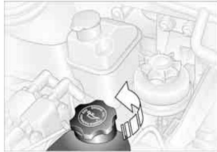
**!** Add oil within the next 30 miles/ 50 km, otherwise the engine could be damaged. ◀
