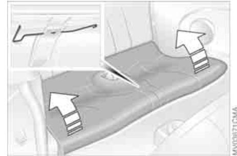
2. Fold the rear bench seat upward and remove the hook attached to it
