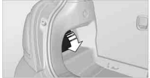
2. Pull on the green knob with the fuel pump symbol. The fuel filler door is released.
