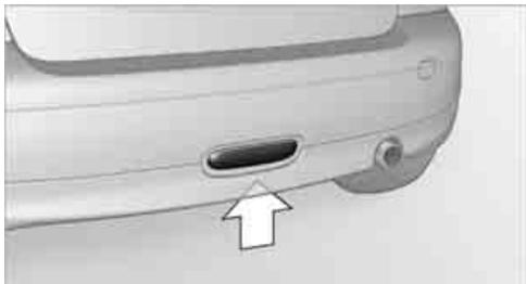
1. Screw out the bulb holder counterclockwise.
