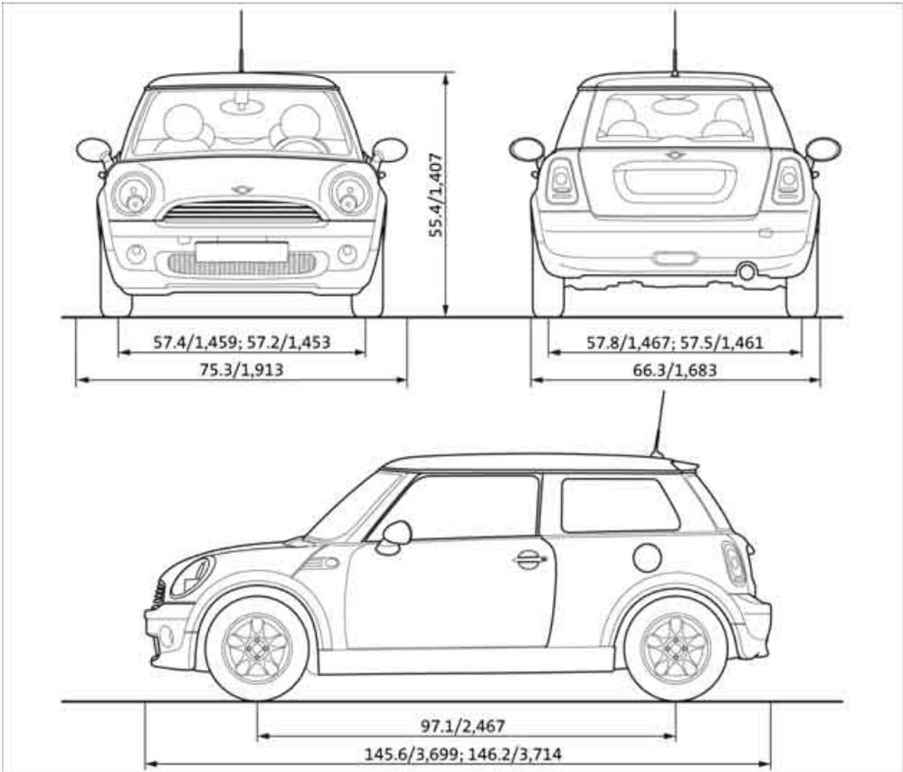
All dimensions given in inches/mm. Smallest turning circle diam.: 35 ft 10 in/10.7 m.
