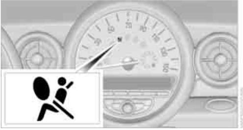
As of radio readiness, page 37, the warning lamp comes on briefly to indicate that the entire airbag system and the belt tensioners are operational.
