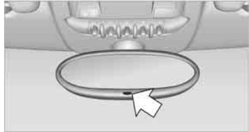
The automatic dimming feature of the interior rearview mirror\* is controlled by two photo cells in the mirror. One photo cell is in the mirror frame, arrow; the other is on the back of the mirror.
