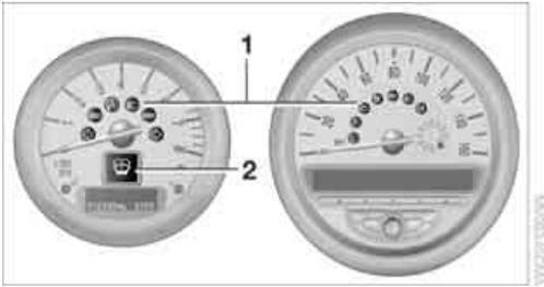
Indicator and warning lamps can light up in various combinations and colors in indicator area **1** or **2**. Some lamps are checked for proper functioning and thus come on briefly when the engine is started or the ignition is switched on.
