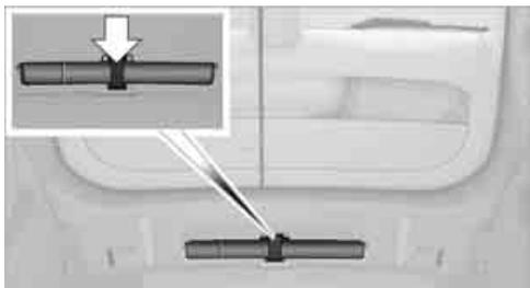
In the cargo area under the loading sill. Open the center lock to take it out.
