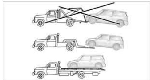
Have the MINI Clubman transported with a tow truck with a so-called lift bar or on a flat bed.
