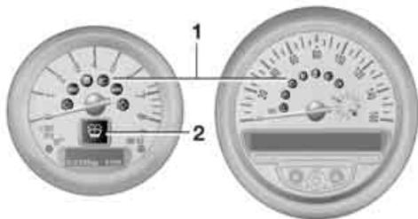
Indicator and warning lamps can light up in various combinations and colors in indicator area 1 or 2. See the table for information on causes and how to react. Note whether a lamp comes on alone or in combination with another. Some lamps can light up in different colors. Corresponding distinctions are made in the text.
