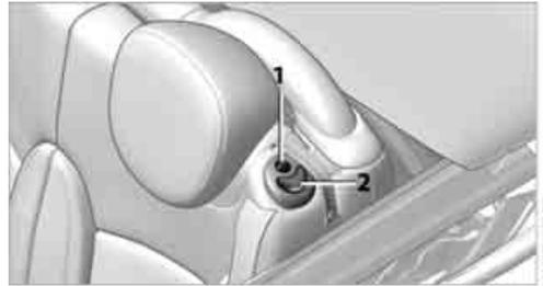
2. Press button 2 and fold down backrest together with the belt strap.
