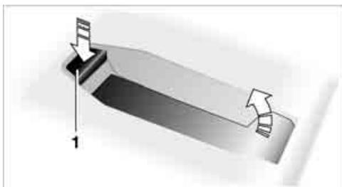
2. Insert the snap-in adapter at the front, arrow 1, and press downward, arrow 2, until it clicks into place.
