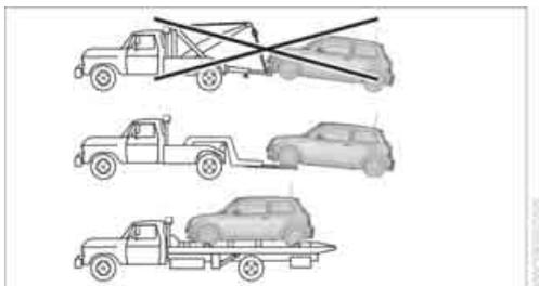
Have the MINI or MINI Convertible transported by a tow truck with a so-called lift sling or on a flatbed.
