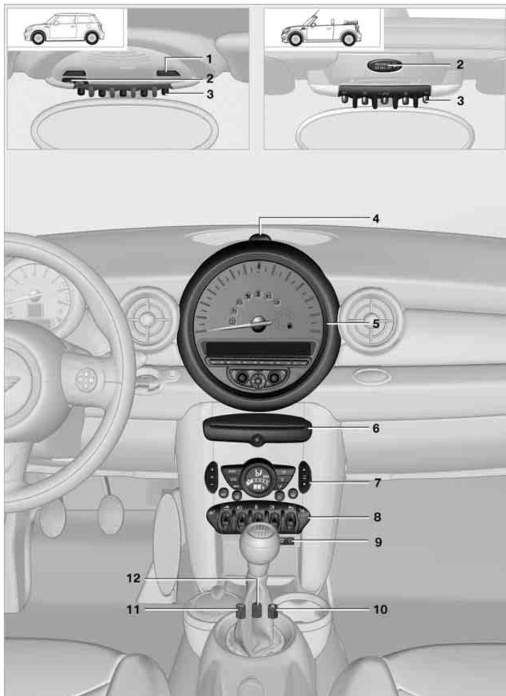
**1** MINI: microphone for voice processing system\* and for hands-free telephone\*
