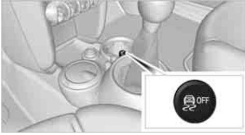
Press the button, the indicator lamp for DTC lights up in the display elements and TRACTION is displayed in the tachometer.
