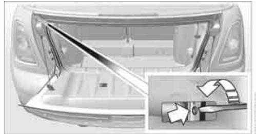
3. Use the screwdriver and turn the gold-colored screw, see arrow, one and a half turns in the direction of the arrow.
