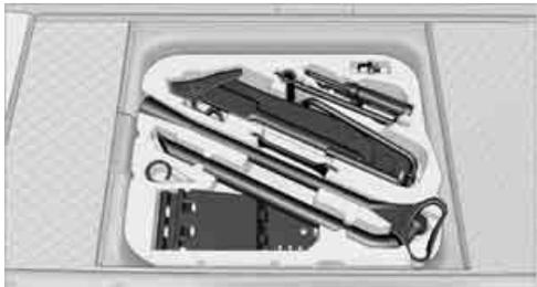
Your vehicle comes with an onboard vehicle tool kit that varies with the equipment version; it is stored underneath the flat load floor.
