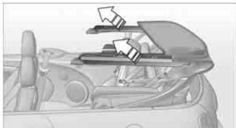
2. Lift out both sides at the same time, and swing the convertible top forward onto the cowl.
