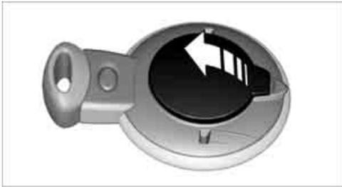
2. Insert the new battery with the plus side facing up.
