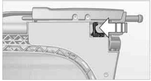
Push the release lever toward the center of the wind deflector and fold both halves together.
