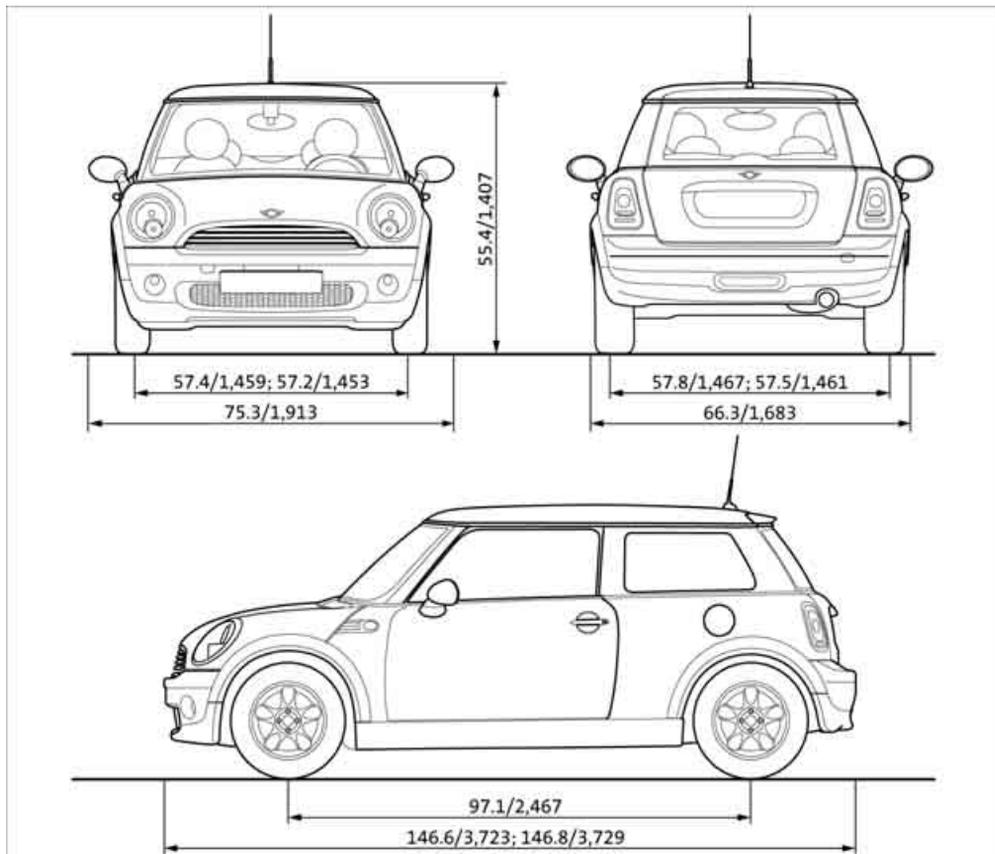
All dimensions in inches/mm. Minimum turning radius Ø: 35 ft 10 in/10.7 m.
