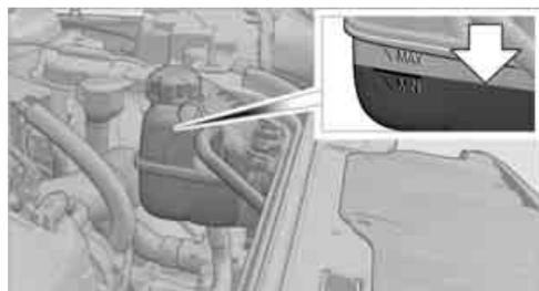
The coolant level is correct if it is between the Min and Max markings.
