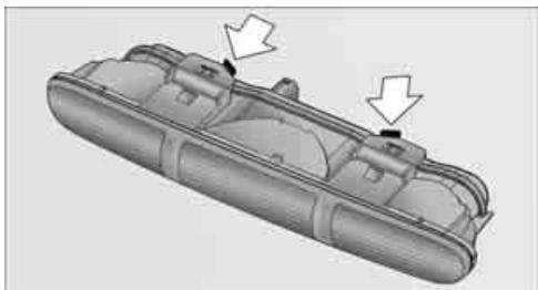
1. Squeeze clamping clips, arrows, and remove bulb holder.
