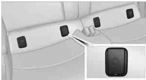
The anchor points for the lower LATCH anchors are located behind the labeled protective caps.
