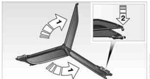
3. Press the locking device together until it engages, see arrow 2.
