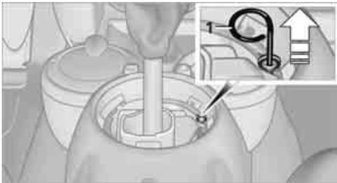
3. Insert extractor hook 1 from the onboard vehicle tool kit into the loop on the passenger's side.
