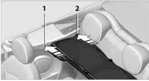
1. Push out retaining pin **2** on one side until it engages.
