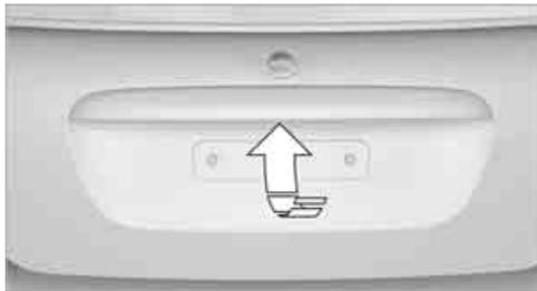
Press the button in the handle, arrow, or the
