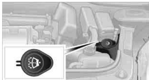
Fill with water and, if required, with a washer antifreeze, according to manufacturer's recommendations.
