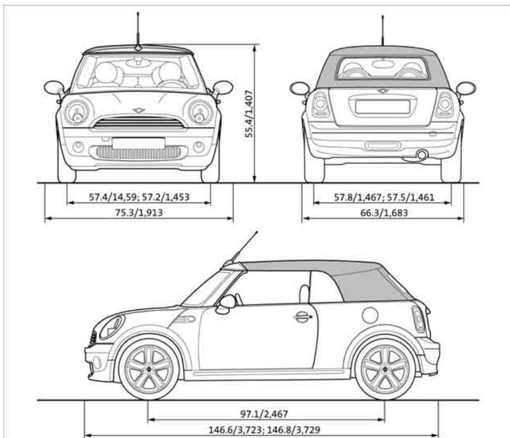
All dimensions in inches/mm. Minimum turning radius  $\varnothing$ : 35 ft 10 in/10.7 m.
