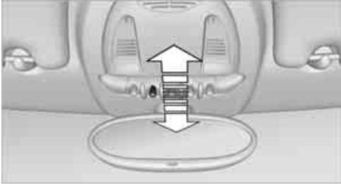
To switch the interior lamps on/off.
