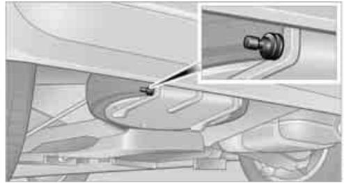
A valve extension for checking the inflation pressure is located behind the bumper.
