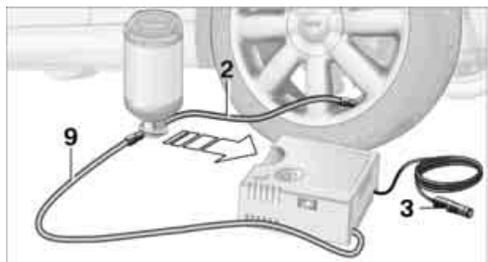
4. Unscrew the dust cap from the valve of the defective wheel and screw the filling hose **2** of the sealant bottle onto the valve.
