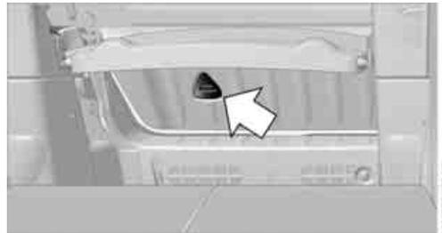
3. Pull the handle, see arrow. The liftgate is released.
