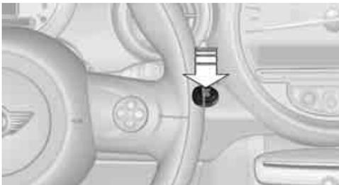
Press the Start/Stop button to switch radio readiness or the ignition on and off. Do not depress the brake or clutch while doing so.
