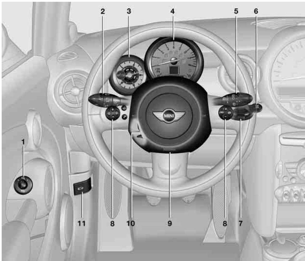
1 Adjusting the exterior mirrors, folding them in and out\* 39
