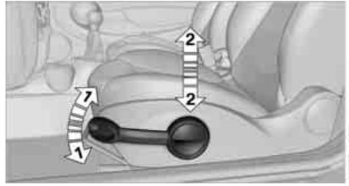
Pull up or push down the lever repeatedly, arrows 1, until the desired height is reached, arrows 2.
