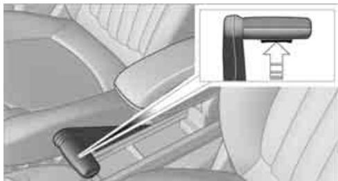
Pull upward slightly, press the button, arrow, and guide the lever down.
