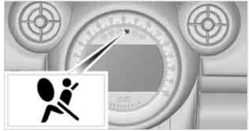
As of radio readiness, page 48, the warning lamp lights up briefly to indicate that the entire airbag system and the belt tensioners are operational.
