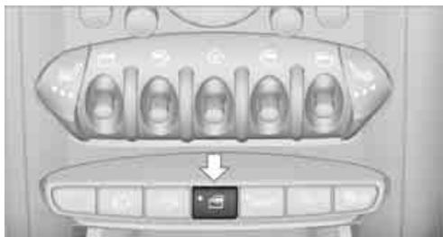
With the safety switch, you can prevent the rear windows from being opened or closed via the switches in the rear passenger area, by children, for example.
