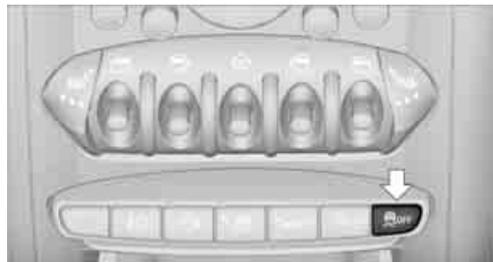
Press the button; the indicator lamp DSC OFF on the speedometer comes on and TRACTION is displayed on the tachometer. The Dynamic Stability Control DSC is deactivated; the Dynamic Traction Control DTC is activated.
