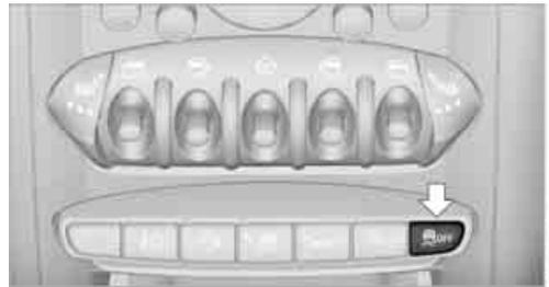
Press the button until the DSC OFF indicator lamp on the speedometer is on and DSC OFF is displayed on the tachometer. DSC is deactivated. Stabilizing and propulsion promoting actions are no longer executed.
