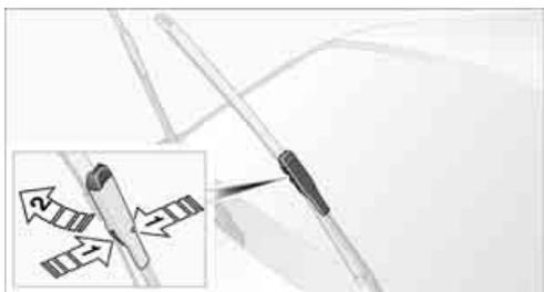
2. Press together the locking spring, arrows 1, and fold out the wiper blade, arrow 2.
