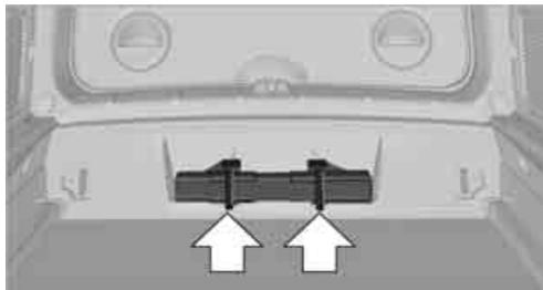
In the cargo area under the loading sill. To remove, open the two clasps.
