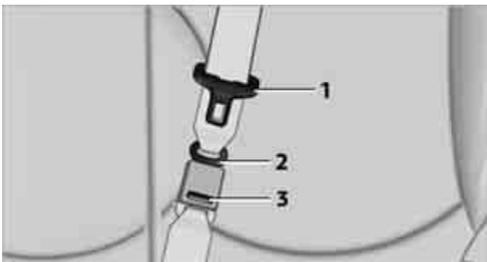
Insert safety belt with small belt latch 2 into the small belt buckle 3.
