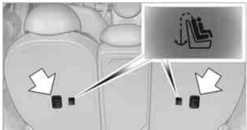
The child restraint anchor fittings for the two outer seats, see arrows, are located behind the back of the rear seats.
