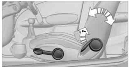
Pull lever, arrow 1, and apply weight to or remove weight from the backrest as needed.
