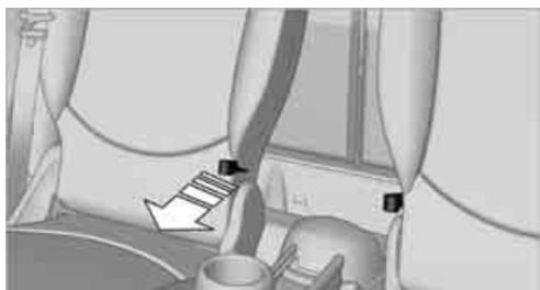
1. Hold on to the backrest near the top, for example on the headrest, and pull on the loop, arrow.
