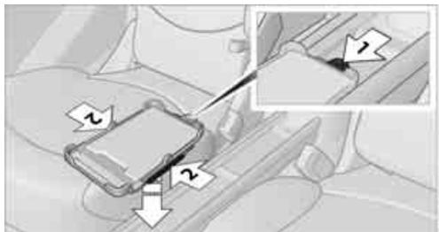
2. First install the smartphone on the Center Rail with the mounts **2**.
