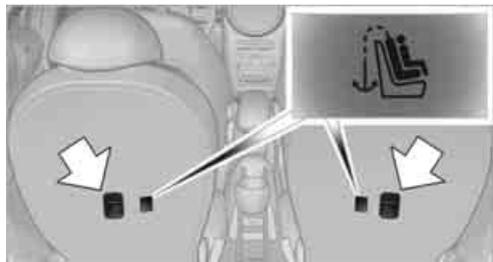
The child restraint anchor fittings, see arrows, are located behind the back of the rear seats.
