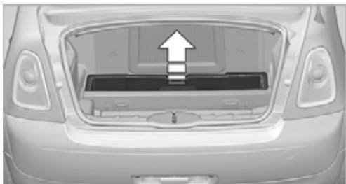
3. Using the Allen wrench from the tool kit, turn the gold-colored screw, see arrow, in the direction of the arrow by about four or five rotations all the way to the stop.
