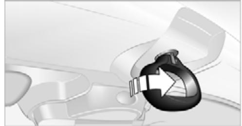
2. Using the handle, push unlocked convertible top upwards and open about six inches.
