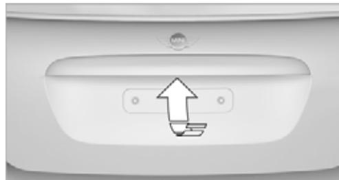
Press the button in the handle, arrow, or the
