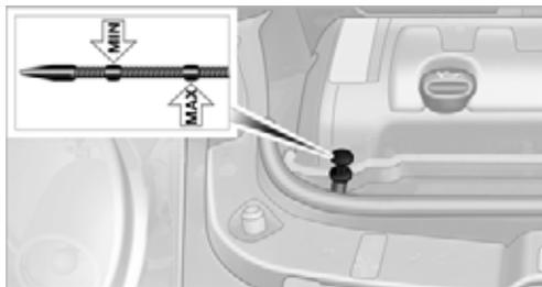
The oil quantity corresponding to the difference between the two marks on the dipstick is 1 US quart/1 liter.
