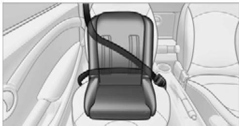
The safety belt for the passenger can be prevented from being pulled out in order to secure child restraint systems.
