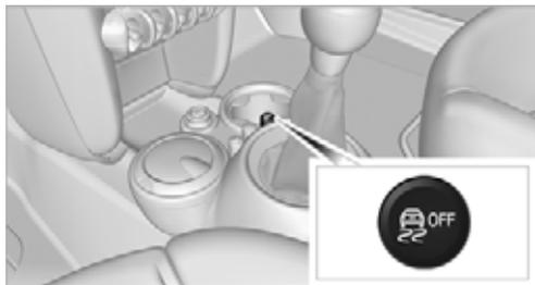
Press the button for at least 3 seconds; the indicator lamp DSC OFF on the speedometer comes on and DSC OFF is displayed on the tachometer. The Dynamic Traction Control DTC and Dynamic Stability Control DSC are both deactivated. There will be no more stabilizing interventions.
