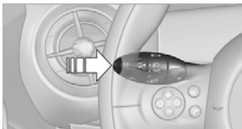
Press the button in the turn signal lever.
