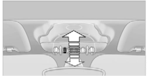
To switch the interior lamps on/off.
