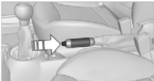
Pull slightly upward, press the button and lower the lever.
