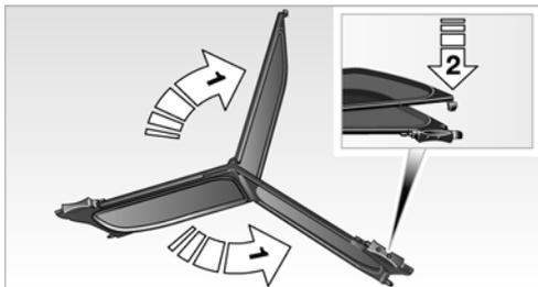
3. Press the locking device together until it engages, refer to arrow 2.
