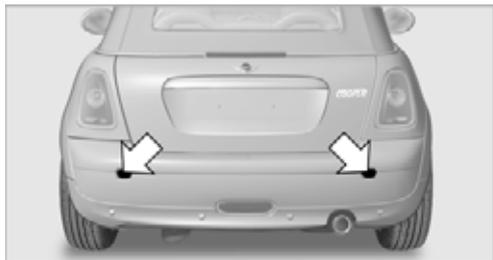
The mounting points are under the protective caps in the bumper.
