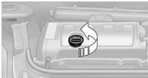
Do not add the maximum quantity of 1 US quart/1 liter of engine oil until the oil level has dropped to just above the lower mark on the dipstick, page 222.
