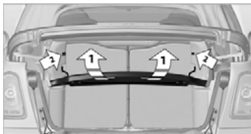
2. Pull luggage compartment roller cover rearward out of the lower brackets and pivot upward, refer to arrows 1,
