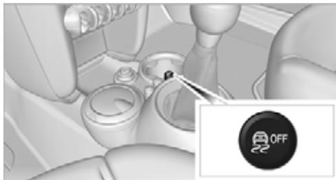
Press the button; the indicator lamp DSC OFF on the speedometer comes on and TRACTION is displayed on the tachometer. The Dynamic Stability Control DSC is deactivated; the Dynamic Traction Control DTC is activated.
