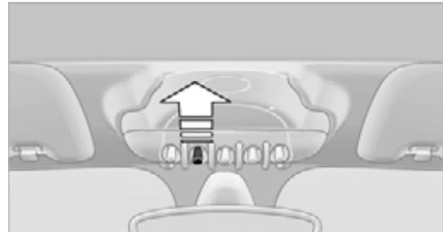
3. Push switch back to open the convertible top. The windows open during this procedure.
