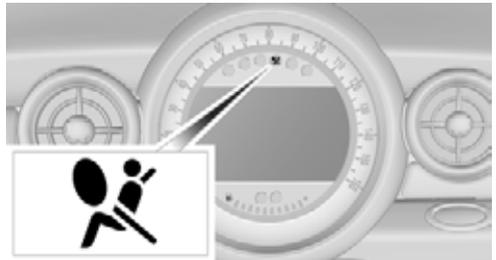
As of radio readiness, page 60, the warning lamp lights up briefly to indicate that the entire airbag system and the belt tensioners are operational.
