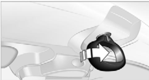
2. Using the handle, push the unlocked convertible top upwards and open about six inches.
