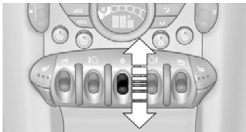
The switch locks or unlocks the doors and tailgate when the doors are closed, but the anti-theft system is not activated. The fuel filler flap remains unlocked.
