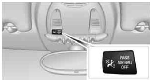
The indicator lamp for the front passenger airbags shows the functional status of the front passenger's front and side airbags in accordance with whether and how the front passenger seat is occupied. The indicator lamp shows whether
