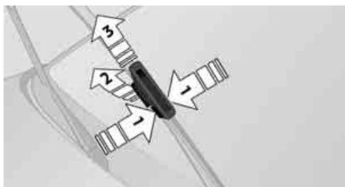
2. Compress the locking spring, arrows 1, and pivot it toward the wiper blade, arrow 2.
