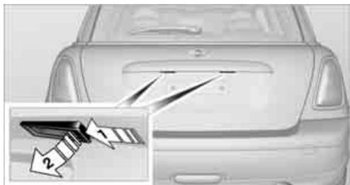
1. Using a screwdriver, push the lamp to the left in the tab of the lamp housing, arrow 1.
