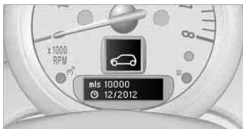
The remaining driving distance and the date of the next scheduled service are briefly displayed immediately after you start the engine or switch on the ignition.
