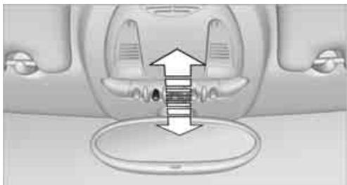
To switch the interior lamps on/off.
