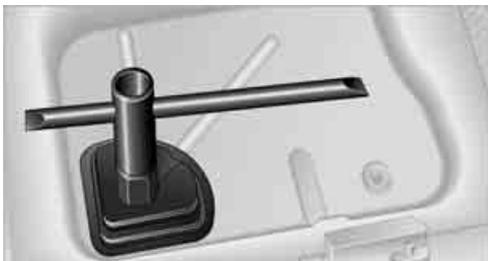
3. Screw the lifting handle from the toolkit onto the thread.
