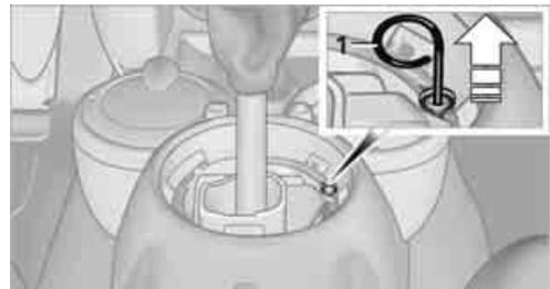
3. Insert extractor hook 1 from the toolkit into the loop on the passenger's side.
