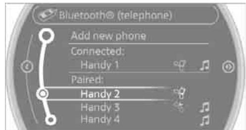
The assigned functions before the unpairing of the mobile phone are assigned to the mobile phone when it is reconnected. If a mobile phone is already connected, then these functions are deactivated if necessary.
