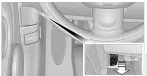
The primary components that make up the emissions can be checked by a device via the OBD socket.
