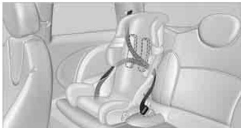
All rear safety belts and the safety belt for the front passenger can be prevented from being pulled out in order to secure child restraint systems.
