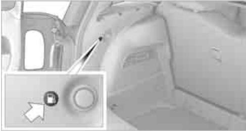
Pull on the green knob with the fuel pump symbol; the fuel filler flap opens.
