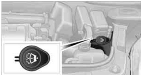
Fill with water and, if required, with a washer antifreeze, according to manufacturer's recommendations.
