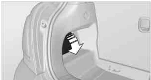
2. Unscrew the desired bulb counterclockwise, arrows 1. Another bulb is located behind the luggage compartment side wall, arrow 2.
