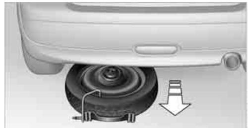
10. Position the space-saver spare tire with the valve facing upward.
