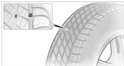
Wear indicators in the base of the tread groove are distributed around the tire's circumference; the letters TWI, for Tread Wear Indicator, on the tire's sidewalls identify tires that incorporate these wear indicators. When tire tread is worn down to the level of the wear indicators, the remaining tread depth is 0.063 in/1.6 mm.
