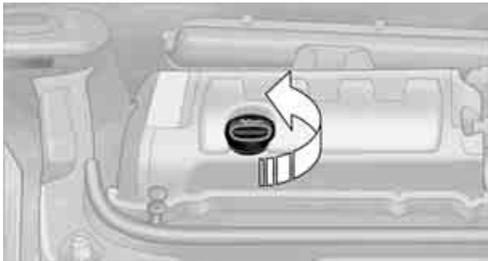
Do not add the maximum quantity of 1 US quart/1 liter of engine oil until the oil level has dropped to just above the lower mark on the dipstick, page 208.
