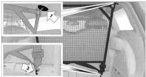
2. Insert each cargo net mounting pin all the way into its respective rear mount in the headliner, arrow 1, and push it forward.
