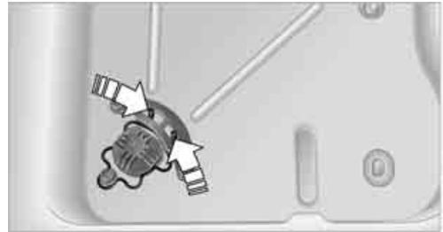
6. The space-saver spare tire is released and must be held by the lifting handle.
