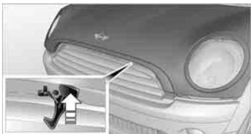
**!** To avoid damage, make sure that the wiper arms are against the windshield before you open the hood. ◀
