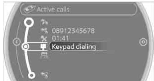
4. Enter the DTMF code via the onboard computer.
