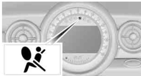
As of radio readiness, page 47, the warning lamp lights up briefly to indicate that the entire airbag system and the belt tensioners are operational.
