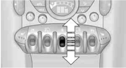
The switch locks or unlocks the doors and tail-gate/Split Rear Barn Doors when the doors are closed, but the anti-theft system is not activated. The fuel filler flap remains unlocked.
