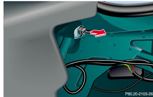
Remove the battery cover (see page 346) and the trim inside the trunk on the right-hand side. Pull the release knob (arrow) and open the fuel filler flap.
