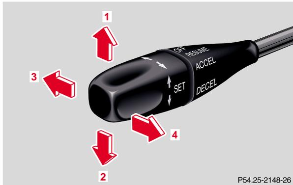
The cruise control allows you to drive in a more relaxed manner, for example over long distances, as it automatically maintains the set speed by actively regulating the throttle setting.
