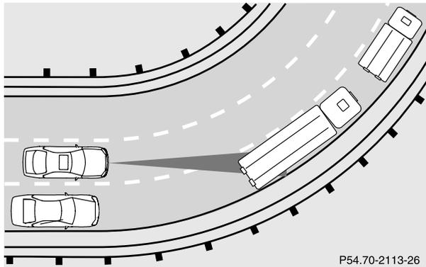
Traveling through turns or bends in the roadway may result in Distronic detecting a moving vehicle traveling in front but not in your lane of travel, causing your vehicle to brake late or unexpectedly. You must be prepared to intercede with accelerator or brake application as necessary.
