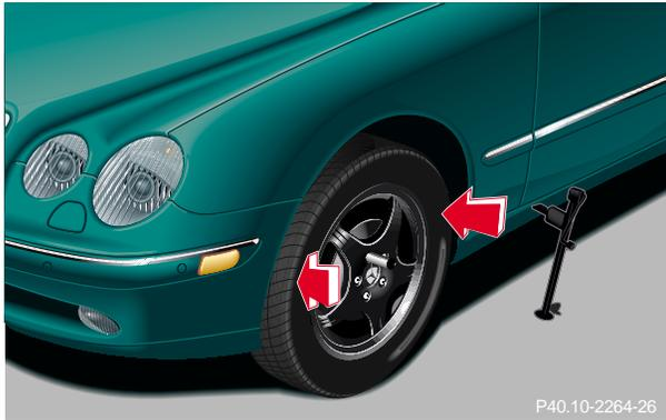
10. Clean contact surfaces of wheel and wheel hub. Install spare wheel on wheel hub. Insert wheel bolts and tighten them slightly.
