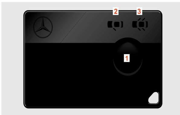
To choose between the selective or global opening mode press and hold button (1) until the indicator lamp at the requested symbol (2) or (3) comes on.
