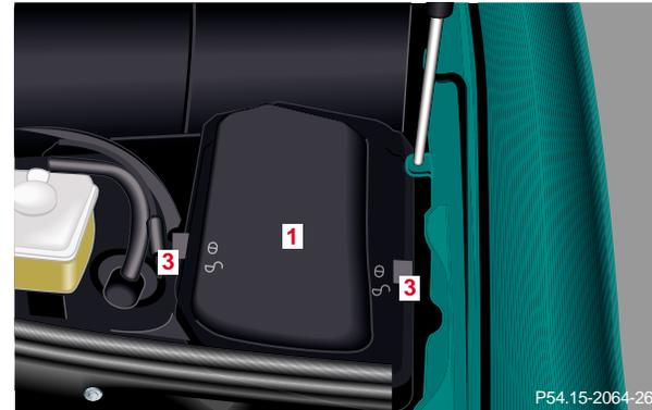
1 Fuse box in engine compartment, left-hand side
