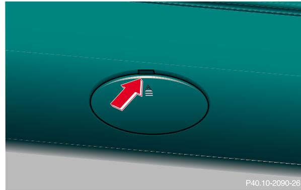
5. Remove the protective cover from the jack support tube opening by inserting the screwdriver (supplied in the tool kit) in the opening and prying it out.
