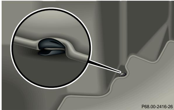
Inside the trunk are six cargo tie-down hooks. Secure cargo by applying even load on the hooks using a cargo net.
