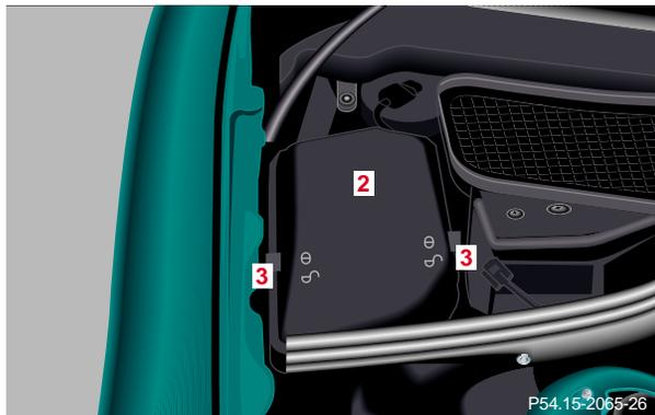
2 Fuse box in engine compartment, right-hand side
