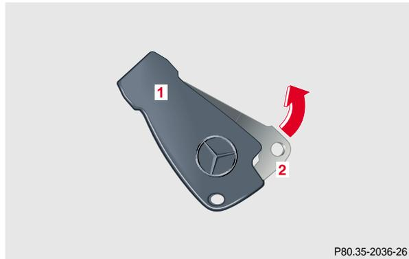
The electronic reserve key is without remote control functions, plus removable mechanical key.
