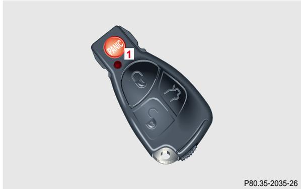
To activate press and hold button (1) for at least one second. An audible alarm and blinking exterior lamps will operate for approximately 2<sup>1</sup>/<sub>2</sub> minutes.
