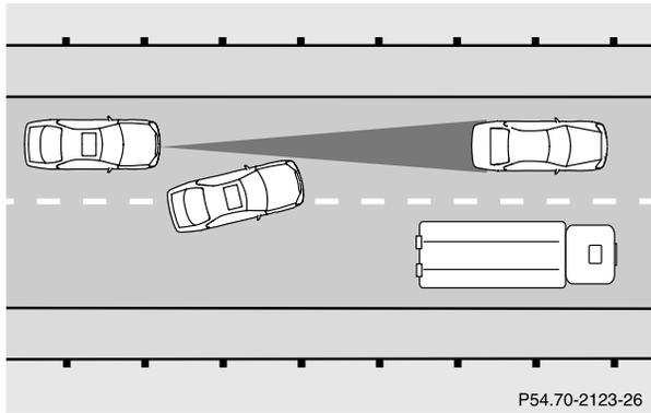
A vehicle changing lanes at close range is only recognized when entering the area scanned by DISTRONIC. You must apply the service brakes to gain sufficient distance to the vehicle ahead.
