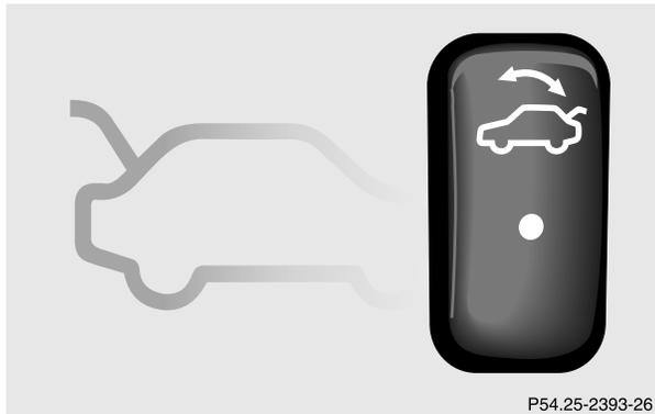
The switch is located on the driver's door.
