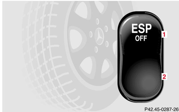
ESP control switch located on center console.
