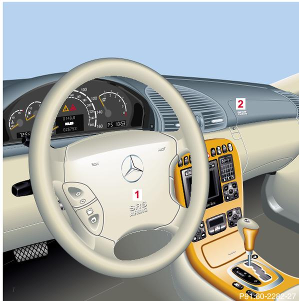
**1** Driver airbag**2** Front passenger airbag
