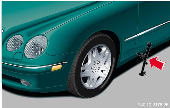
6. Insert jack arm fully into the tube hole up to the stop. Place jack on firm ground. Position the jack so that it is always vertical (plumb-line) as seen from the side (see arrow), even if the vehicle is parked on an incline.
