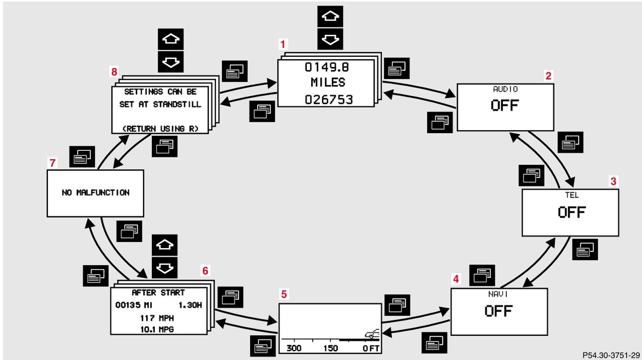
Depending on your vehicle's equipment, you may use the buttons on the multifunction steering wheel to call up, control and set the following systems in the multifunction display:
