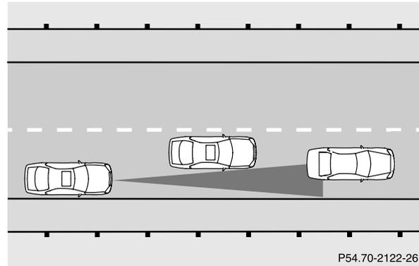
The Distronic system's detection zone is relatively narrow at the start and becomes broader as it senses further from the vehicle. Thus, Distronic may not recognize another vehicle coming into your path close to the front of your vehicle. You must be prepared to intercede with braking or steering as necessary. A vehicle not traveling directly in front of you could cause detection problems, the actual distance to that vehicle really being much shorter.
