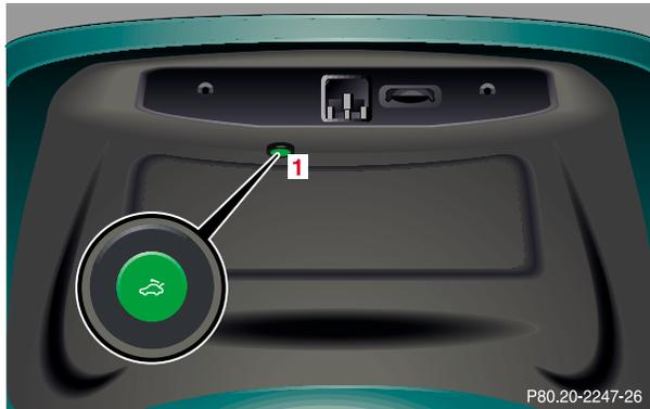
The emergency release button (1) is located in the trunk lid.
