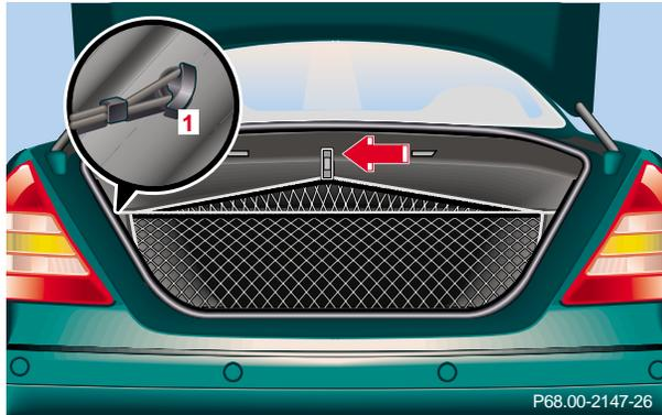
There are hooks (1) on the left and right inside the trunk from which the parcel net is suspended.
