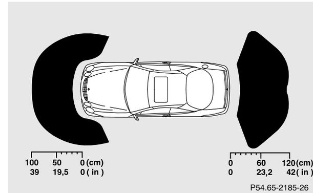
The first yellow segment lights up at these distances. Additional segments light up as the vehicle comes closer to the obstacle.
