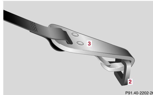
To secure a tether strap to the anchorage, securely fasten the hook (3), which is part of the tether strap, to the anchorage ring (2). For safety, please make sure that the hook has attached to the ring beyond the safety catch, as illustrated.
