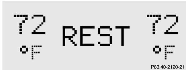
With the engine switched off, it is possible to continue to heat or ventilate the interior for a short while. Air volume and distribution are controlled automatically.
