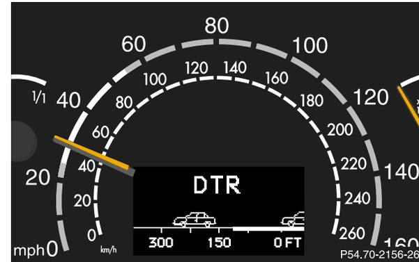
If a vehicle is detected ahead, those segments in the speedometer dial light up that indicate the speed range from the speed of the vehicle in front up to the Distronic stored speed.
