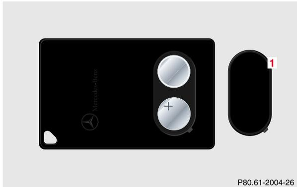
Pry open cover (1) (e.g. by using a narrow blade screw driver) and remove batteries.
