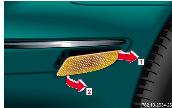
Carefully slide lamp towards rear (arrow 1), and remove front end first (arrow 2).
