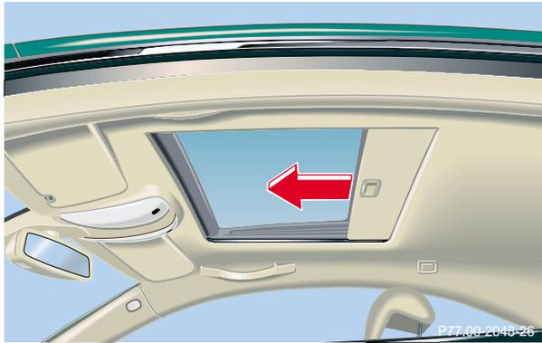
With the roof closed or tilted open, a screen can be slid into the roof opening to guard against sun rays. When sliding the roof open, the screen will also retract.
