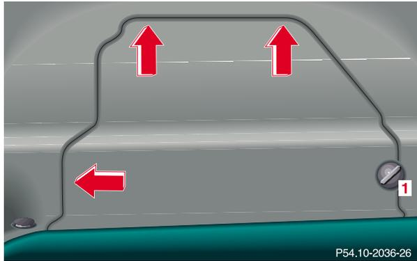
The maintenance-free battery is located in the trunk under the right-hand wheel well cover panel.
