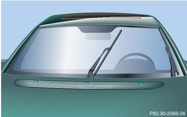
To prevent damage to the hood or the wipers, the wiper arms should only be folded forward while in the position shown above.
