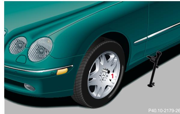
8. Unscrew upper-most wheel bolt and install alignment bolt (1) supplied in the tool kit. Remove the remaining bolts. Keep bolt threads protected from dirt and sand.
