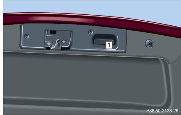
Lower trunk lid using handle (1) and close it with hands placed flat on trunk lid. Please remember to keep your fingers out of the space between the lid and the vehicle.
