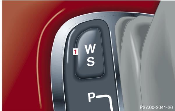
The transmission is provided with a selector switch (1) for Standard “S” and Winter/Wet (snow and ice) “W” program modes.
