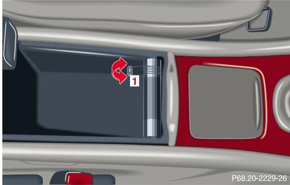
The front center console compartment has its own air outlet.
