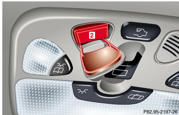
Press the emergency call switch (2) briefly (for longer than 2 seconds). The indicator lamp in the emergency call switch (2) will flash until the emergency call is concluded. Wait for a voice connection to the Response Center.
