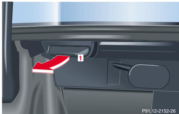
1. Pull handle (1) located in trunk to unlock backrest.
