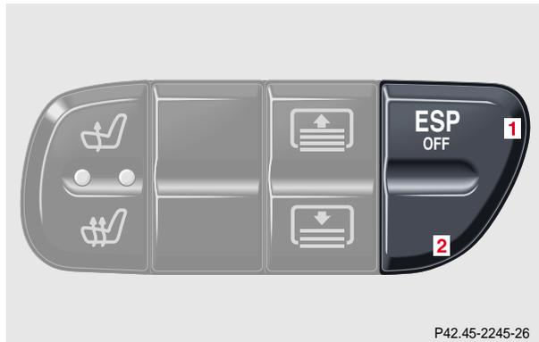
ESP control switch located on center console.
