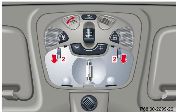
Slide both locking tabs (2) in direction of arrow, lower rear of cover and remove.
