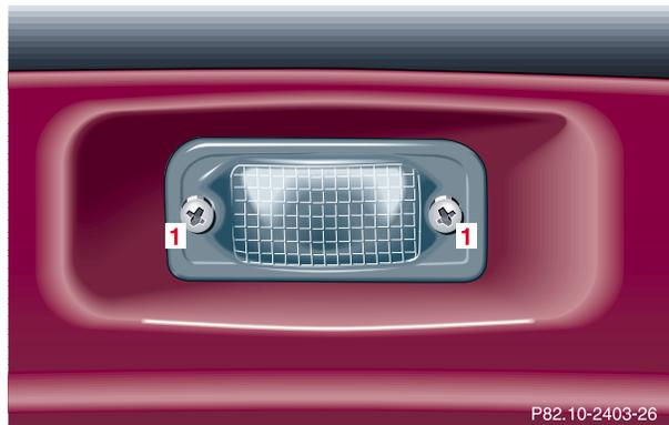
Loosen both securing screws (1), remove lamp and replace tubular lamp (C 5 W/4 cp).
