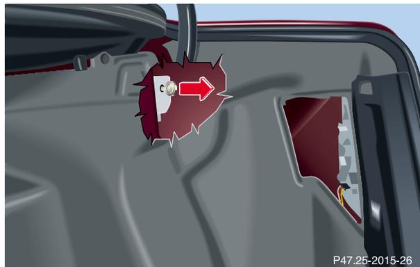
Open the trunk lid and fold right-side taillamp trim aside. Reach inside and pull the release knob (arrow). Open the fuel filler flap.
