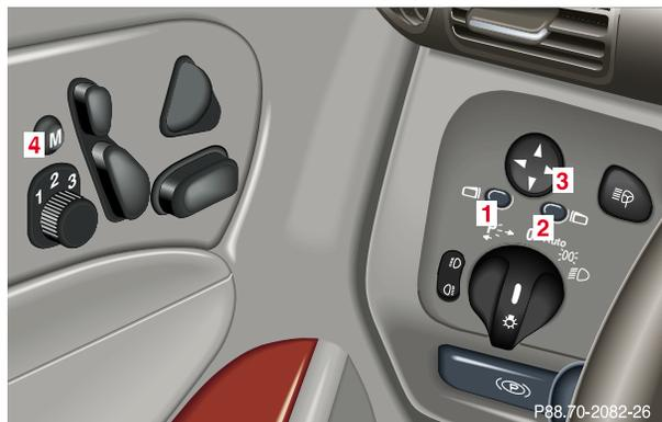
The buttons are located above the exterior lamp switch. The memory button (4) is located on the driver's door.
