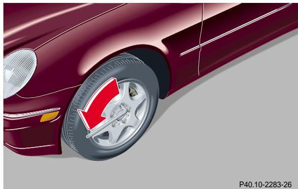
5. Remove the two-piece wheel wrench from the vehicle tool kit and assemble (see page 305).
