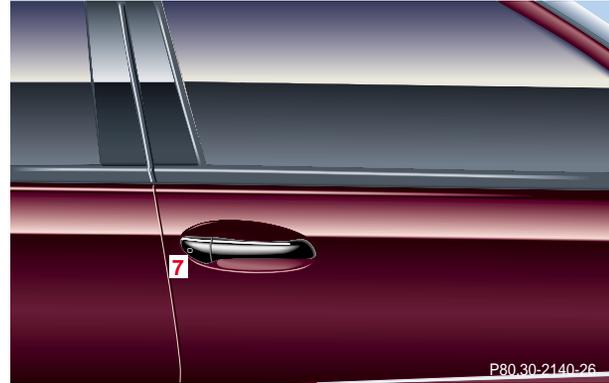
7 Infrared receiver in front passenger door handle
