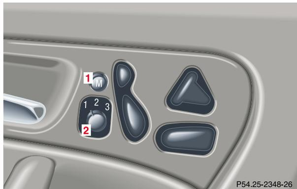
Together with the driver's seat position you can store the positions for steering wheel and exterior rear view mirrors.
