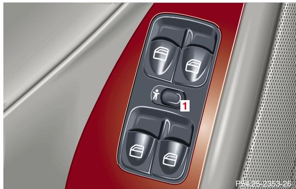
The switch (1) is located on the driver's door.
