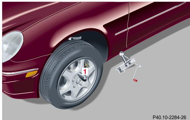
9. Unscrew upper-most wheel bolt and install alignment bolt (1) supplied in the tool kit. Remove the remaining bolts. Keep bolt threads protected from dirt and sand.
