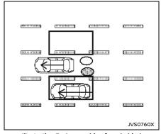
Illustration 3 - Approaching from behind Illustration 3: If the I-BSI system is on and your vehicle approaches a lane marker while another vehicle is in the detection zone, the system chimes (three times) and the side indicator light and I-BSI indicator flash. The I-BSI system activates to help return the vehicle back to the center of the driving lane.
