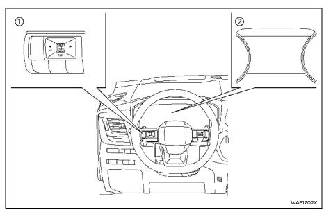
Steering-wheel-mounted controls (left side)
