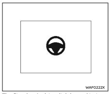
The Steering Assist switch is used to temporarily turn on and off the Steering Assist system.
