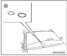
Be sure not to put anything on top of the photo sensor (a) located on the top of the instrument panel. The photo sensor controls the Intelligent Auto Headlight; if it is covered, the photo sensor reacts as if it is dark and the headlights will illuminate.
