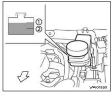
Check the fluid level in the reservoir. If the fluid is below the MIN line @ or the brake warning light comes on, add Genuine NISSAN Super Heavy Duty Brake Fluid or equivalent **DOT3** fluid up to the MAX line n and it is recommended you have your vehicle checked by a NISSAN dealer as soon as possible. If fluid must be added frequently, the system should be checked. It is recommended you visit a NISSAN dealer for this service.
