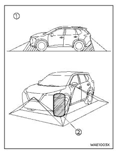
There are some areas where the system will not show objects and the system does not warn of moving objects. When in the front or the rear view display, an object below the bumper or on the ground may not be viewed fig. When in the bird's-eye view, a tall object near the seam a of the camera viewing areas will not appear in the monitor.
