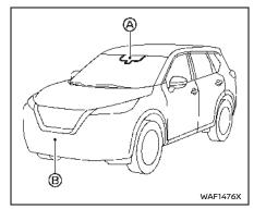
The AEB with Pedestrian Detection system uses a radar sensor @ located on the front of the vehicle to measure the distance to the vehicle ahead in the same lane.
