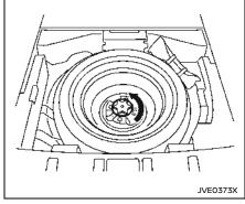
Remove the spare tire by removing the clamp holding it.
