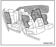
FRONT, FRONT CENTRAL\*, REAR **OUTBOARD SEAT-MOUNTED SIDE-**IMPACT SUPPLEMENTAL AIR BAG AND ROOF-MOUNTED CURTAIN SIDE-IMPACT AND ROLLOVER SUPPLEMENTAL AIR BAG SYSTEMS
