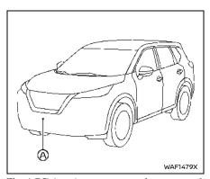
The I-FCW system uses a radar sensor (A) located on the front of the vehicle to measure the distance to a second vehicle ahead in the same lane.
