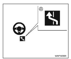
When ProPILOT Assist is active and the status indicator (A) is illuminated in blue, Lane Change Assist helps the driver make a lane change when the turn signal is activated. The driver must place their hands on the steering wheel prior to the lane change maneuver and ensure safety throughout the lane change.
