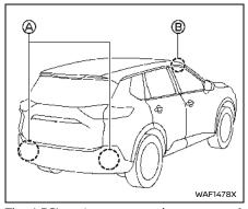
The I-BSI system uses radar sensors @ installed near the rear bumper to detect other vehicles in an adjacent lane. In addition to the radar sensors, the I-BSI system uses a camera (c) installed behind the windshield to monitor the lane markers of your traveling lane.
