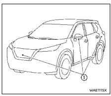
To display the multiple views, the Intelligent Around View® Monitor system uses cameras n located on the front grille, on the vehicle's outside mirrors and one just above the vehicle's rear license plate.
