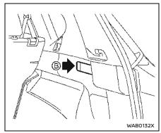
Pull the lever (c) (if so equipped) located on the side of the luggage area.
