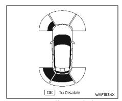
When the shift lever is in the R (Reverse) position and the Parking Assist screen is displayed in the vehicle information display, the RAB system can be disabled temporarily by pushing the scroll dial on the steering wheel.
