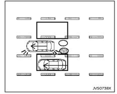
Illustration 2 - Approaching from behind Illustration 2: If the driver activates the turn signal then the system chimes a sound (twice) and the side indicator light and I-BSI indicator flash.
