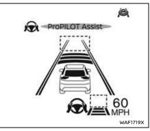
System set display — no vehicle detected ahead (for ProPILOT Assist, ProPILOT Assist 1.1)\*
