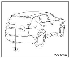
To display the rear view, the RearView Monitor system uses a camera n located just above the vehicle's license plate.
