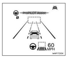
System set display - no vehicle detected ahead (for ProPILOT Assist 2.1)
