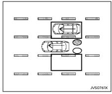
Illustration 6 - Overtaking another vehicle Illustration 6: If the I-BSI system is on and your vehicle approaches a lane marker while another vehicle is in the detection zone, the system chimes (three times) and the side indicator light and I-BSI indicator flash. The I-BSI system activates to help return the vehicle back to the center of the driving lane.
