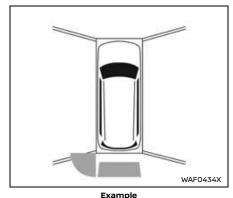
The sonar indicator also appears on the camera view of the center display.
