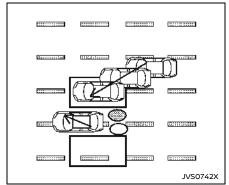
Illustration 10 - Entering from the side Illustration 10: The I-BSI system will not operate if your vehicle is on a lane marker when another vehicle enters the detection zone. In this case only the BSW system operates.
