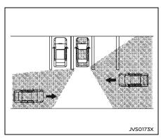
The RCTA system uses radar sensors (a) installed on both sides near the rear bumper to detect an approaching vehicle. The radar sensors can detect an approaching vehicle from up to approximately 66 ft (20 m) away.
