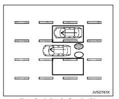
Illustration 9 - Entering from the side Illustration 9: If the I-BSI system is on and your vehicle approaches the lane marker while another vehicle is in the detection zone, the system chimes (three times) and the side indicator light and I-BSI indicator flash. The I-BSI system activates to help return the vehicle back to the center of the driving lane.
