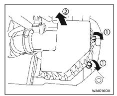
To remove the filter, release the lock pins n and pull the unit upward o.
