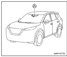
The LDW system will operate when the vehicle is driven at speeds of approximately 37 MPH (60 km/h) and above, and the lane markings are clearly visible on the road.
