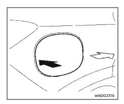
OPENING THE FUEL-FILLER DOOR To open the fuel-filler door, push the middle left side of the door.
