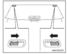
Before moving the rear (outer) luggage board, release the lock on the both sides of the board as shown.
