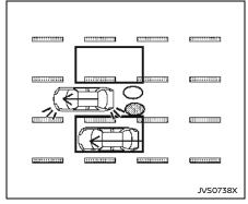
Illustration 2 - Approaching from behind Illustration 2: If the driver activates the turn signal while another vehicle is in the detection zone, then the system chimes (twice) and the side indicator light and BSW indicator flash.
