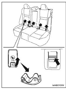
LATCH lower anchor cover removal
