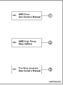
If the "AWD Error" warning (1) appears. there may be a malfunction in the Intelligent 4x4 system. Reduce vehicle speed and have your vehicle checked by a NISSAN dealer as soon as possible.
