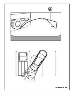
Backing up near a projecting object The predictive course lines (A) do not touch the object in the display. However, the vehicle may hit the object if it projects over the actual backing up course.
