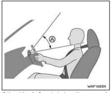
If the driver's face is below the camera's detection range A the driver monitor may not work properly. Adjust your face position so that the camera can detect vour entire face, by lowering the steering column or raise the seat position, for example.
