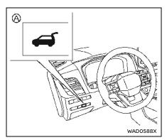
Power liftgate switch - Instrument panel
