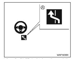
When ProPILOT Assist is active and the status indicator (a) is illuminated in blue, Passing Assist will help the driver to overtake a slower vehicle by:
