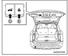
Power liftgate close and lock switches — Liftgate
