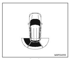
Example When the rear of the vehicle moves closer to an obstacle, the sonar indicator appears in the vehicle information display.
