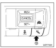
Assist in lane change with Lane Change Assist after the driver's acceptance by the Lane Change Assist switch © on the steering wheel.
