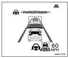
System set display — a vehicle detected ahead (for ProPILOT Assist, ProPILOT Assist 1.1)\*
