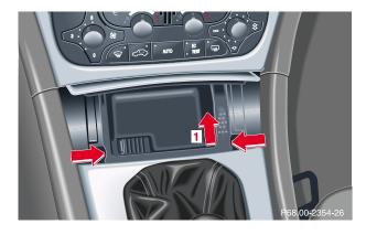
Slide ashtray insert in direction of arrow (1) until the insert disengages. Grip ashtray insert at indents (left and right arrows) and remove from ashtray frame.
