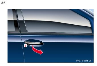
7 Infrared receiver in passenger door handle
