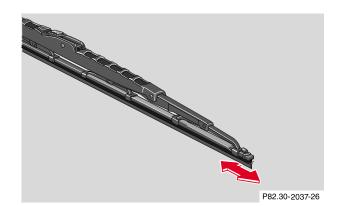
Place wiper blade on firm support. Press down both tabs and slide (direction of arrow) the wiper blade insert out of the retainer claws.
