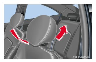
Adjust the head restraint angle by hand. Push or pull the head restraint in direction of arrow.
