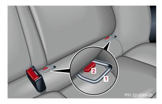
This vehicle is provided with two "LATCH" (LOWER Anchors and Tethers for CHildren) type mounts (at each of the rear seats) for the installation of a "LATCH" child seat having the matching mounting fittings. The mounts can be folded back between the seat cushion and the backrest.
