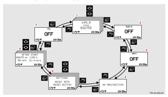
Depending on your vehicle's equipment, you may use the buttons on the multifunction steering wheel to call up, control and set the following systems in the multifunction display:
