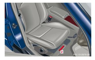
Vehicle Identification Number (VIN) (below right front passenger seat)
