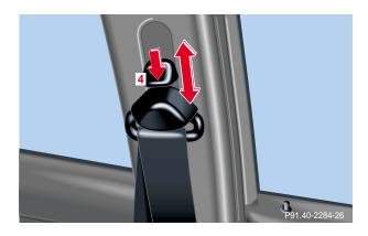
4 Button for belt outlet height adjustment
