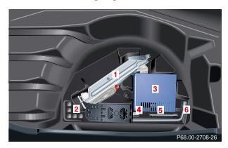
Vehicle tools and air pump are located in the wheel well below the trunk floor.
