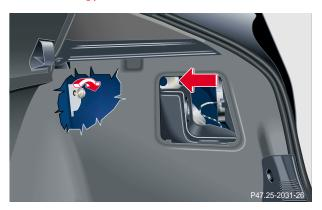
Open the trunk lid and fold right-side taillamp trim aside. Reach inside and turn the release knob (arrow) clockwise. Open the fuel filler flap.
