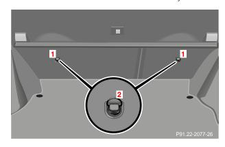
The anchorage rings (1) are located on the back side of rear backrests.
