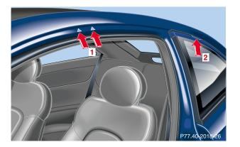
Mount roof racks only between the fastening points (1) (see arrows) and in the recess of the rubber strip (2).
