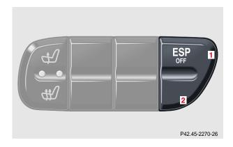
ESP control switch located on center console.
