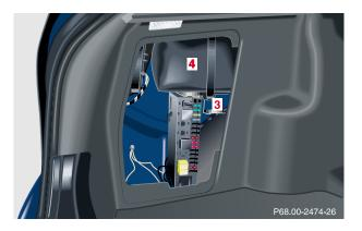
Loosen securing strap (3) and remove first aid kit (4).
