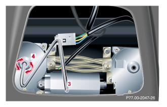
Obtain crank (3) (supplied with vehicle) and insert through left hand side motor hole (4).
