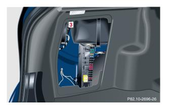
Press together the latches (3) and remove bulb carrier.
