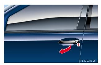
6 Infrared receiver in driver's door handle
