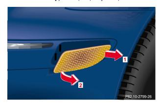
Carefully slide lamp towards rear (arrow 1), and remove front end first (arrow 2).
