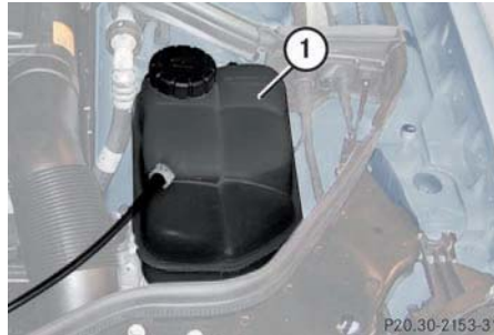
1 Coolant expansion tank
