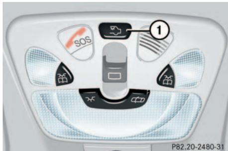
1 Switch for cargo compartment lamps
