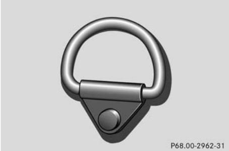
The cargo area is provided with four tie-down anchors.
