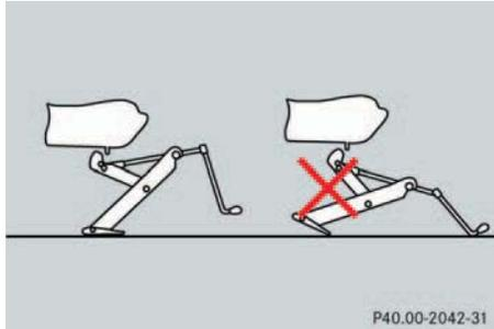
Make sure the foot of the jack is directly under the take-up bracket so that it is always vertical (plumb-line) as seen from the side, even if the vehicle is parked on an incline
