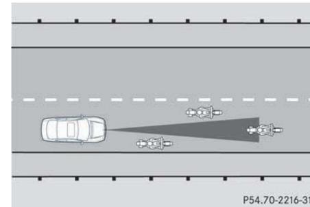
Because of its narrow profile, the vehicle traveling near the edge of the roadway has not yet been detected by Distronic. There will be insufficient distance to the vehicle ahead.
