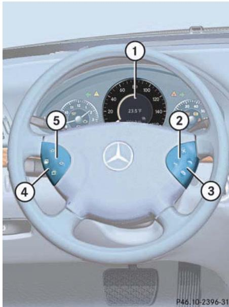
Pressing any of the buttons on the multifunction steering wheel will alter what is shown in the multifunction display.
