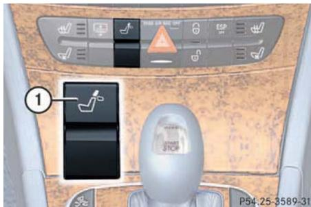
① Head restraint release switch
