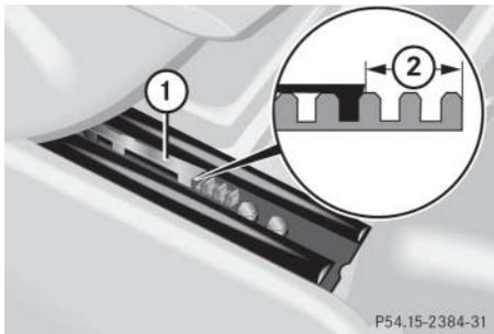
Front end stop on the right seat rail, left seat rail laterally reversed
