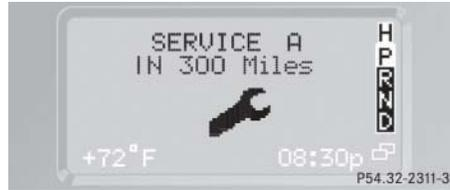
The type of service due is indicated in the speedometer display field:
