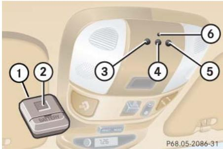
**Remote control integrated into the overhead control panel**
