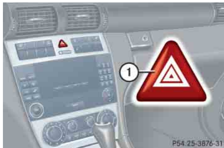
① Hazard warning flasher switch
