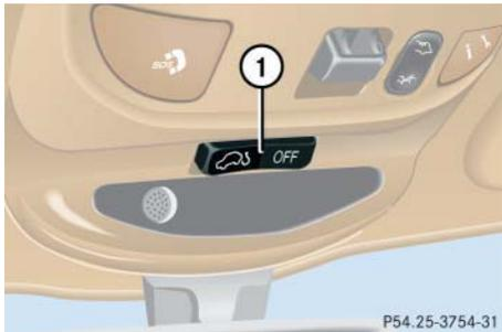
① Switching off tow-away alarm and glass breakage sensor
