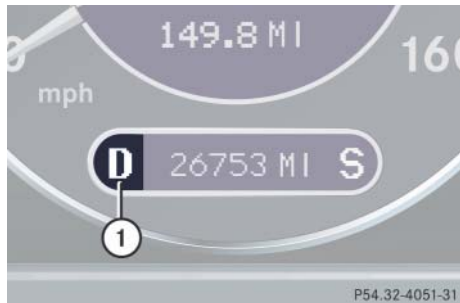
① Current gear selector lever position
